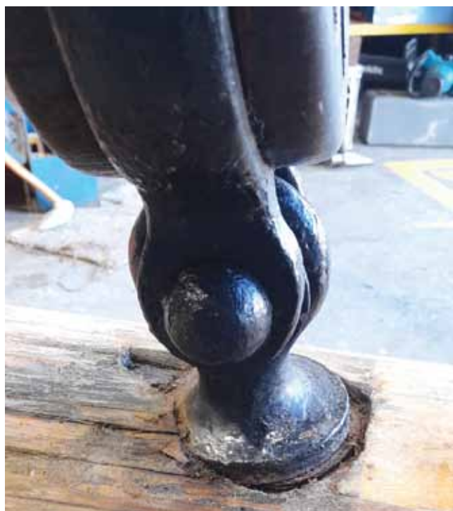
FIGURE 1 – Inner forestay deadeye with signs of rot.
