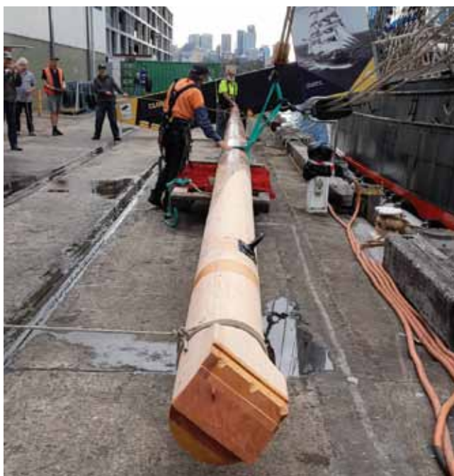
FIGURE 12 – Jib boom ready for hauling into place.
