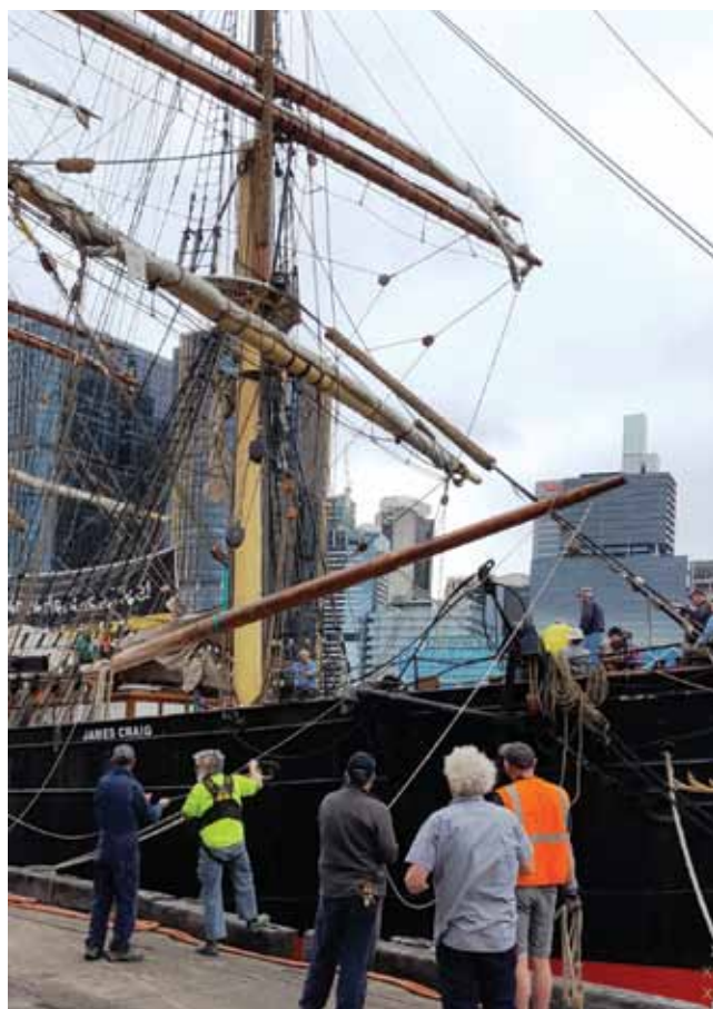
FIGURE 13 – Jib boom on its way to the focsle.
