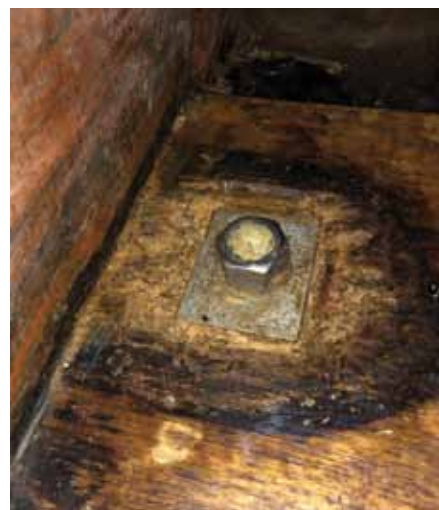
This was how the keel bolts looked before removal, the discolouration was only on the surface.
