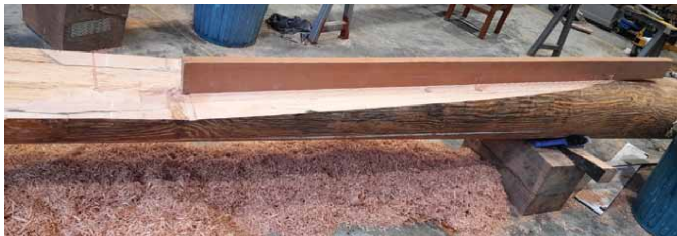
FIGURE 7 – Tapered scarf section of the jib boom.
