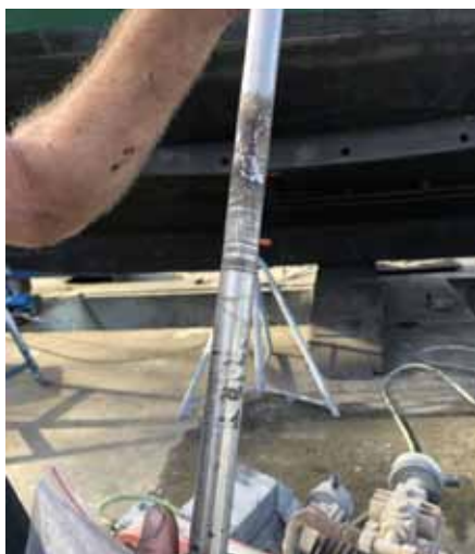
THE KEEL BOLT'S in very good condition.
