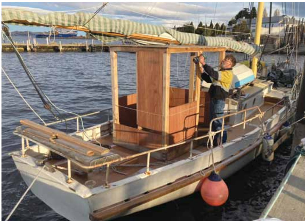
PETER INSTALLING the new wheelhouse. Image Paul Chapman
