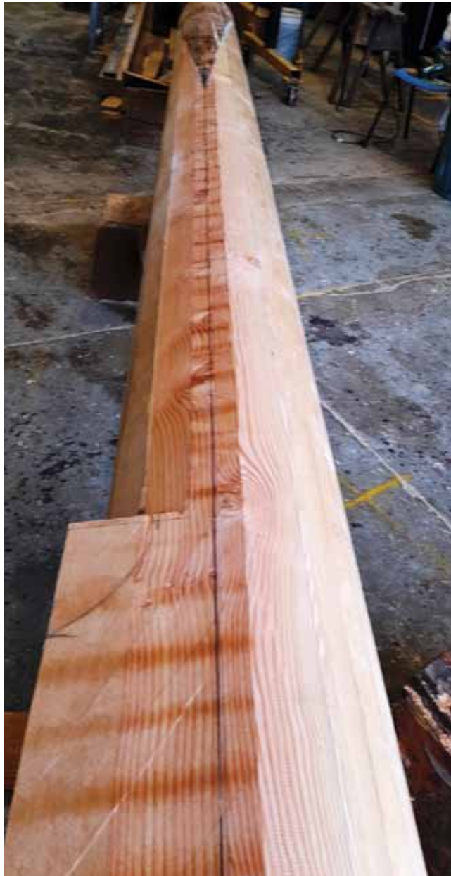
FIGURE 9 – The jib boom shaped to 16 sides.
