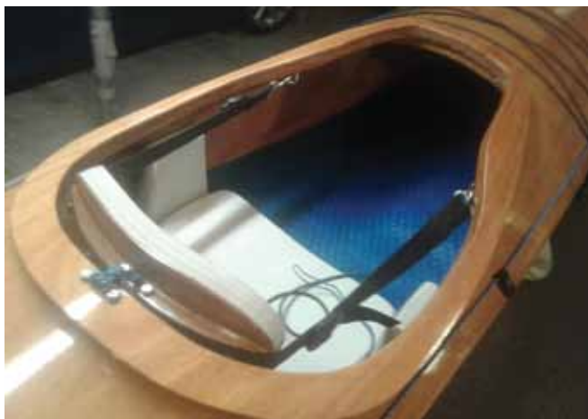
Cockpit 50mm wider than plans.
