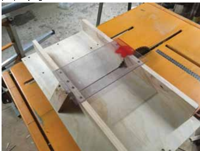
SLED. Will do an article on manufacture of this. Note red paint 'safety warning'.
