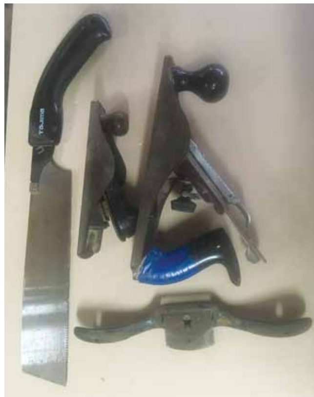
PULL SAW AND PLANES. A pull saw is more accurate and faster than a tenon saw. Block plane works well pulled rather than pushed. On ply holding the plane at a 45° angle across the edge works best.
