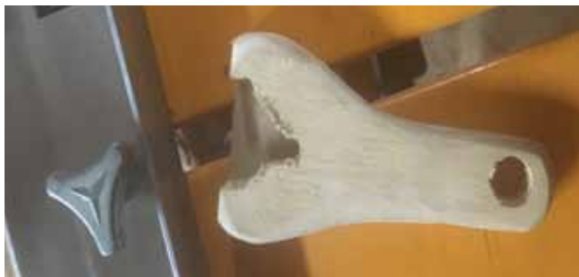
WOODEN SPANNER. This is specific to Triton MkIII. The bolts to hold the fence in place are hard to tighten sufficiently. Hence the wooden spanner. (Make your own special tools as needed.)
