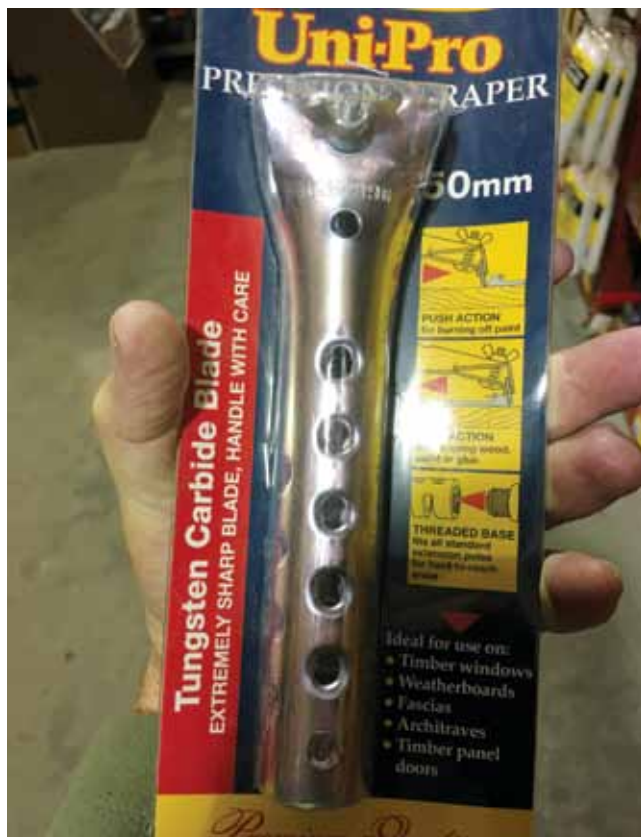
SCRAPER. Remove corners so they can't dig in.
