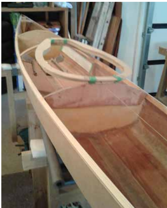
Frame and cockpit rim before deck fitted.
