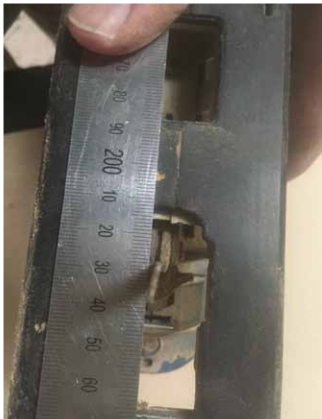
JIGSAW BLADE. Cheap saw – notice the blade is not parallel to the side of the saw. Nice looking saw but ...
