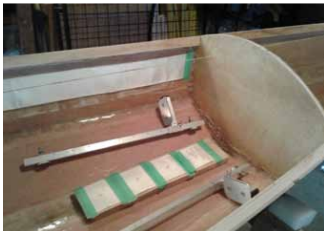
Adjustable footrests epoxied to inside hull, no holes!
