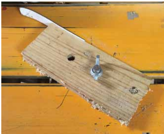
FINGER SPRING. Cut off 1/2" coach bolt fits perfectly in Trojan slot. Set up with spring a short distance before saw blade. Nut only needs to be finger tight.
