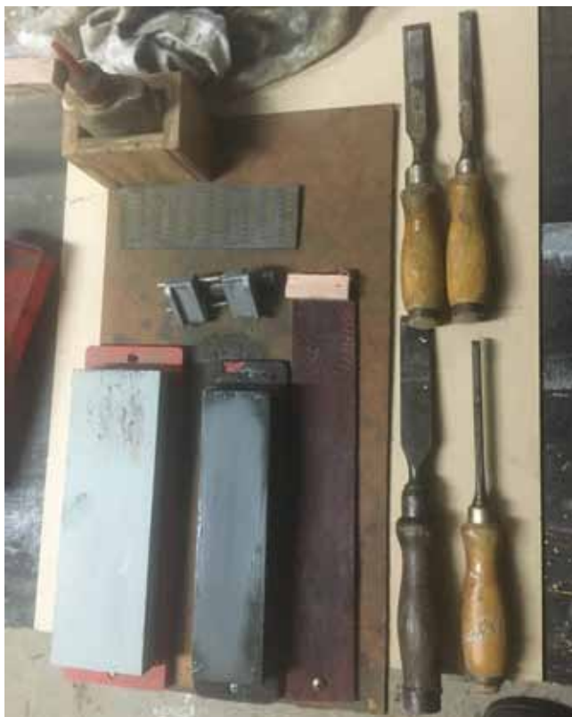
CHISELS AND SHARPENING JIG. Sharpen with a 25° main bevel and a short (1-2mm) working bevel of 30°. Leather strop to remove feather edge. Wider stone kept for plane blades as frequent chisel sharpening leaves stone face concave.
