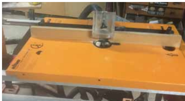
ROUTER TABLE. Safer than hand held and some of the sawdust can be collected.
