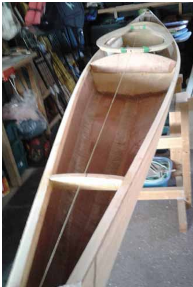
String line – an essential tool for keeping things straight.
