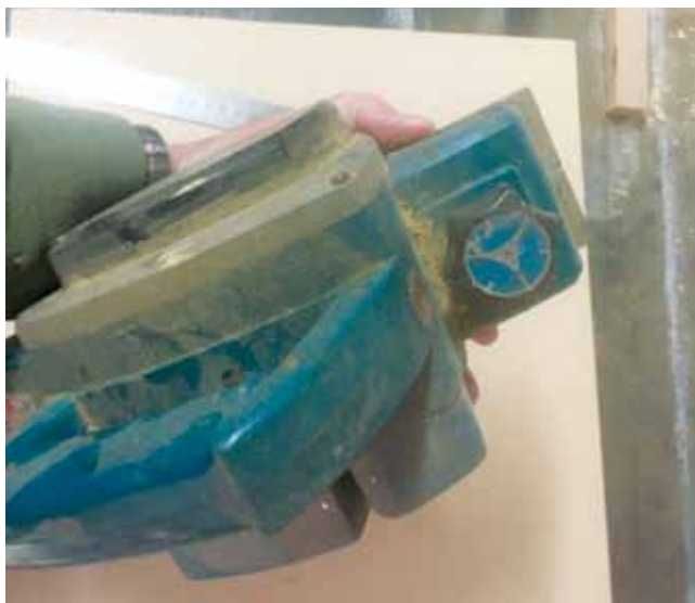
POWER PLANE. DON'T grab plane like this before the blade has completely stopped!
