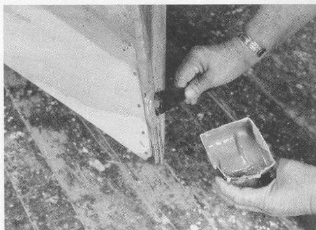
Fill out the stem area with plenty of putty.
