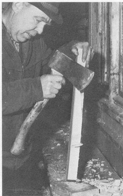
The futtock is shaped with an axe.
