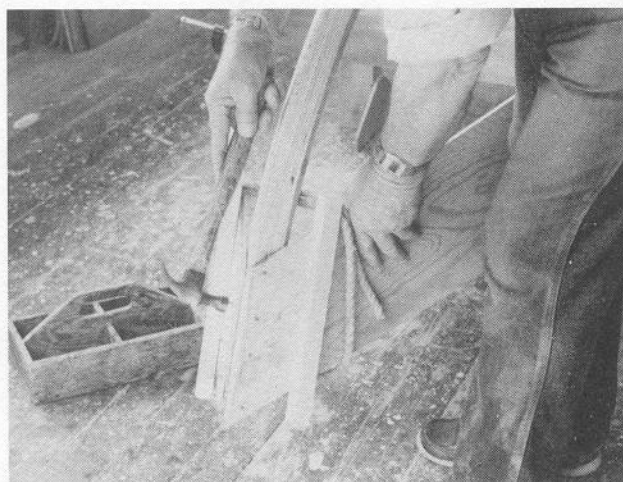
Fitting the side panels to the stem.
