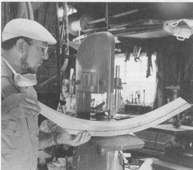
Cutting the stem bevel with a bandsaw.
