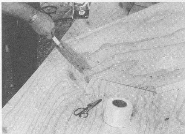
With the top cleat removed, use putty to create a fillet between the frame and the side panel.
