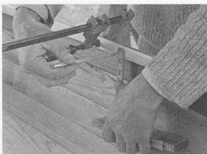
Marking the frame centerlines on the shear clamp.
