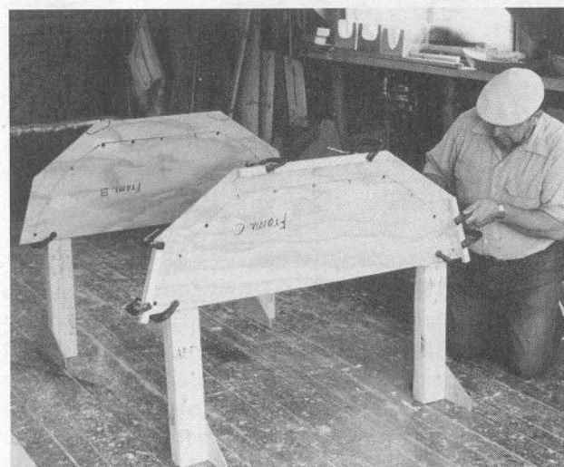
Clamping the frames to the legs.
