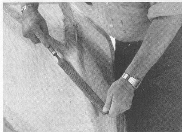
Use a rasp to round the puttied stem to shape.
