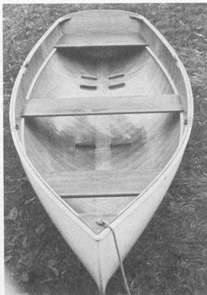
Once the panels are fastened together, the rails go on and the transom goes in. Knees, breasthook, seats, and oarlock pads complete Gull's construction.
