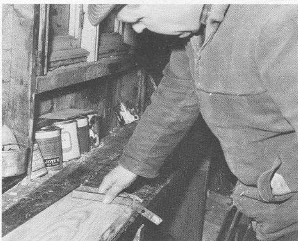
The planed plank is checked with a sliding bevel set to the appropriate mark on the bevel board.
