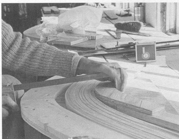
Laminating the stem.
