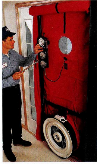
Energy audits done by power companies may use a blower door to measure airflow and detect leaks.
