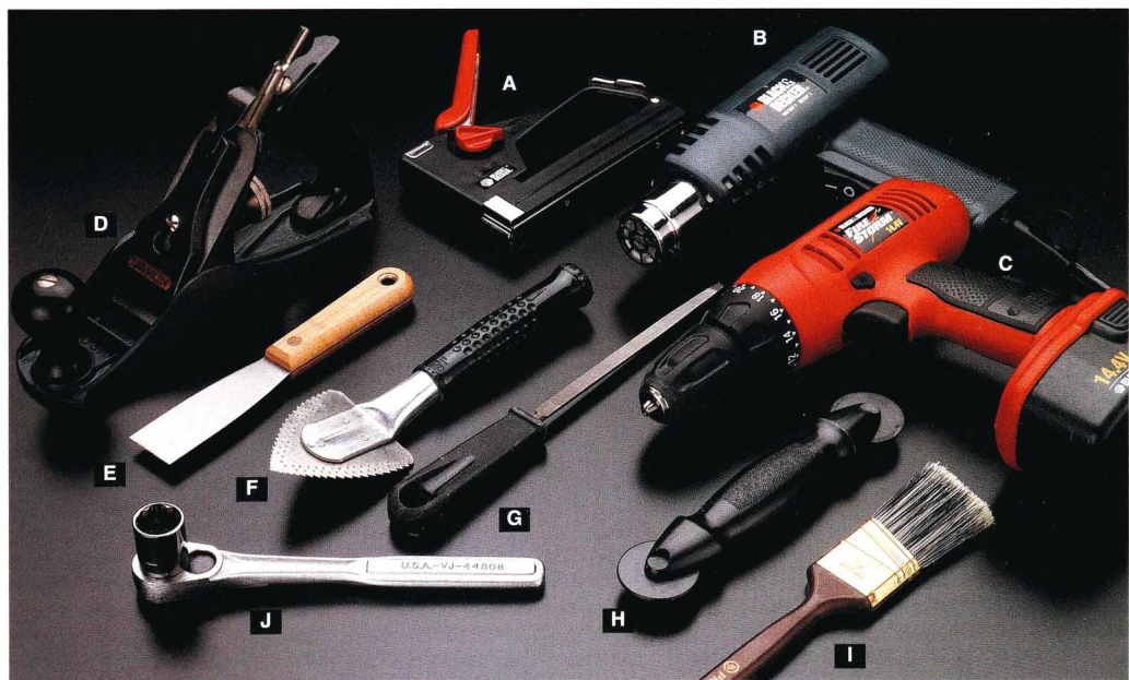
Tools for window and door repairs include: staple gun (A), heat gun (B), drill (C), plane (D), putty knife (E), window opener, sometimes called a "paint zipper" (F), metal file (G), spline roller (H), paintbrush (I), ratchet wrench (J).
