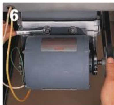
Loosen the bolts that hold the motor on its sliding bracket, and move the motor carefully until the pulleys are aligned.
