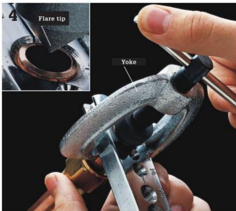
4 Slip yoke of flaring tool around base. Center flaring tip of yoke over end of pipe (inset photo above). Tighten handle of yoke to shape the end of the pipe. Flare is completed when handle cannot be turned farther.
