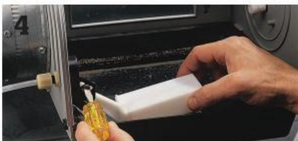
Loosen the locknut on the water line with an open-end wrench.
