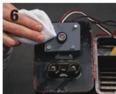
6 If the motor doesn't have cups or openings for adding lubricating oil, it's probably sealed and may not need extra lubrication.
