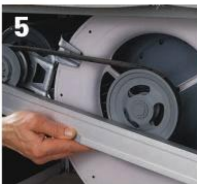
Check the pulley alignment , using a straightedge.
