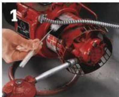
1 To clean the air intake, use a brush designed for cleaning the condensing coils on a refrigerator.
