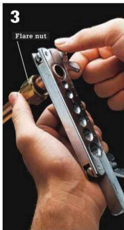
3 Clamp pipe inside flaring tool base. End of pipe must be flush with flat surface of base.
