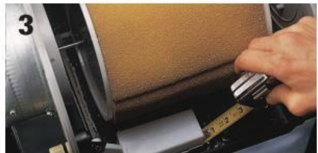
Make sure the pad soaks in the water. Mineral deposits left on the wall will indicate the original water level.
