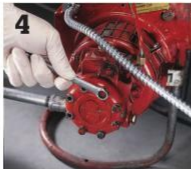
4 Leave the pump cover attached to the fuel line when you remove it.
