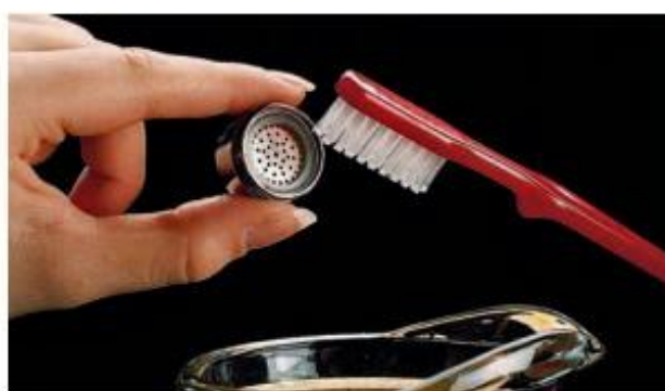
Clean faucet aerators and sink sprayers to fix most low water-pressure problems. Take aerator or sprayer head apart, then use a small brush dipped in vinegar to remove sediment.
