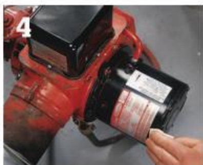
4 To prevent dust or dirt from getting in the motor while you add oil, clean off the surface with a damp cloth before opening the ports or cups.
