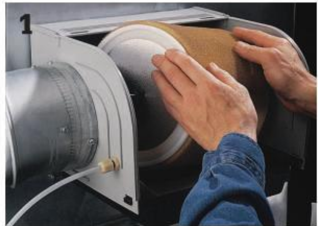
Remove the drum-style evaporator by lifting it from its slots.
