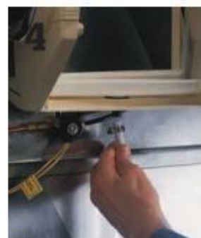
4 Disconnect the drain hose and flush it with cold water.
