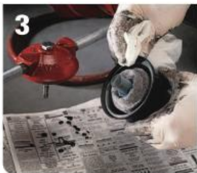
3 Wipe the edge of the cartridge, first with a solvent-dipped rag and then with a dry rag.
