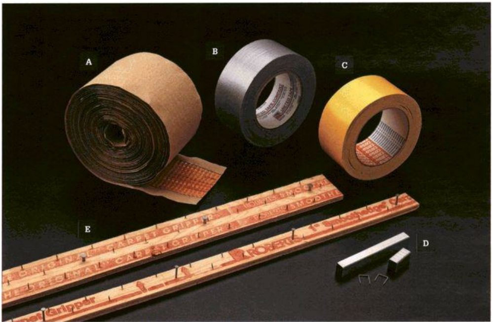
Carpeting materials include: hot-glue seam tape (A), used to join carpet pieces together; duct tape (B), for seaming carpet pads; double-sided tape (C), used to secure carpet pads to concrete; staples (D), used to fasten padding to underlayment; and tackless strips (E), for securing the edges of stretched carpet.
