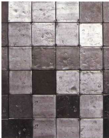
Recycled materials give old materials — and your home — new life. Here, from left to right, tile made of recycled glass, aluminum, and brass are shown.
