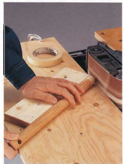
C. Use a mounted belt sander and an angle guide to create precise chamfers.
