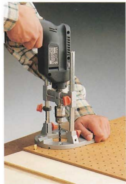
C. Drill two vertical rows of \frac{1}{4} " holes along the inside face of each side panel to hold pin-style shelf supports.
