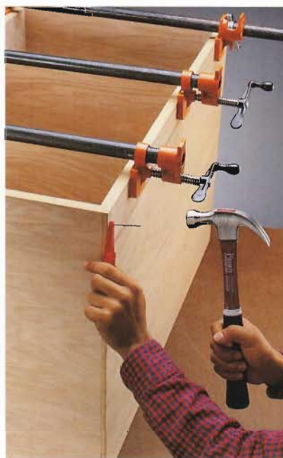
E. Reinforce each joint with 2" finish nails.
