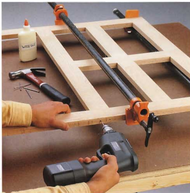
B. Measure, cut, and assemble the face frame using the dimensions and layout provided in the Base Cabinet Detail on page 27.
