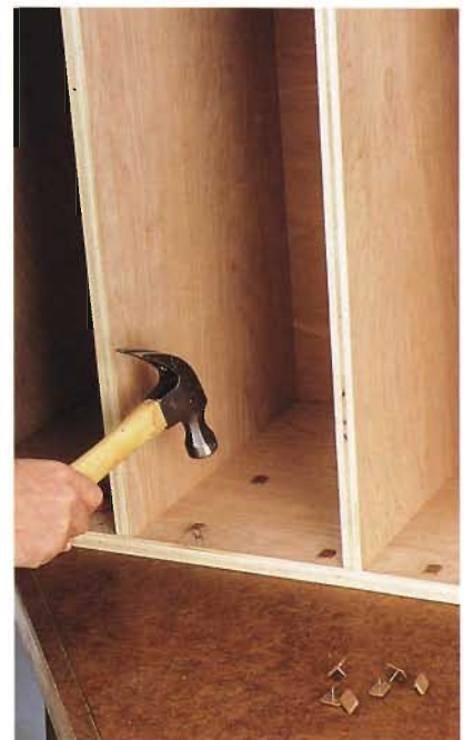
C. Tack plastic drawer glides to the inside faces of the drawer openings to eliminate friction.
