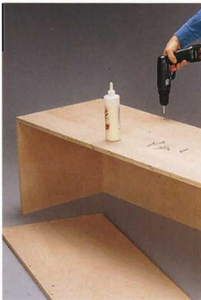
A. Attach the side panels to the top and bottom ends, and the back panel with glue and wood screws.
