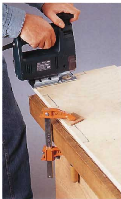
A. Use a jig saw to cut notches for the standards in the back edges of the center shelf.
