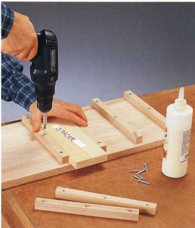
A. Use a spacer to keep the slats aligned properly, and attach them with glue and screws.
