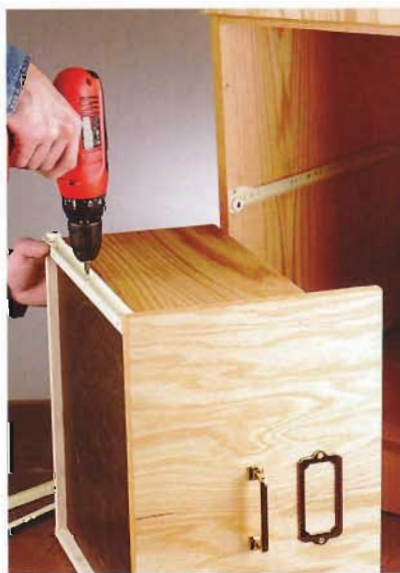
E. Attach the drawer glides to the interior of the finished cabinet following the manufacturer's instructions.
