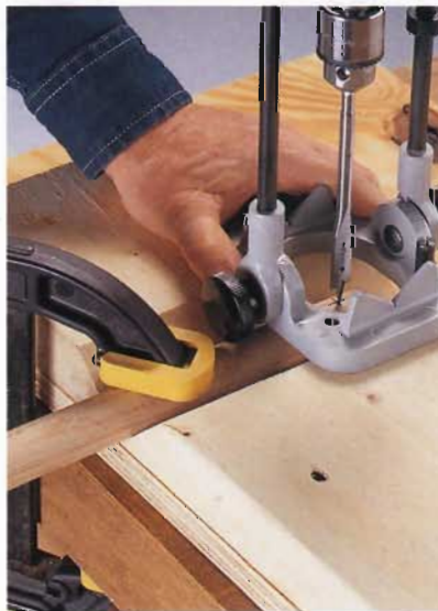
B. Clamp the rod in the V-jig and support the portable drill guide on the flat sides of the 2 \times 8 to create a straight hole.
