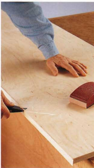
A. Apply veneer edge tape to the exposed plywood edges. Trim off excess tape with a sharp utility knife.
