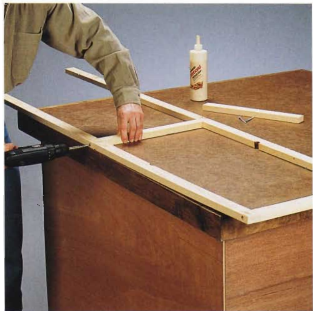
E. Assemble the rails and stiles to make the two differently sized door frames.
