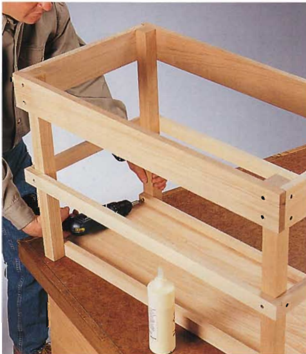
F. Fasten the bottom shelf by driving wood screws through the bottom rails and into the legs.
