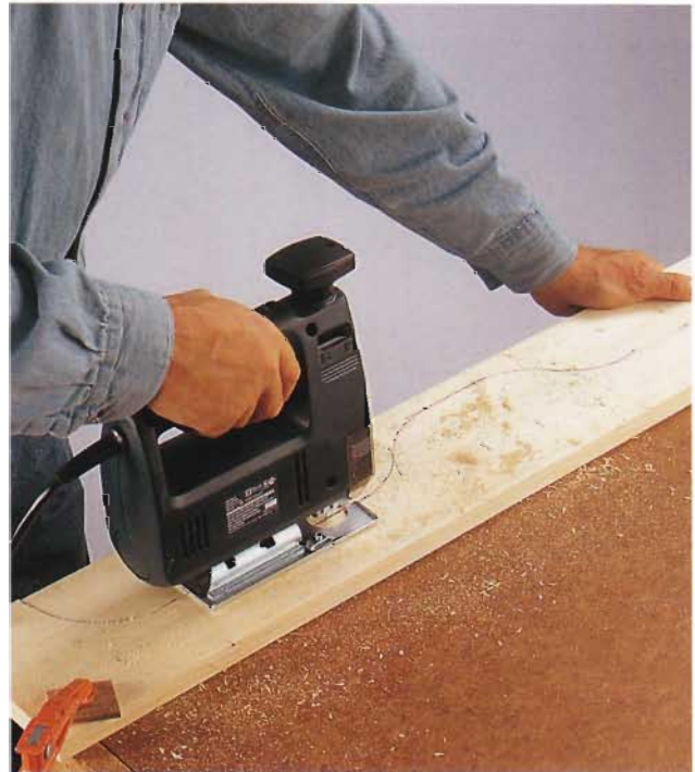
E. Use a compass to mark the decorative cutout at the bottom of the front skirt board. Then cut the curves, using a jig saw.
