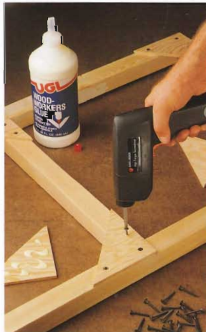
B. Assemble legs and cross braces with triangular gussets or metal connectors.
