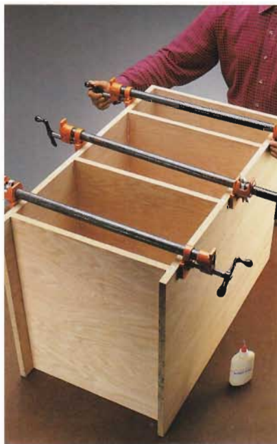
D. Glue and clamp the cabinet frames together, making sure the front edges of the pieces are flush.
