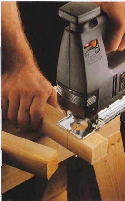
A. To build ladder brackets, cut the legs and cross braces from 2 \times 2 lumber.
