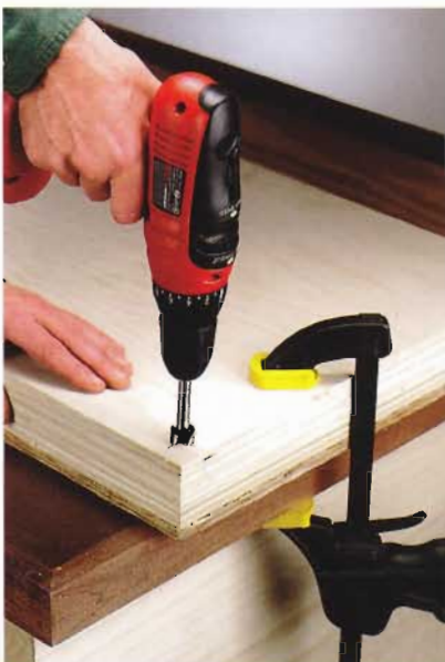
A. Mark reference lines and drill a hole at each corner of each shelf.
