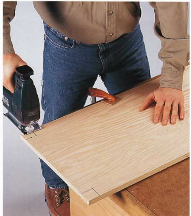
G. Cut notches at each corner of the middle shelf so it will fit between the credenza legs.
