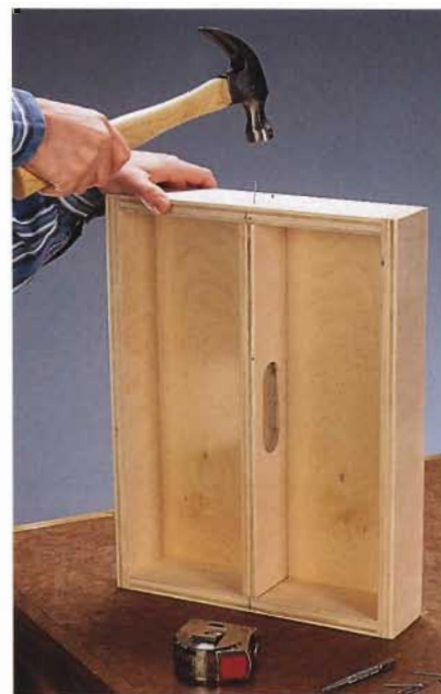
C. After making the handle cutout in the divider, attach it between the tray ends with glue and finish nails.
