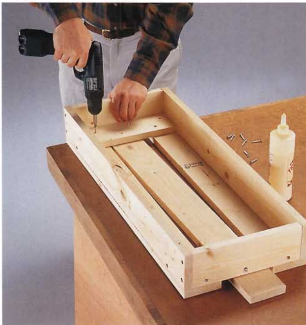
C. Join the fixed-shelf slats to the stretchers with glue and 1/4" screws driven through the underside of the stretchers.
