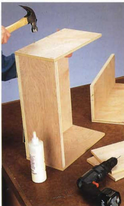
D. Fasten the sides to the front with wire nails driven through pilot holes in the sides.
