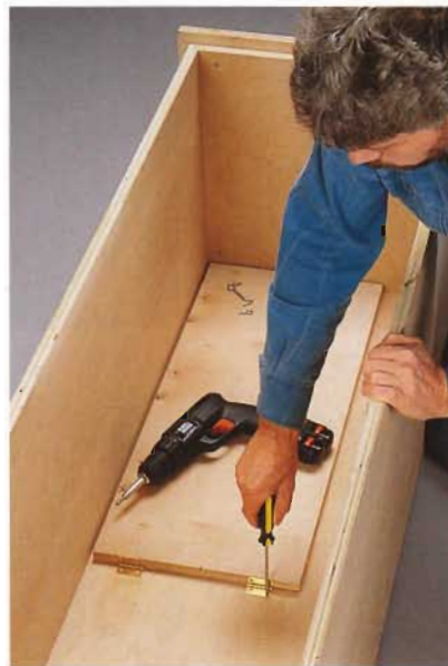
B. Screw butt hinges into the back panel to secure the drop-down shelf to the cabinet.
