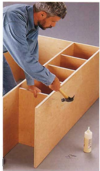
C. Fasten the shelves between the side panel and center panel with glue and 6d finish nails.
