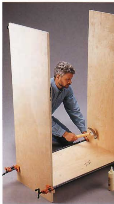
B. Clamp the bottom panel between the sides and fasten it to the cleats, using glue and finish nails.
