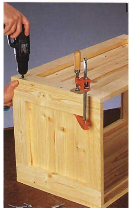
C. Secure the end panel assemblies between the side panel assemblies.
