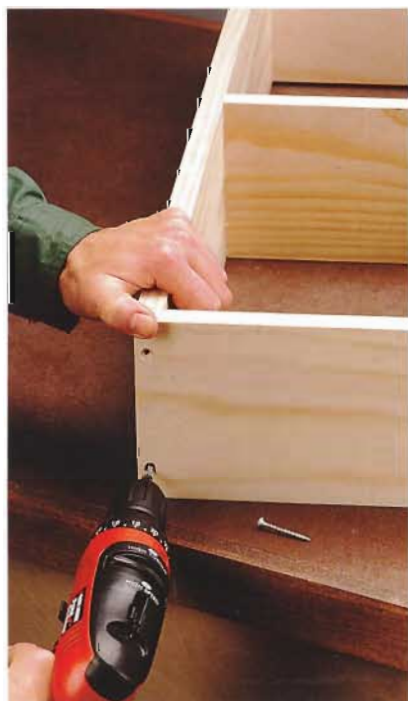
A. Assemble the frame of the box, using glue and 1½" wood screws.
