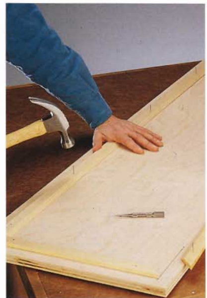
C. Attach the stop molding to the door, 1" in from the top, bottom, and side edges.
