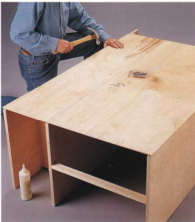
D. Nail the \frac{1}{4} "-thick back panel to the back edges of the carcass to help keep it square.
