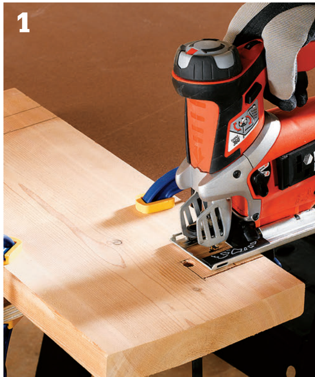
Cut the notches in the cross supports. Drill a starter hole for your jigsaw blade in one corner of each notch. Clean up the edges of the notch with a chisel, if necessary.
