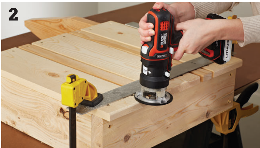
Round the sharp slat edges with a router and roundover bit or simply break the edges by sanding with a power sander.
