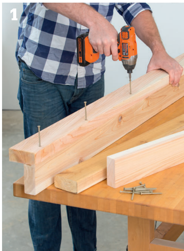
Create four legs by fastening leg sides to leg fronts at right angles.
