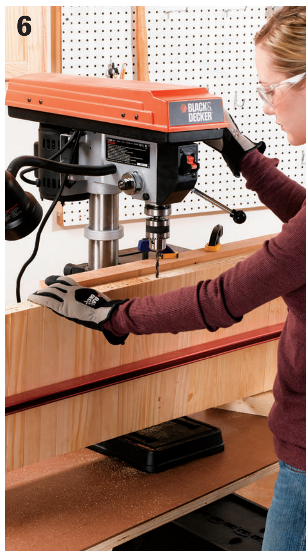
Drill mating dowel holes in the top and bottom ends of the filler stiles and the corner boards. Gang the parts together edge to edge to ensure a uniform setback from the front faces.
