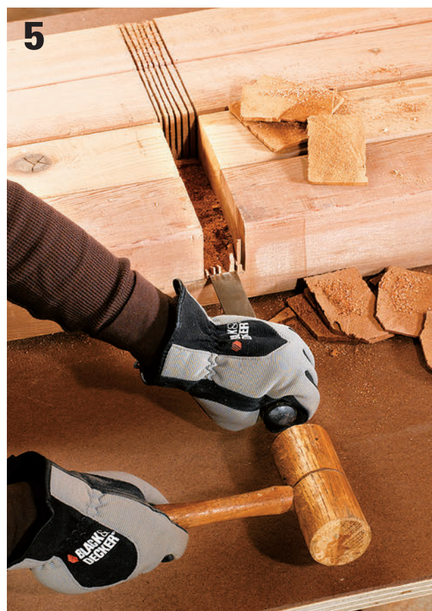
Smooth out the notches. Use a sharp wood chisel and mallet to clean up the ridges and edges left in the notch bottom after cutting the kerf.
