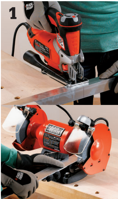
1 Cut the aluminum angle for the frame parts (top) and then deburr the cut ends on a bench grinder (lower). Don't overdo it on the grinder or use a file.
