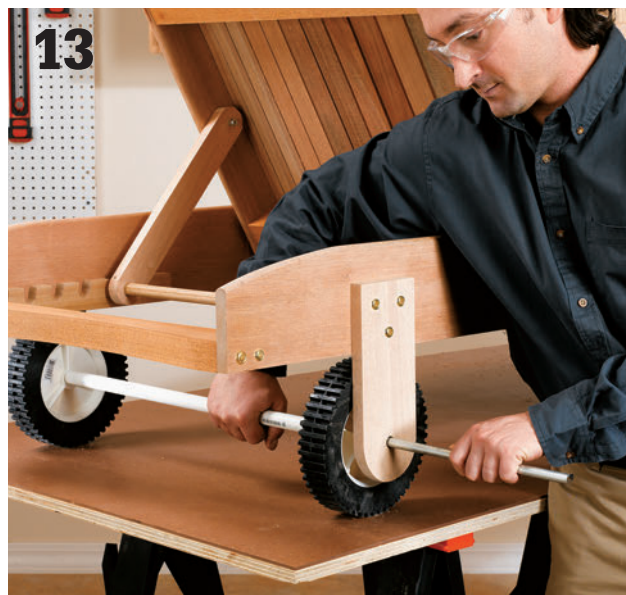
Install the axle. Slip the aluminum rod into a CPVC plastic tube sleeve and insert into the guide holes in the wheels.
