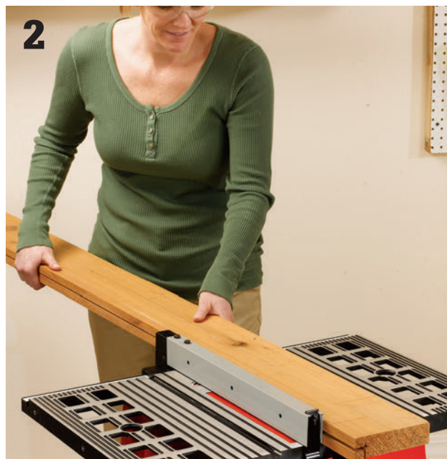
Cut panel rabbets. Make the 3/4 × 3/4" rabbet cuts in the rail stock using a table saw or router. The rabbets will accept the plywood side panels.
