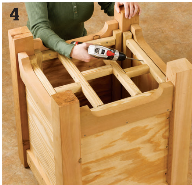
Attach the bottom braces. Assemble the braces into a square grid using adhesive and screws and then attach the whole assembly to the base rails by screwing through the four outer braces that meet the rails.
