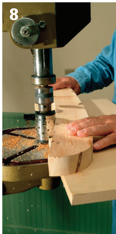
Cut out the rafters using a jigsaw, then smooth the edges. The microplane rotary shaper drill press attachment used here minimizes sawdust and cuts cedar quickly.
