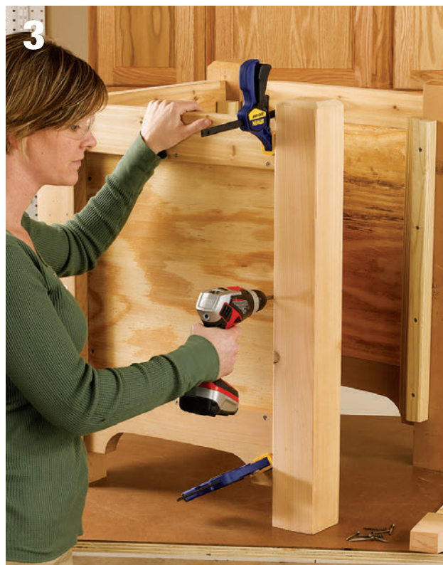
Attach the side assemblies. First, drive 3" deck screws through the corner nailers and into the rails. Then, drive 1½" deck screws through the side panels and into the nailers. Reinforce the joints with construction adhesive.
