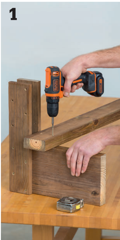
Attach the trestle to the legs, making sure it is positioned correctly against the top cleat bottoms.
