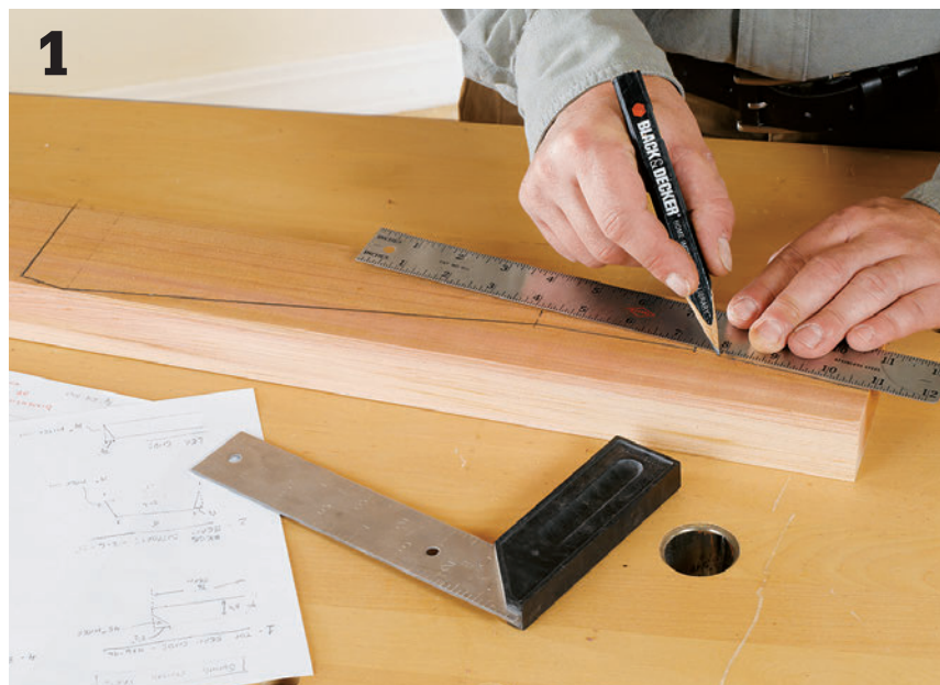
Lay out the parts. Plot the seat support profile onto one of the seat support workpieces using the dimensions given on page 39 as a reference.
