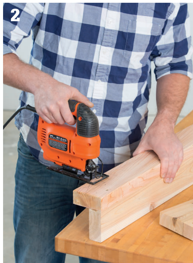
Cut a 2 x 4-size notch in the top of each of the four leg pairs to hold the crossbeams.
