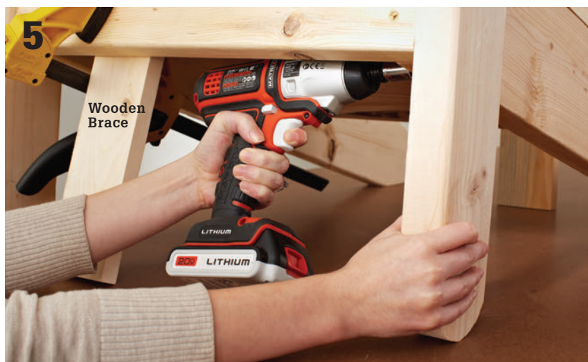
Clamp wood braces to the parts of the chair to hold them in position while you fasten the parts together.
