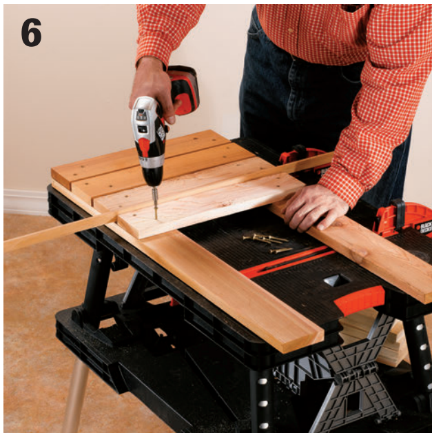
Attach the door siding boards to the door stiles. The top door siding board is attached with only one screw in each end.
