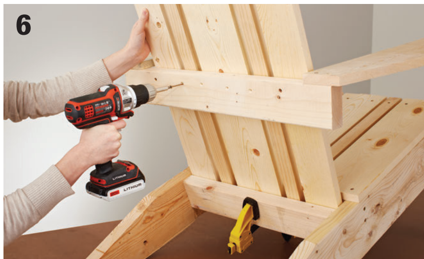
Drive screws through counterbored pilot holes in the arm cleat, near the top and into the slats. Check to make sure they did not penetrate the back slats on the seat side.
