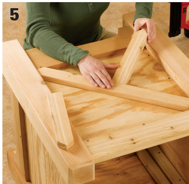
Make the X shape. The distinctive X shape on the outer surfaces of the side panels is made with 2"-wide strips of cedar that are fastened with adhesive and 1" brass brads.
