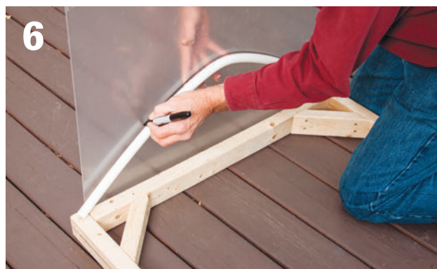
Trace the profile of the end ribs onto a sheet of clear acrylic to create a cutting line for the end panels.
