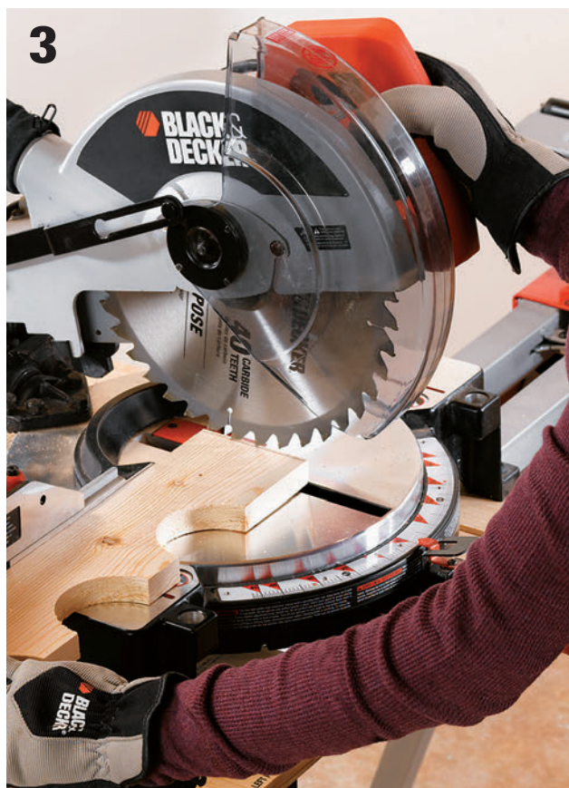
Trim the scalloped rails to length so the correct amount of uncut materials is left at each end.
