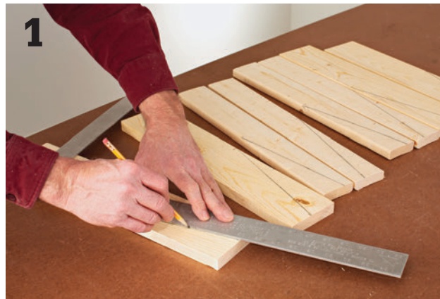
Carefully measure and mark the taper cutting lines for both the wide and the narrow sides of the legs. Work on the wide sides first, and then the narrow, to avoid mixing them up and mis-measuring the cut lines.
