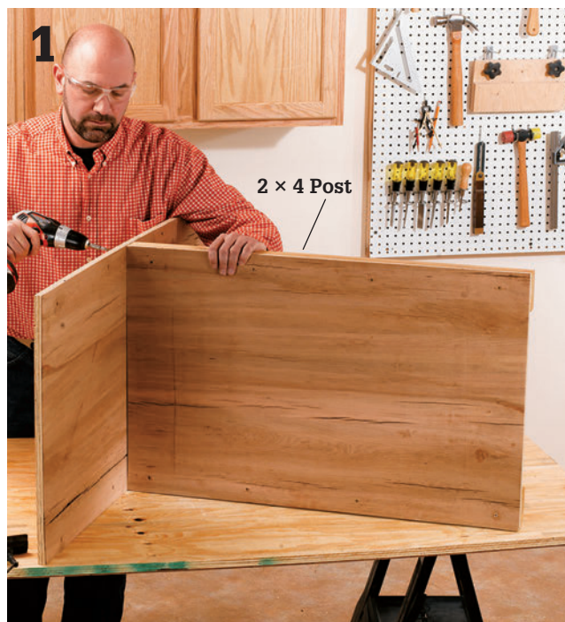
Attach the bottom panel to the posts. Drive 2\frac{1}{2} " screws through the underside of the bottom panel and into the ends of the center panel posts.
