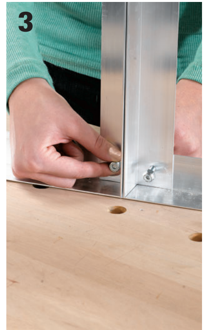
3 Assemble the frame. Secure each frame joint with a \frac{1}{4} \times \frac{3}{4} " bolt and lock nut. If you're able to locate aluminum fasteners use them, otherwise use stainless steel or hot-dipped fasteners.
