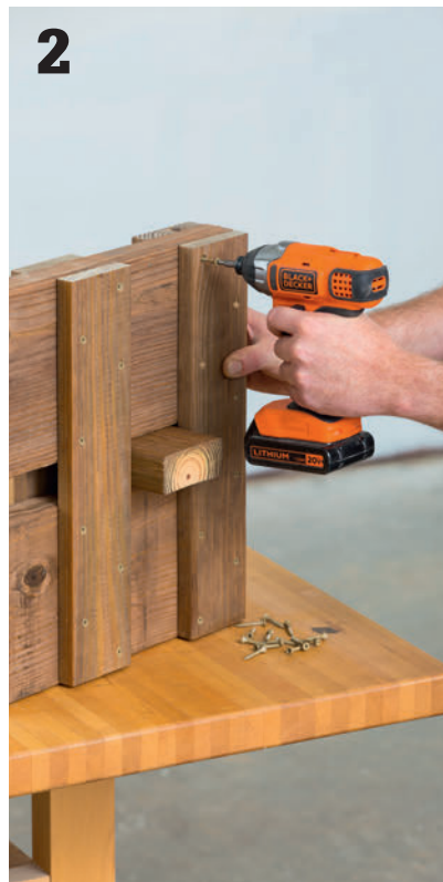
Attach the remaining leg half to the cleats on both ends, sandwiching the trestle on all sides.
