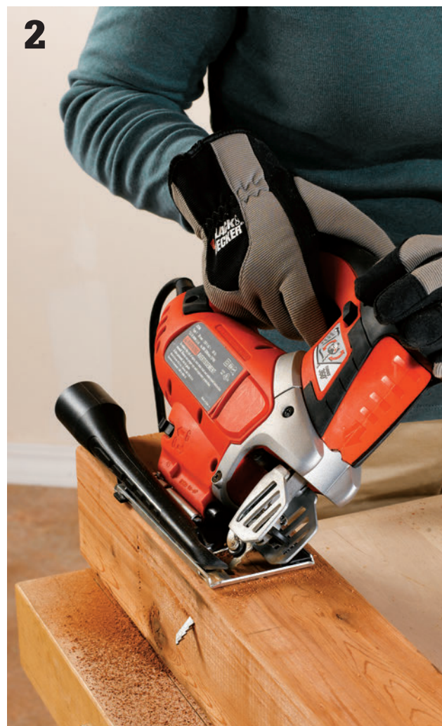
Cut the bevels. Tilt the foot of a jigsaw at a 45^\circ angle so it will ride smoothly on the post face and follow the bevel cutting line. Make a bevel cut along the layout line.
