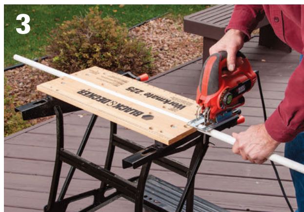
Cut the ribs for the canopy support framework from ½" PVC tubing. Make sure you're using flexible PVC and not rigid Schedule 40 PVC.
