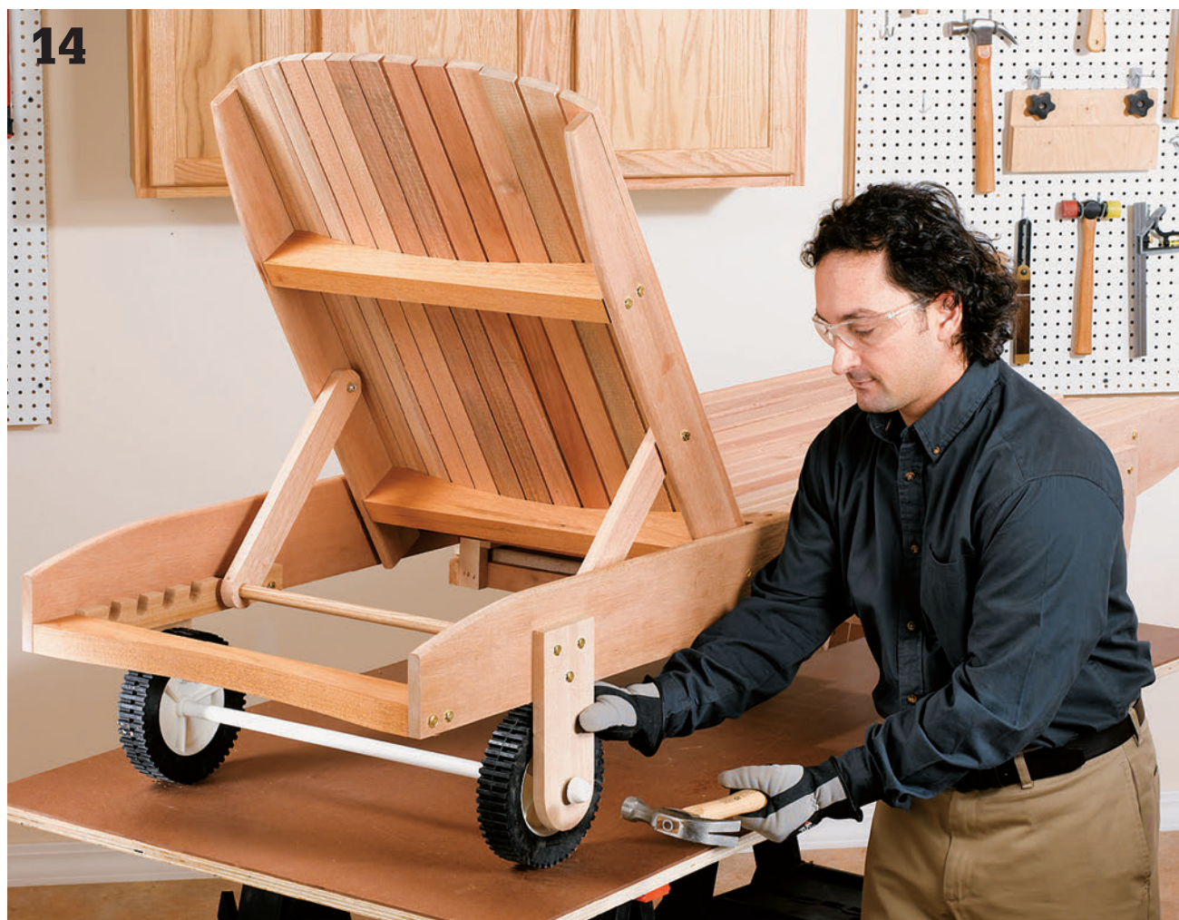
Install the wheels. Make sure the spacers ( \frac{1}{2} " inside-diameter washers) are in place on each side of the wheel and then fasten flanged push caps onto the ends of the rod to secure the wheels to the axle.
