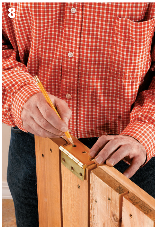
Hang the door and install hardware. Fasten the door hinges to the door (or doors if you choose to cover each opening) and then attach the door to the cart frame. Use a \frac{1}{4} " spacer under the door to position it.
