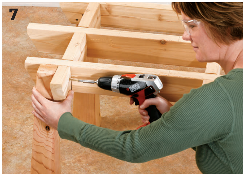
Assemble the base. The framework of the supports is fastened to the legs with 2" screws.
