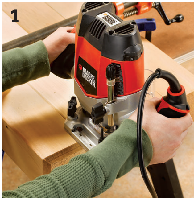
Make the posts. After cutting them to length from 4 × 4 cedar, make a 1/4" chamfer cut around all the tops. Gang the posts together for profiling if you like.
