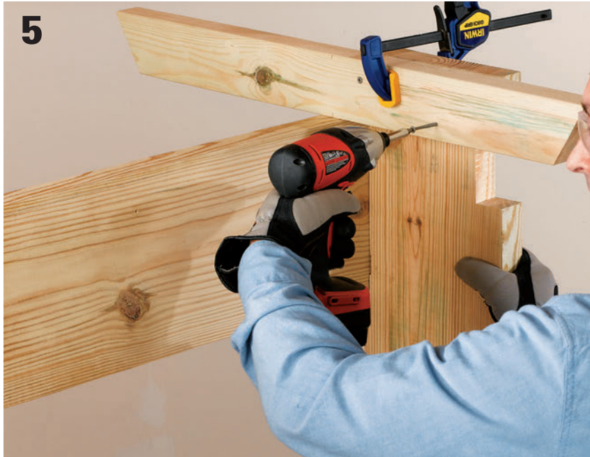
Join the supports and legs. Attach one of the cross supports to the inner leg that has already been attached to the middle stretcher.
