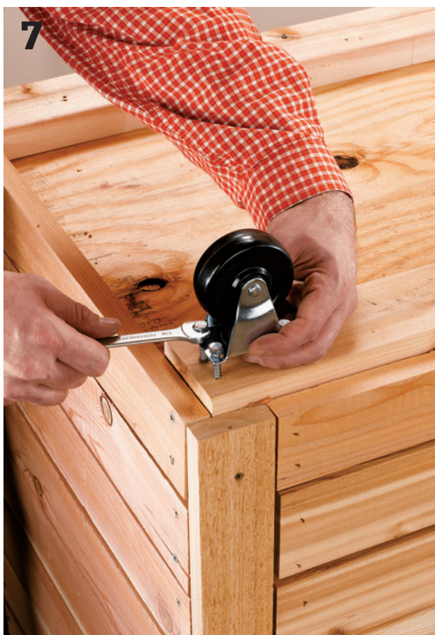
Attach the casters. Position each caster and drill pilot holes for each caster screw. Attach the casters with \frac{1}{4} \times 1\frac{1}{4} " lag screws.
