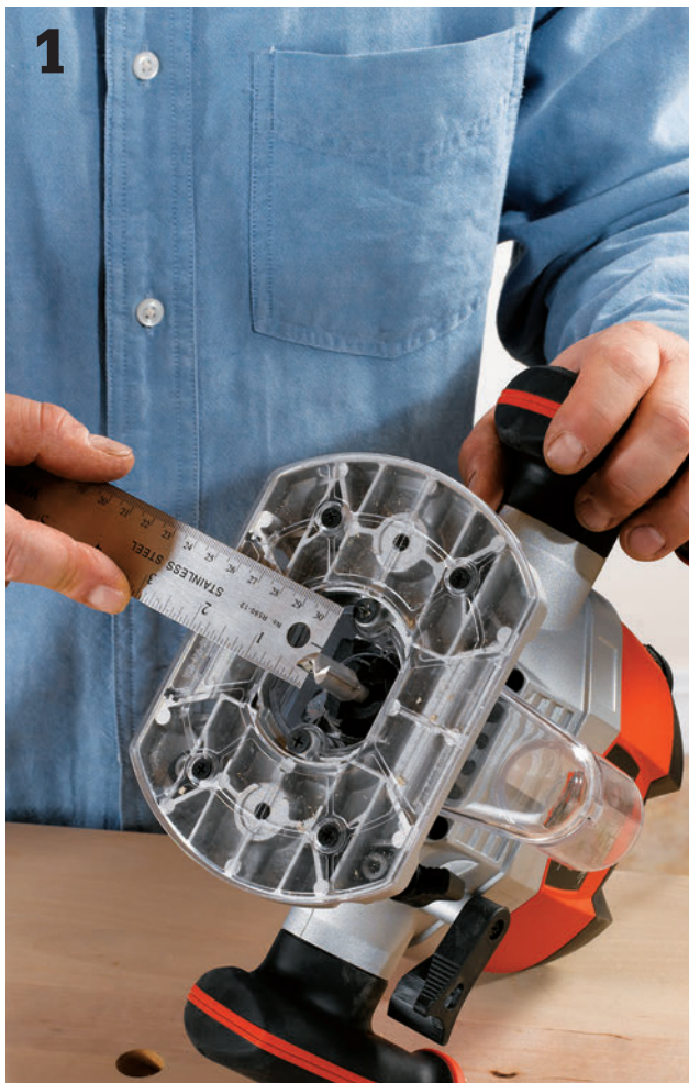
Measure the router bit setback. So you know where to place the straightedge cutting guides to cut the notches with your router, measure the distance from the edge of the straight bit to the outside edge of the base plate.
