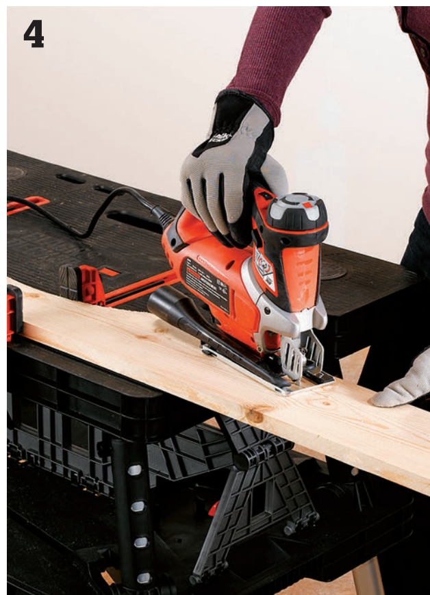
Make the 2"-deep arc cutouts on the bottoms of the rails to create the feet shapes.
