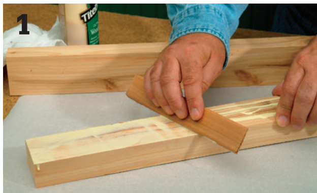
Prepare the seat slats for gluing by trimming off the bullnose edges of the 2 × 4 stock and spreading an even layer of exterior-rated wood glue onto one face in each face-glued joint.
