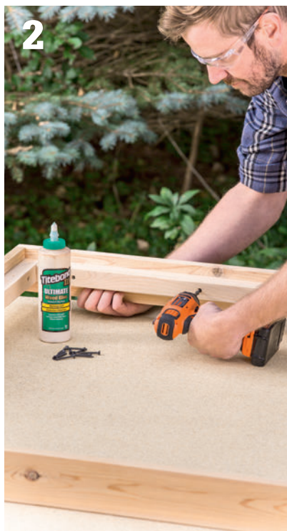
Attach the end cleats to the inside faces of the end rails. Maintain a \frac{3}{4} " distance from the top edge of the rails to the top edge of the cleats.
