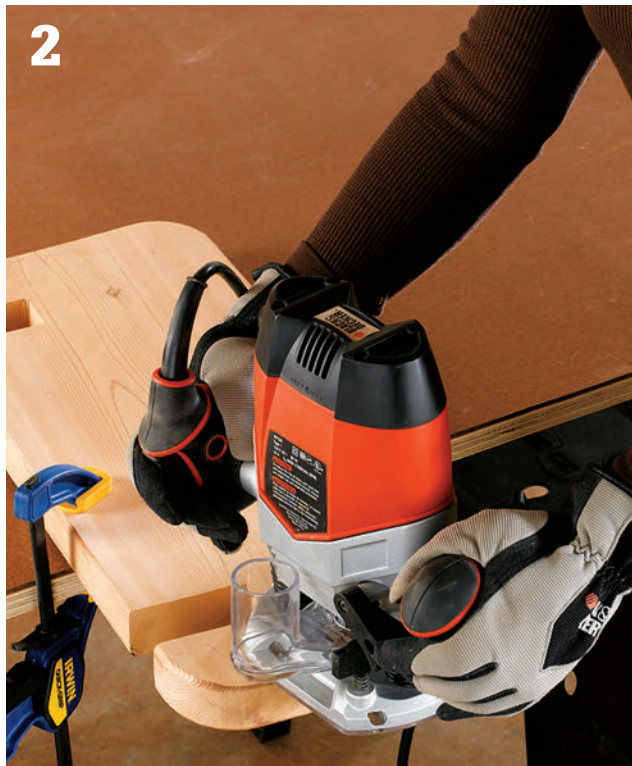
Round over the part edges. Ease the outside edges of the cross supports with a router and \frac{1}{4} " roundover bit. Leave the edges of the cross-support notches square.
