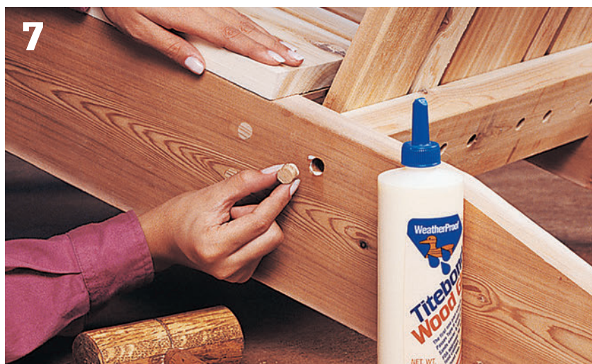
Glue cedar plugs into the counterbores to conceal the screw holes.
