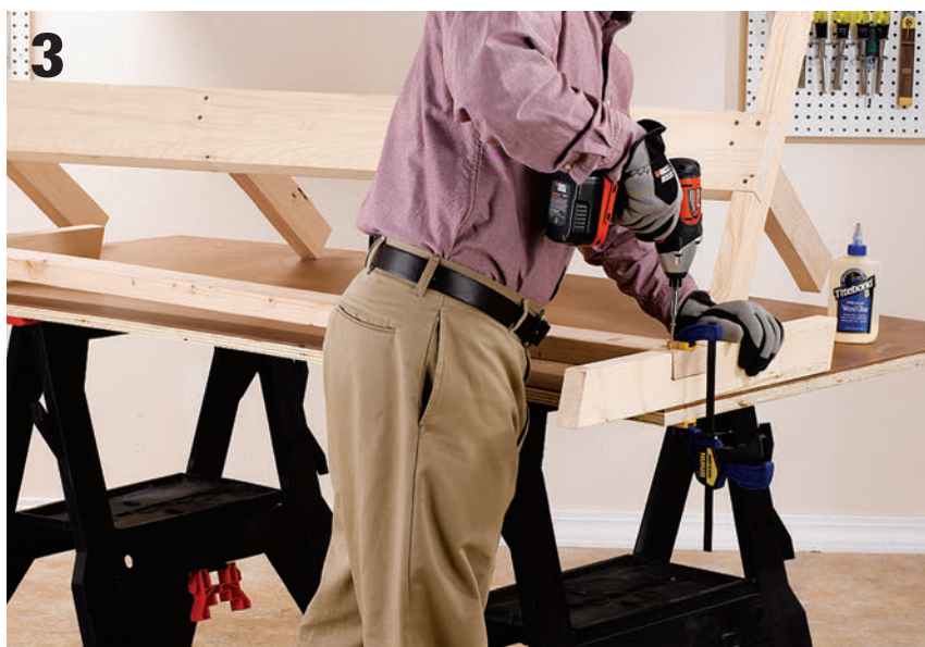
Attach the rails. The front rails should be attached to the front legs and the back rails are attached to the back legs. Use exterior wood glue and 2½" deck screws.
