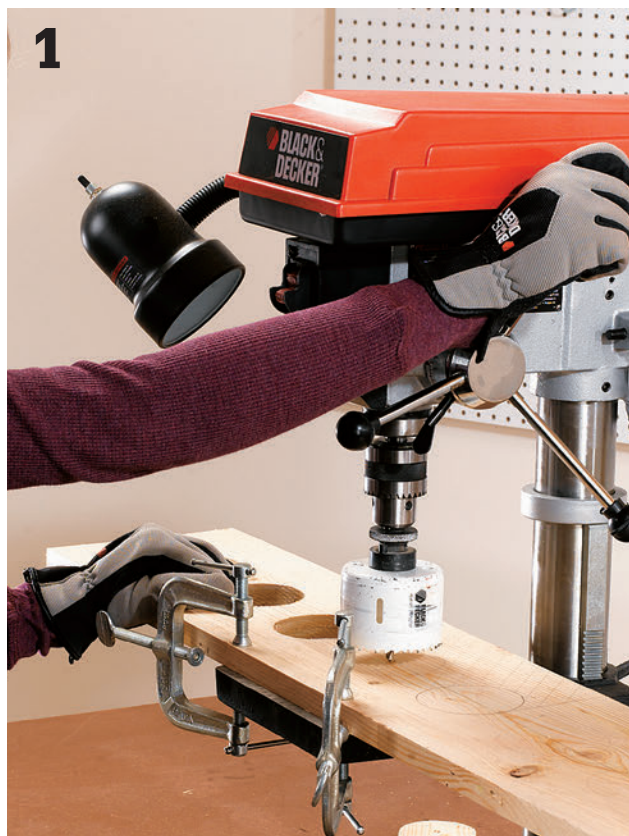
Cut out 3"-dia. circles along a centerline on a 1 \times 8 workpiece to make the top rails. Use a 3" hole saw to cut the wood.
