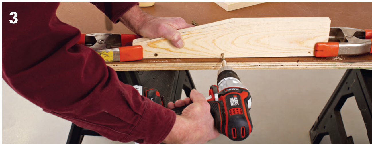
Work on a perfectly flat surface to ensure the leg sides are exactly aligned. Apply a bead of glue where the inside face overlaps the edge of the smaller leg piece, and then drill three countersunk holes and screw the pieces together.
