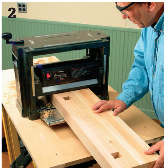
Glue the seat platform in two sections that are narrow enough to fit in a planer; then plane the sections (and the stock for the armrests) to the final thickness.
