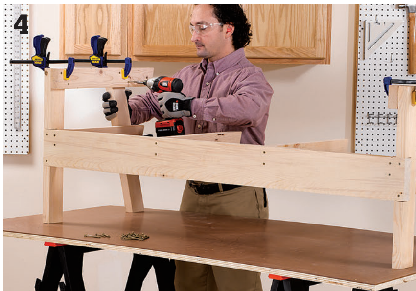
Attach the supports and legs. Temporarily clamp the parts together in the correct orientation and then drive 2½" screws through the inside faces of the arm supports and seat supports to attach them to the legs.
