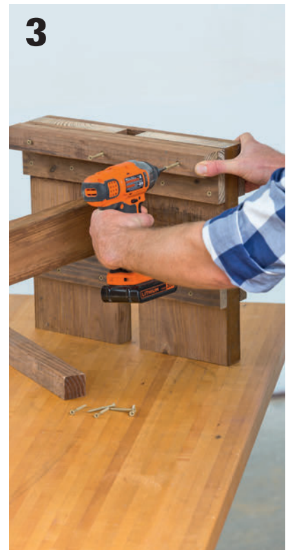
Attach the outer brace for the seat slats directly to the inside faces of the cleats.
