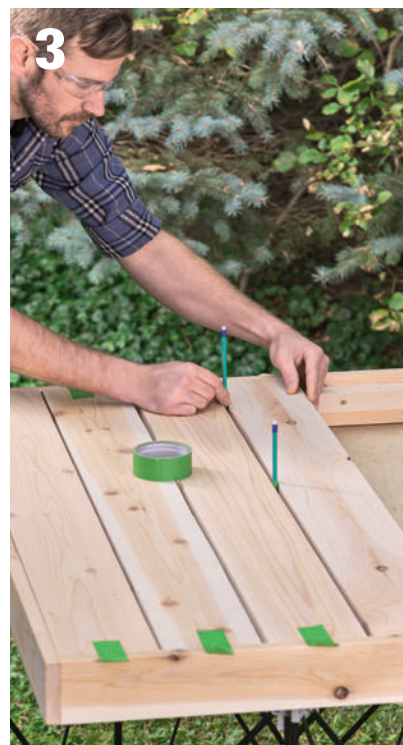
Install the tabletop slats. Use pencils or dowels as spacers to set even gaps between top slats. Tape the slats in position with masking tape.
