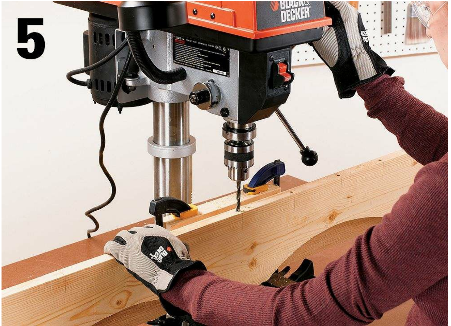
Drill dowel holes in the top and bottom rails to make dowel joints with the filler stiles and the corner boards.
