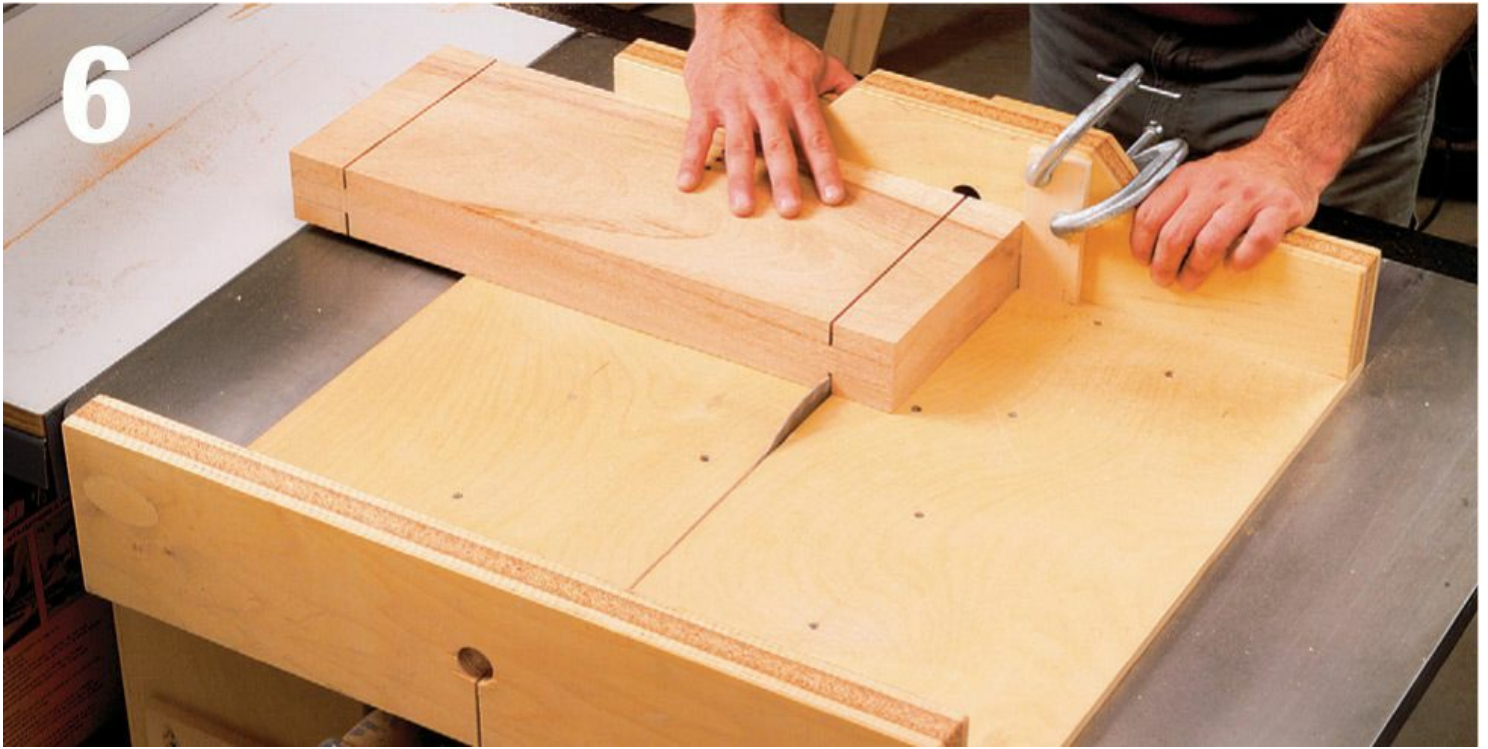
Cut the tenon shoulders using a table saw crosscut sled. Clamp a stop block to the sled to ensure consistent cuts.
