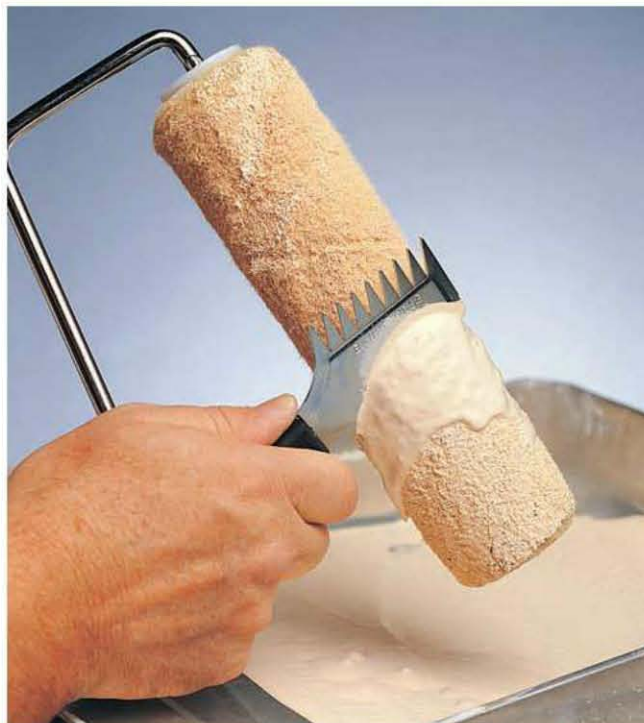
Scrape paint from a roller cover with the curved side of cleaner tool. Remove as much paint as possible before washing the tools with solvent or water, depending on your paint.
