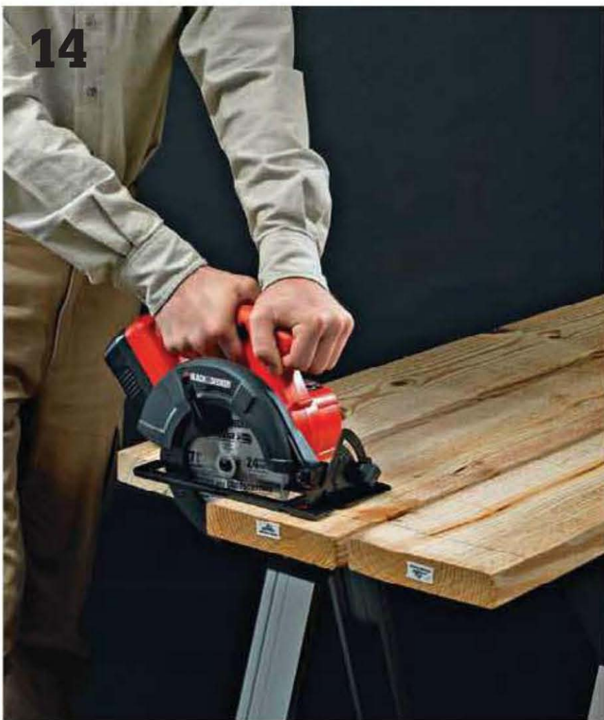
14 Measure and mark lumber for joists, using a combination square as a guide. Cut joists with a circular saw or power miter saw.
