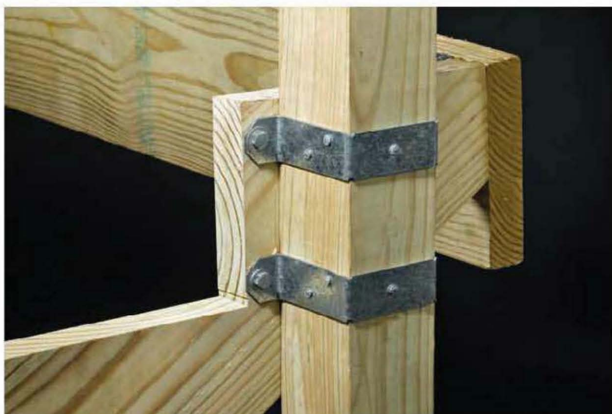
Deck post ties fasten stair or railing posts to stringers or joists without through bolts. Hardware is manufactured in 2 × 4 and 4 × 4 size options.
