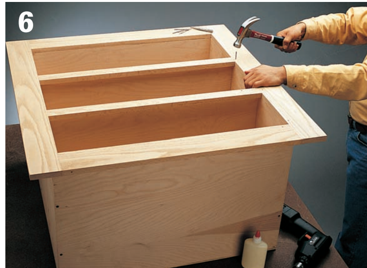
Attach the face frame to the front edges of the cabinet, using glue and finish nails.
