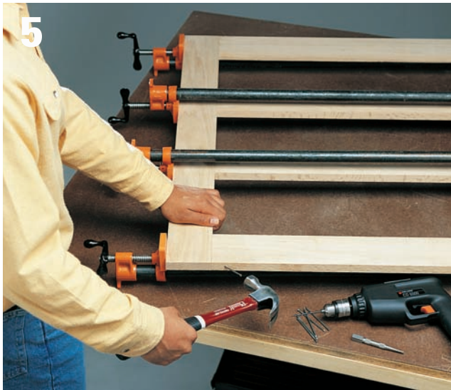
Assemble the face frame pieces , and reinforce the rail-and-stile joints with toenails.
