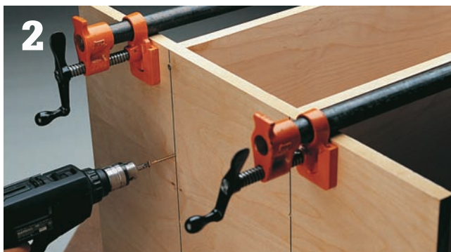
2 Draw layout lines for the shelves, then attach them between the side panels with glue and screws.
