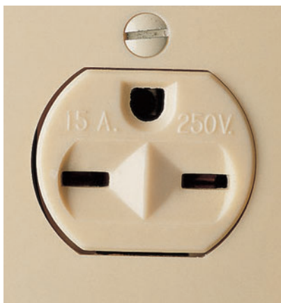
15 amps, 250 volts. This receptacle is used primarily for window air conditioners. It is available as a single unit or as half of a duplex receptacle with the other half wired for 120 volts.
