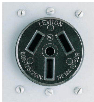
50 amps, 125/250 volts. This receptacle is used for ranges. The high-voltage current powers heating coils, and the 125-volt current runs clocks and lights.
