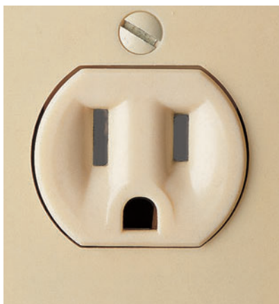
15 amps, 120 volts. Three-slot grounded receptacle has two different sized slots and a U-shaped hole for grounding. It is required in all new wiring installations.
