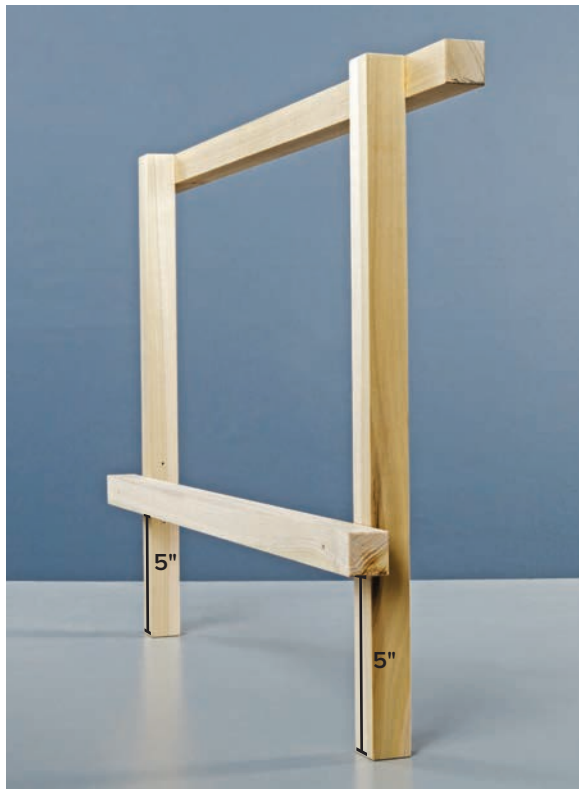
BACK SUBFRAME ASSEMBLY upports the seat back.
