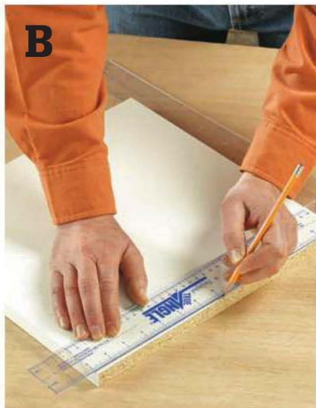
Transfer your measurements to a sheet of melamine (or shelf stock without predrilled holes).
