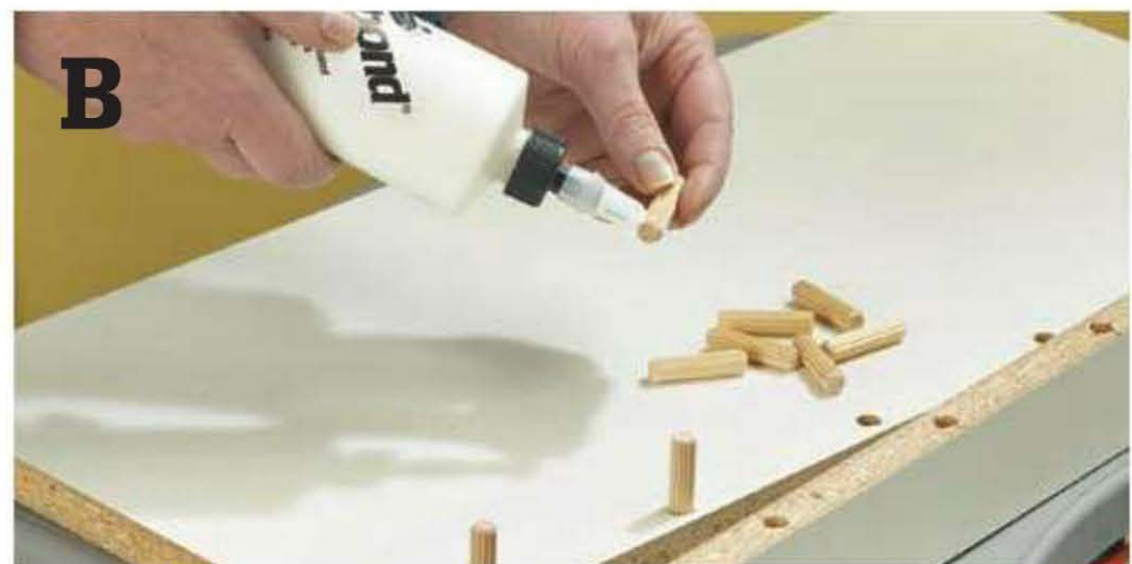
Apply glue to the dowels and insert them into the shelf holes. Fasten the 1 × 2 cleat to shelf with 1½" fluted dowels in the cleat.
