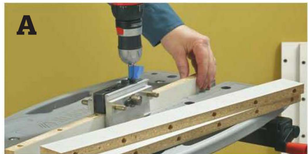
Drill ½"-deep dowel holes every 3" to 4" on the shelves, and drill 1¼"-deep dowel holes every 3" to 4" on the cleats.
