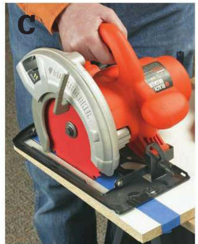
Cut the top shelf , using a circular saw with a melamine blade. Place painter's tape along cut lines to prevent chipping—this is especially helpful for cutting angles.
