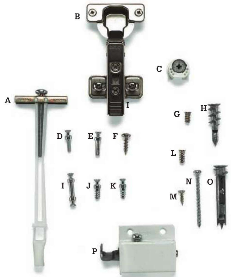
A. Toggler SnapToggle 1/4-20, B. Euro cabinet door hinge, C. knock-down fitting (KD), D. connecting bolts (KD dowel), E. a single connector bolt, F. panhead screws, G. Euro screw, H. self-drilling anchor, I. double-ended bolt (KD screw/dowel connector), J. connecting bolt (KD screw), K. connecting bolt (KD screw), L. Euro or “barrel” screw, M. flathead screw, N. machine screw, O. self-drilling toggle, P. hanging bracket (fastened to verticals).
