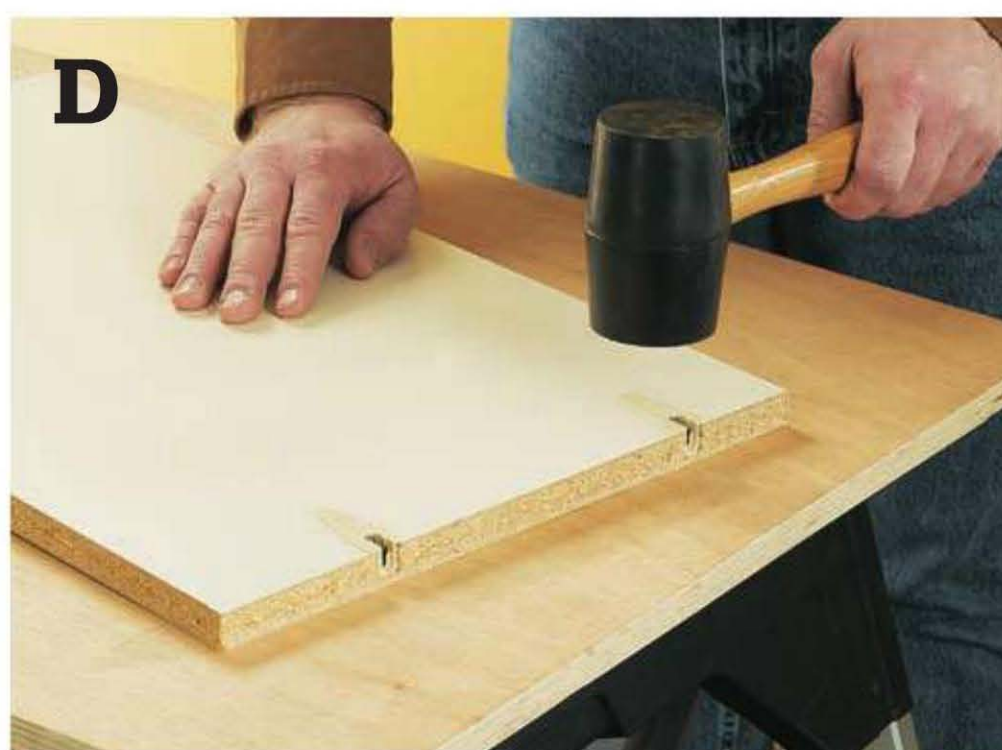
Tap KDs in to place on fixed shelves using a rubber mallet.
