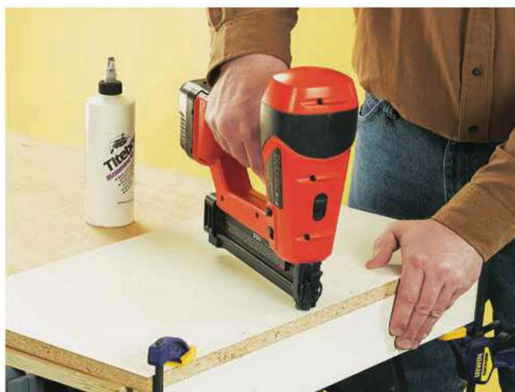
Option: Fasten the cleat to the underside of the fixed shelf using glue and pin-nails.
