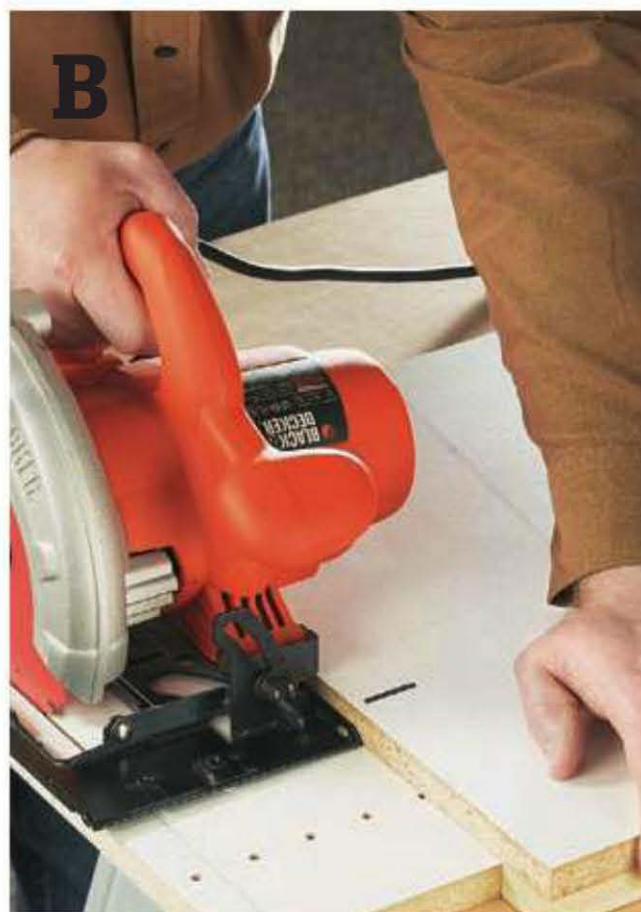
Cut the top shelf with a circular saw with a melamine blade.
