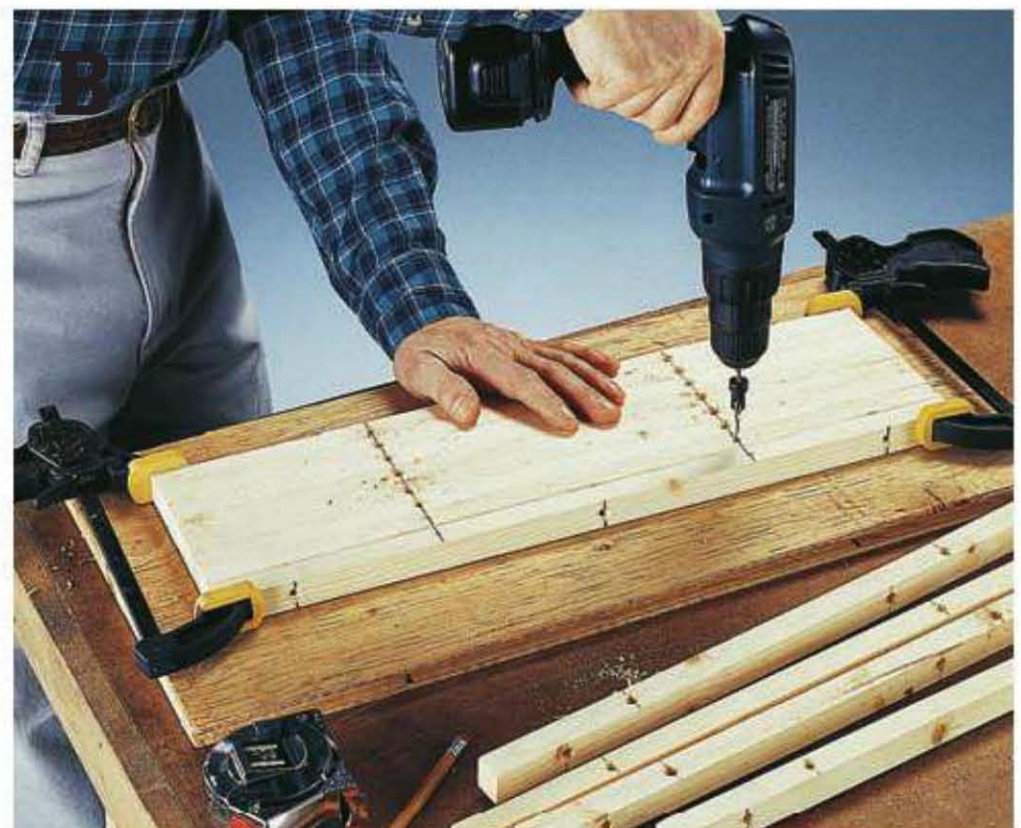
Gang the cleats together while drilling countersunk pilot holes.
