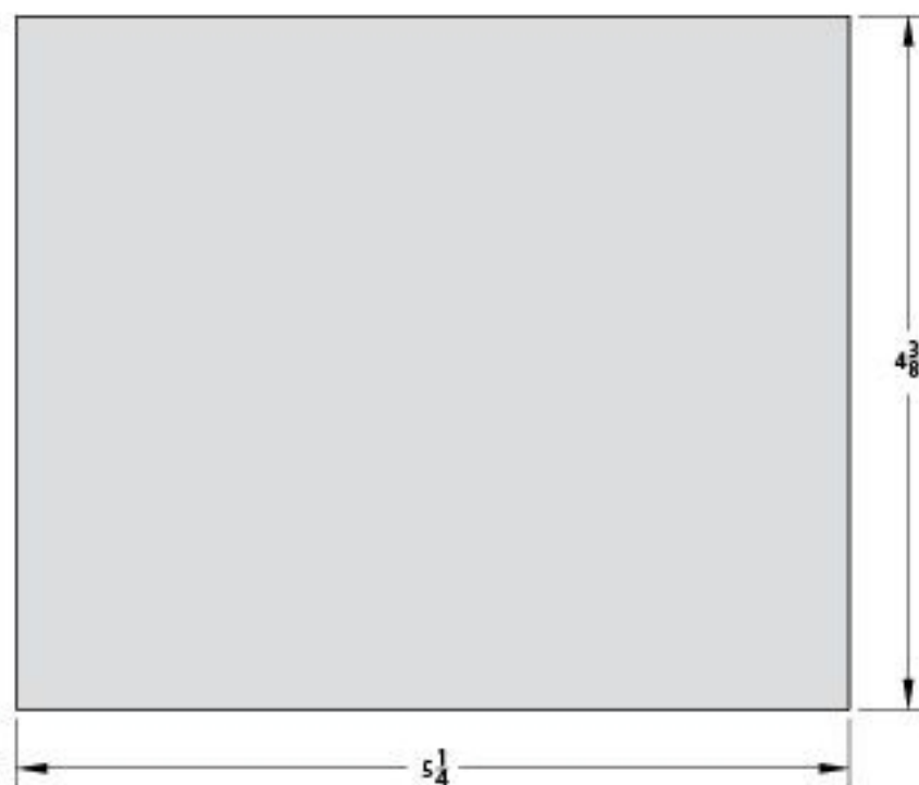
ROOF A 5/8" \times 4-3/8" \times 5-1/4"
