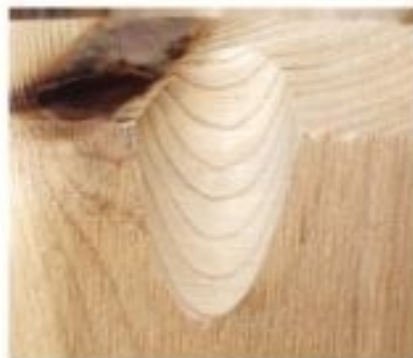
A finger recess in the Right Side Bottom piece makes it easier to lift the side door.
