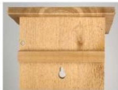
Use a cleat at the back of the birdhouse to make sure it tilts forward once mounted.
