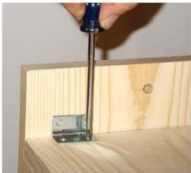
Install the hinges. Install the hinges with a #2 Phillips-head screwdriver.
