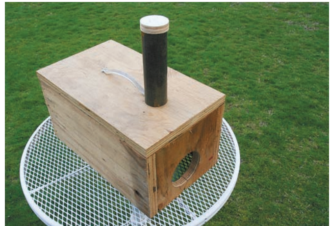
The steel pipe affixed to this removable nest box lid allows the photographer to drop a camera into the burrow. Steve Simmons
