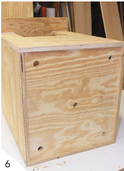
6 Recess the floor 1/2" . Drill four or five 1" diameter drainage holes into the floor.
