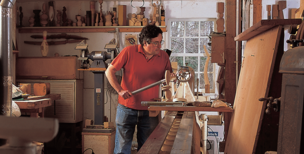
Mark Sfirri at his lathe, a Oneway to which he has added two full-bed extensions for a 13' capacity.
