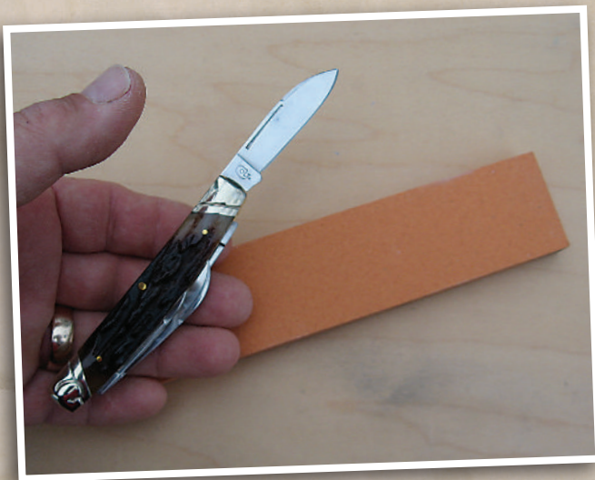
An India stone is commonly used to sharpen a pocket knife.
