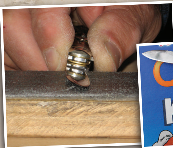
Stropping should be done at this angle.
