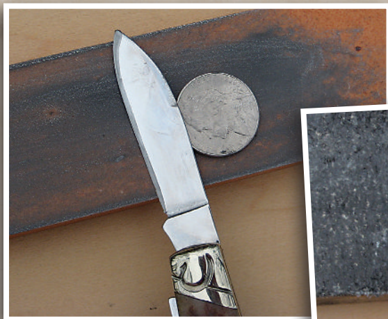
Just reverse the grinding to properly bevel the other side of the blade.
