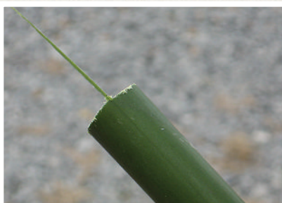
4. If you do saw the cane, or other tube material, it will leave some fibers that will need to be trimmed.
