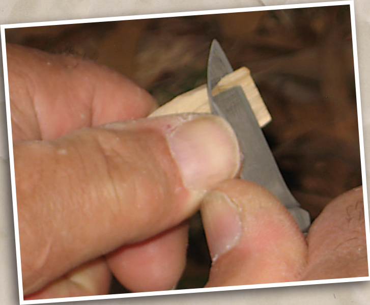
This is the thumb push cut—very precise.
