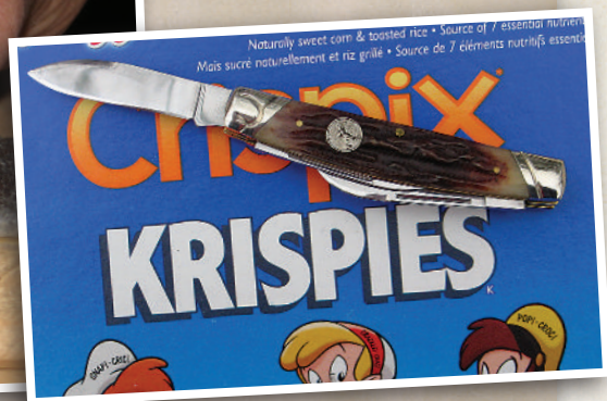
In a pinch, use box board as a strop.
