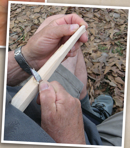
Here is the pull cut.
