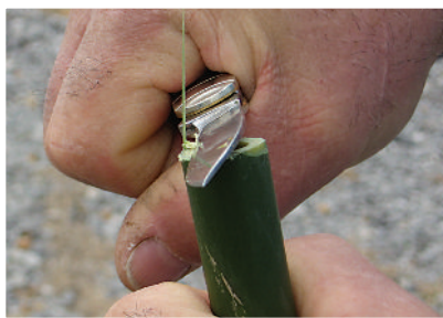
5. Do not cut from the center towards the outside as in this picture.
