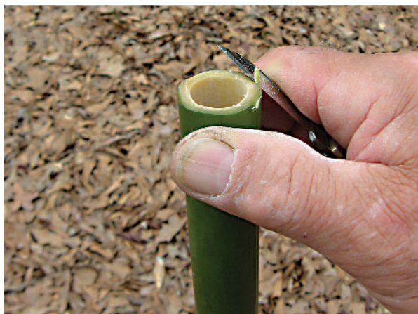
2. Carefully smooth the sharp edges off of the outside and inside of the mouthpiece end of the trumpet.
