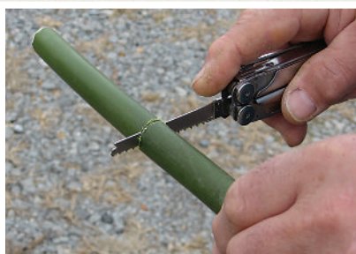
3. The saw on a multi-tool is useful for cutting cane.
