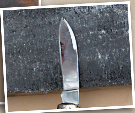
Stropping is the finishing touch to make a blade really sharp.
