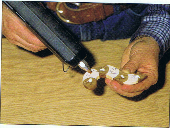
Photo 5:8 Place a couple drops of hot glue, as well, on the back of the tail section.
