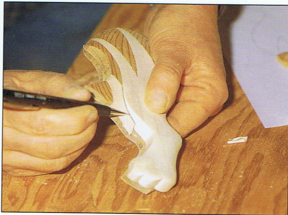
Photo 3:16 Reassemble the pieces to check the "stair step" between the stomach and the leg and mark the height with a pencil. Disassemble the pieces.
