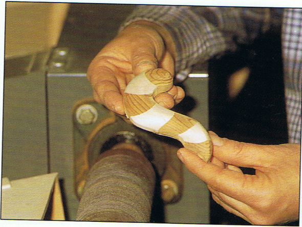
Photo 3:8 Using the drum sander, rough-in the tail section. The edges of the tail should taper down to about \frac{1}{4} " where it joins the body.
