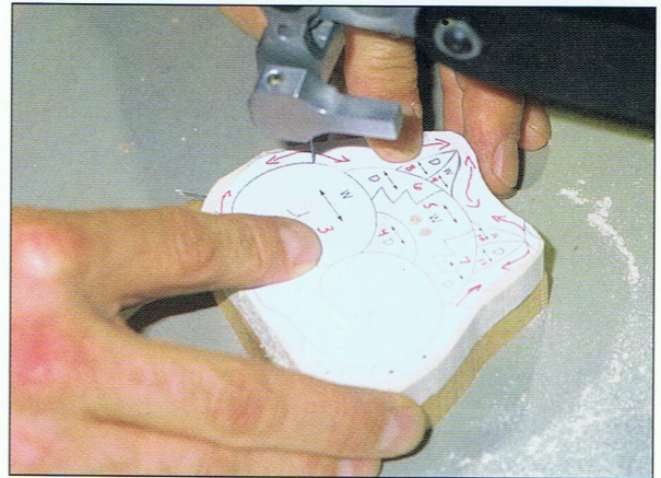
Photo 2:9 Cut the head section. Be careful to follow the lines exactly on the right side where the cat's head meets the body.
