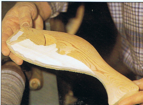
Photo 2:8 Taper the body down at the base of the tail and up at the tip of the tail to add to the appearance of a flipping tail.
