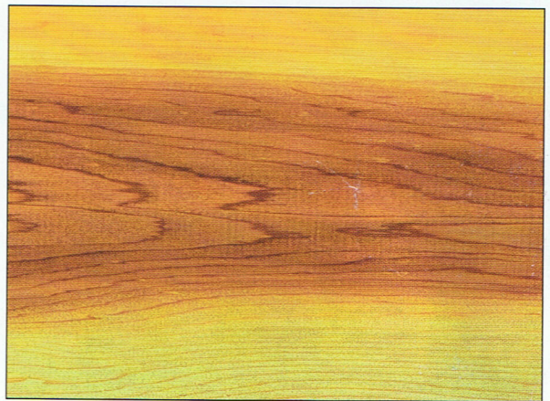
Photo 1:2 Though it is hard to find, red cedar sap wood can be used as white-colored wood in place of the more common basswood, pine or aspen.
