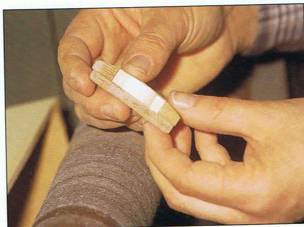
Photo 3:23 Round the upper head section back toward the ears. Lower it to about \frac{3}{8} ".
