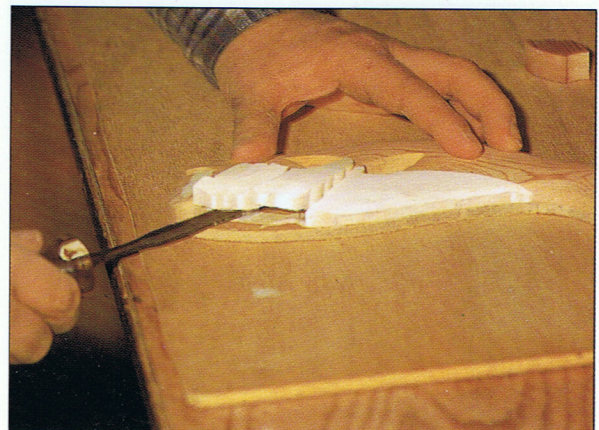
Photo 2:9 Take apart the gill section. Use the sander and a chisel to give it a layered look.
