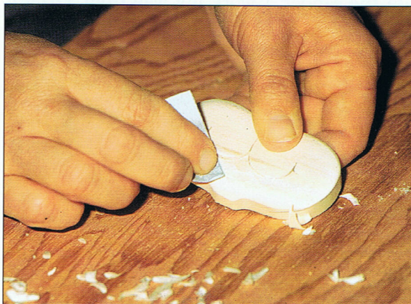
Photo 3:30 Hand-sand the area under the smile to achieve a smooth surface and eliminate any "step" between the areas.
