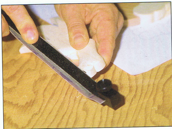
Photo 3:20 Use an Intarsia Detail Sander to blend the toes into the surrounding area.
