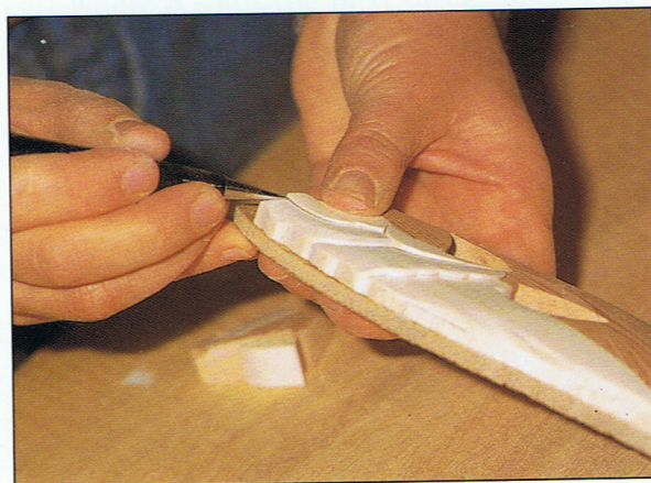
Photo 2:13 Continue this process tapering toward the next un-sanded part each time to give a stair-step pattern, until you reach the mouth.
