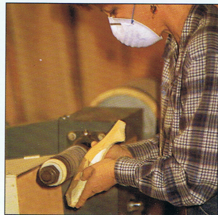
Photo 2:7 Rough-in the body of the fish. Do not remove wood below the pencil marks you made to indicate the height of the fins.
