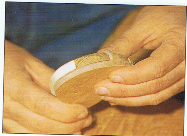
Photo 3:13 Sand the pieces that touch the face and the one paw down to about \frac{1}{4} ". Leave the area around the tail thicker.
