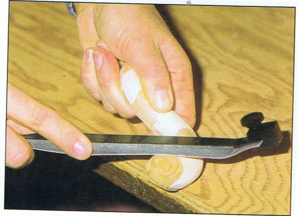
Photo 3:9 Use an Intarsia Detail Sander to rough-in the areas around the sharp curve in the cat's tail.
