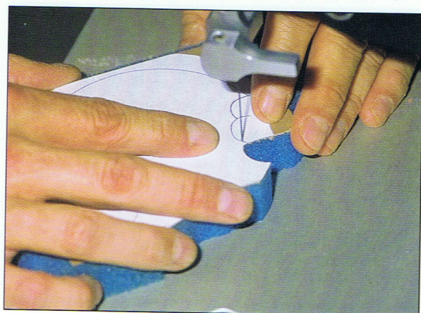
Photo 4:1 A tight-holed sponge is used for the ball. Use spray adhesive to attach the pattern to the cardboard and then to the top of the sponge. Cut the sponge with a scroll saw.
