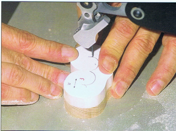
Photo 2:16 To make the cut for the mouth, follow along the lines to the end of the smile.
