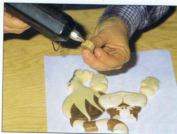
Photo 5:1 Apply a clear finish to all the parts. Glue some of the stripes together. Here, I am gluing the tail section.
