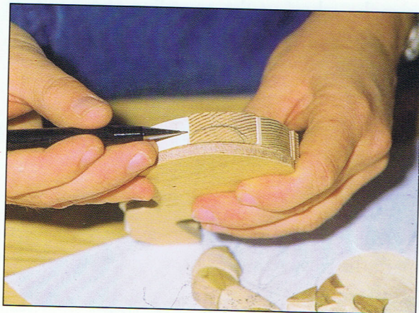
Photo 3:12 Mount the pieces from the hind leg section on a sanding shim. Note the pencil mark added in Photo 3:11.
