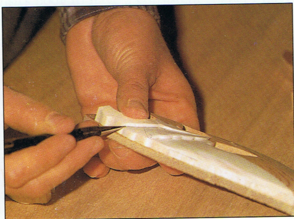
Photo 2:12 Sand this gill part, tapering it toward the mouth or the next un-sanded part. Mark this part where it joins the next piece.
