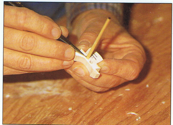
Photo 3:37 Insert the dowel into the eye from the back of the face. Mark the dowel with a pencil and cut the dowel flush with the piece.
