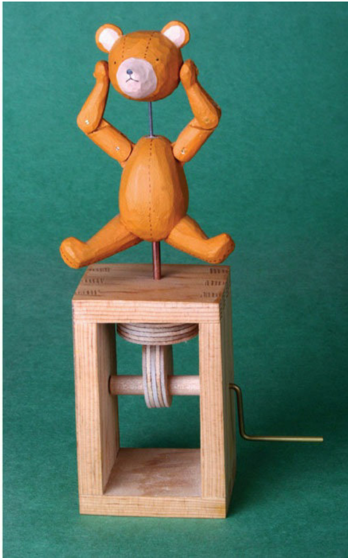
Kasuaki Harada's Teddy Bear , operated with a single eccentric cam.
