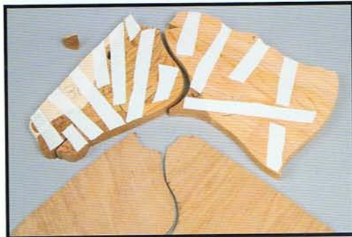
Photo 3.13. Use double-sided carpet tape to hold the parts in place.
