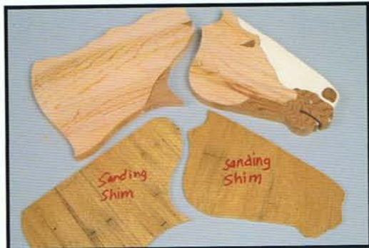
Photo 3.12. Use sanding shims to help sand a consistent contour.
