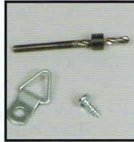
Photo 1.27. We use a mirror hanger instead of a saw tooth hanger because it is strong, reliable, and adjustable.
