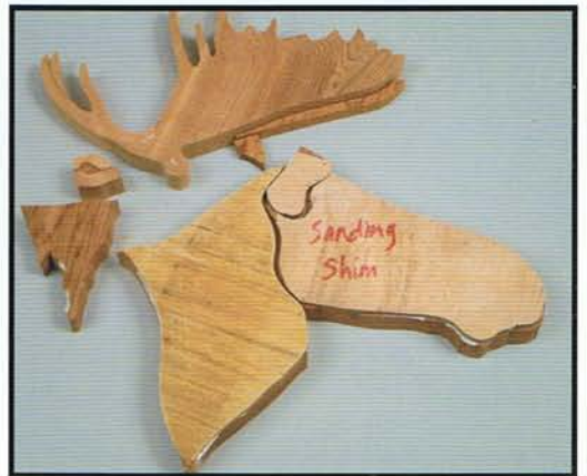
Photo 4.5. Line up the shims to enable you to sand the sections side by side.
