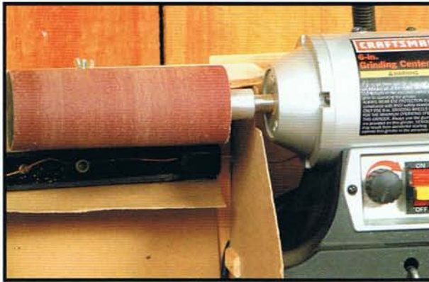
Photo 1.16. A soft sander like the Flex Drum Sander DS-I will make it easier to get the soft contours.
