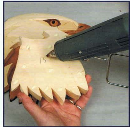
Photo 2.39. Use a combination of hot glue and yellow wood glue. The hot glue works like a clamp as the yellow glue dries.
