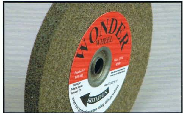
Photo 1.17. The Wonder Wheel is flat on the edge when it comes from the factory. For most texturing, it is better to make the flat edge into a V shape.
