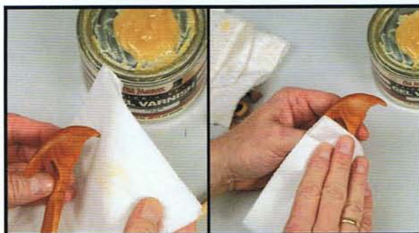
Photo 1.25. Use folded paper towels to wipe off the excess gel and to buff the pieces.
