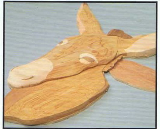
Photo 5.4. Taper the neck toward the head, and then rough in the head. Use some scrap plywood to raise the mane to the same thickness as the parts on the sanding shims.
