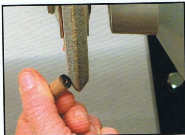
Photo 1.19. The wheel works great for eyes made from dowels or pieces of wood. Going over the surface of the wood will burnish and darken the wood.
