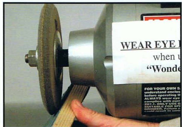
Photo 1.18. To make the flat edge into a V shape, we staple a piece of coarse sandpaper to a flat piece of wood. Sand a 45-degree angle on both sides.
