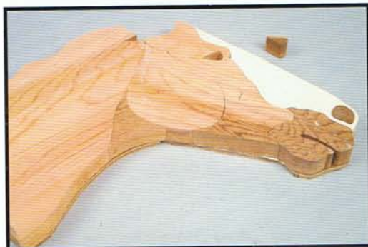
Photo 3.15. The taped sections should line up together to make it easier to match them up while sanding.
