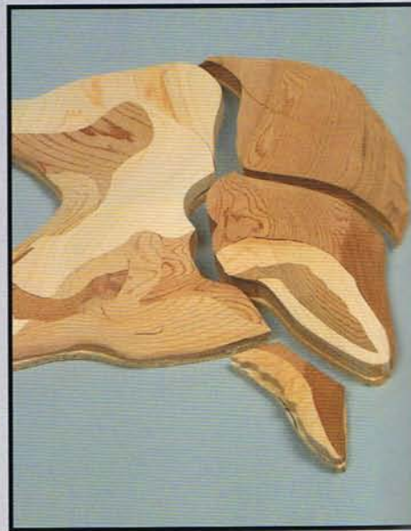
Photo 7.3. Note the sections taped to the sanding shims. Rough in all of the parts while they are taped to the sanding shims. This will give your project a nice, consistent shape.
