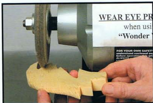
Photo 2.29. A tool called the Wonder Wheel is ideal for adding texture to intarsia projects.
