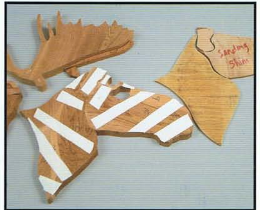
Photo 4.4. Put double-sided carpet tape on the backs of the parts.
