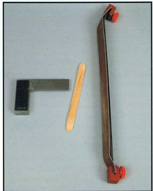
Photo 1.11. Hand tools to have nearby while you are sawing include a square (check often to make sure you are cutting square), a wooden craft stick (to help hold down a loose pattern while sawing), and a flat Detail Sander (to remove the burr on the backside of the wood).
