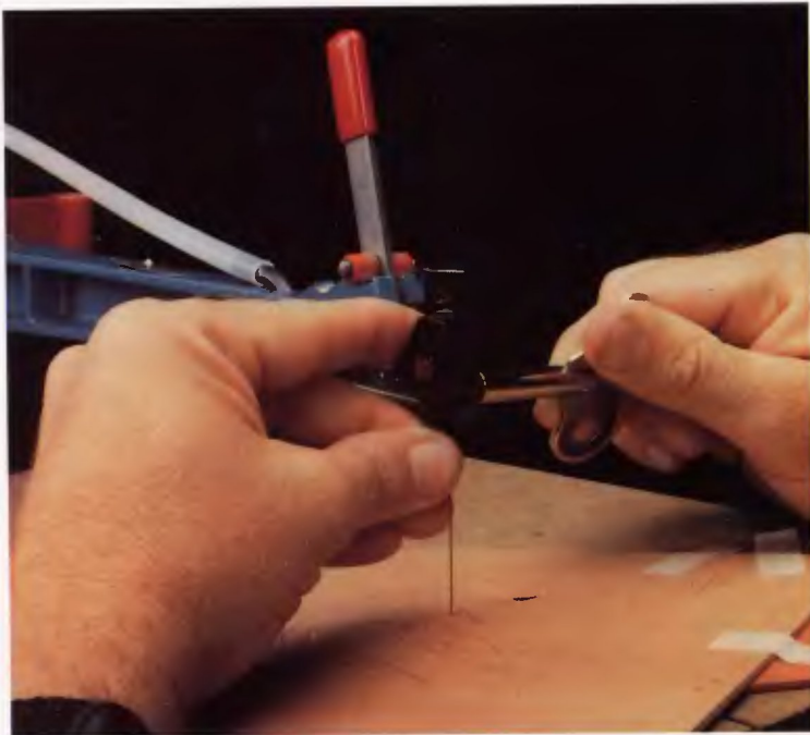
Attach the saw blade to the blade clamp and tension the blade.
