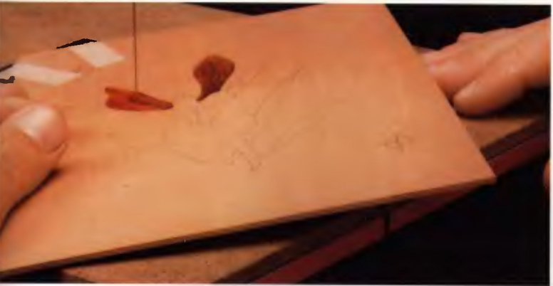
Since the angle of the drill hole is greater than the angle of the table, the workpiece won't lay flat on the saw table after threading the blade. With both hands lightly on the workpiece, touch and release the "on" switch of the saw. By causing the saw to take a couple of strokes, the blade will bring the workpiece flat on the table. If the blade breaks, remove the pieces from the blade clamps and re-thread a new blade. Begin cutting, carefully following the pattern line. When reaching a corner, carefully rotate the workpiece 180 degrees without allowing the teeth to cut the workpiece. Follow the saw kerf that was just created as you start back up the other line, merging into the drawn line. This will leave a very fine point on both ends of the insert piece.
