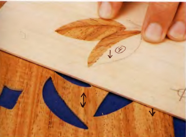
Position the background veneer over the insert veneer. Again check to make sure the arrow in the leaf section lines up with the grain of the insert veneer. Secure the two veneers with masking tape.
