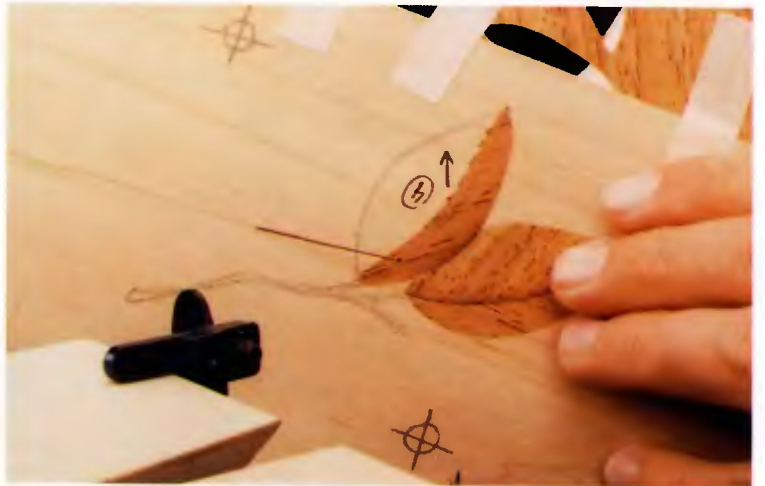
Thread the blade through the veneers. Flex the saw frame with your shoulder and fasten the blade.
