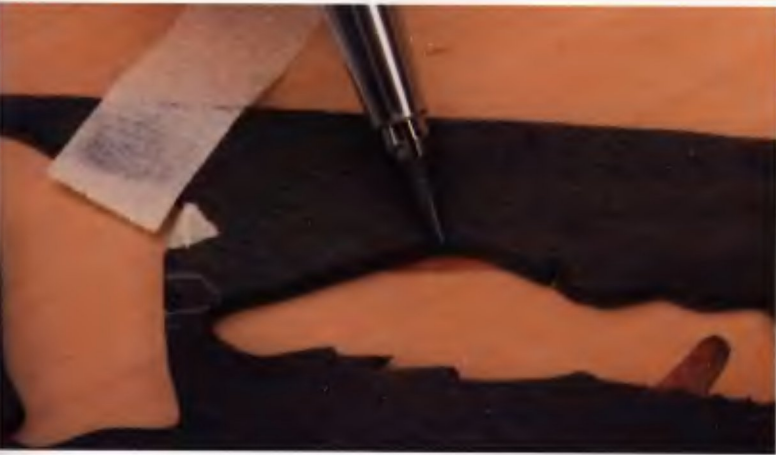
Turn the background veneer over and place the ebony in position over the flower petal. Tape in place.
