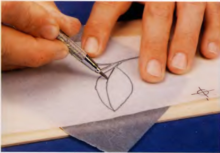
To begin working on leaf section #4, lay the pattern over the background veneer using the reference marks for positioning. Tape the pattern in place, slide graphite paper between the pattern and the background veneer, and retrace the center line of the leaf.
