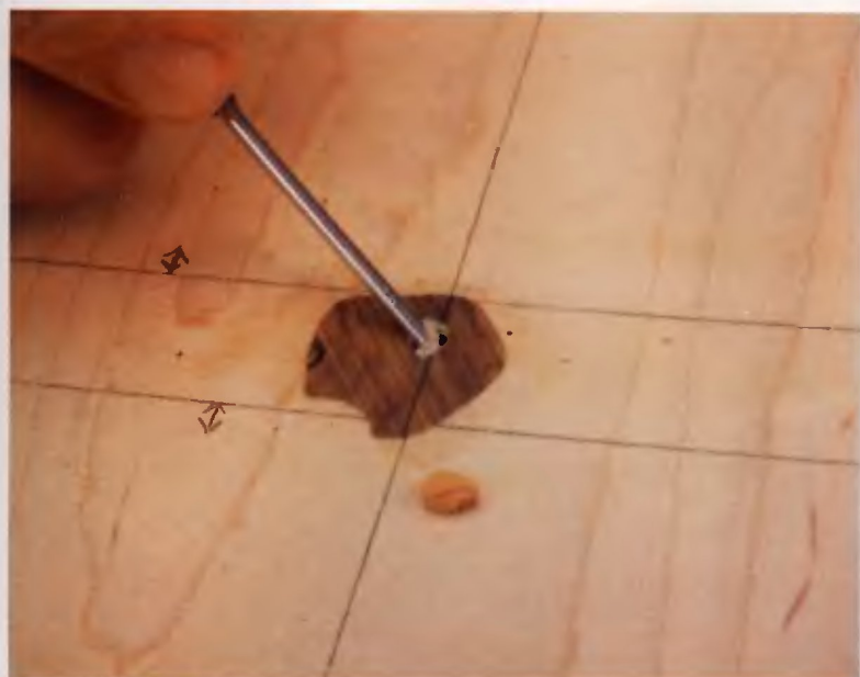
Working from the back side of the background veneer, glue the insert in place.
