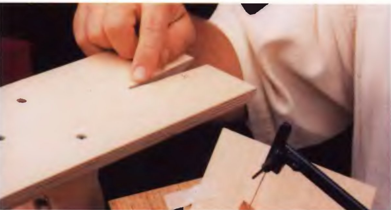
The adjustable fret saw table has been tilted to 7 degrees since I'm still using 5/64" veneers and a 2/0 saw blade. The notch in the front of the table, called the "birds-mouth", is where the sawing takes place.
