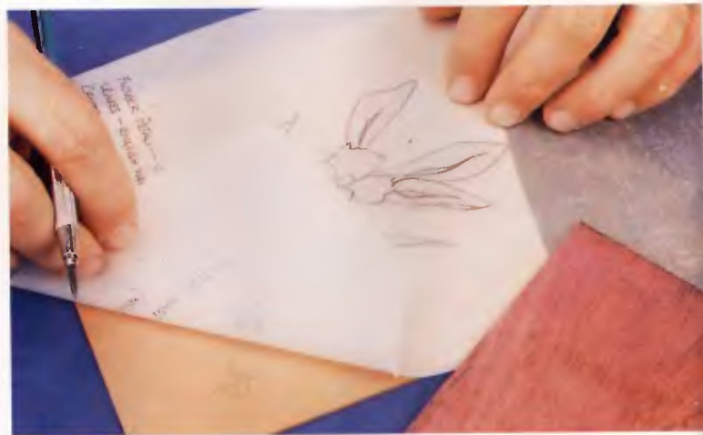
Transfer the last vein shape to the workpiece. Tape the two veneers together. Pierce, turn the workpiece over and countersink the hole. Cut out the insert, carefully working your way through the turns.
