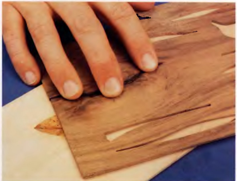
Be sure to completely cover the drilled locator holes, being sure the grain direction of the insert veneer is running in the direction of the branch. Secure with masking tape.
