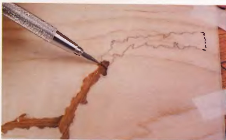
The workpiece ready to be drilled and cut. Here I'm pointing to the area that will overlap the previous section of the branch. After completing the cut, shade the bottom edge of the insert piece to complete the branch. Shading the concave edge of this piece is difficult in sawn veneers. It helps to lean the insert piece slightly face down into the sand.
