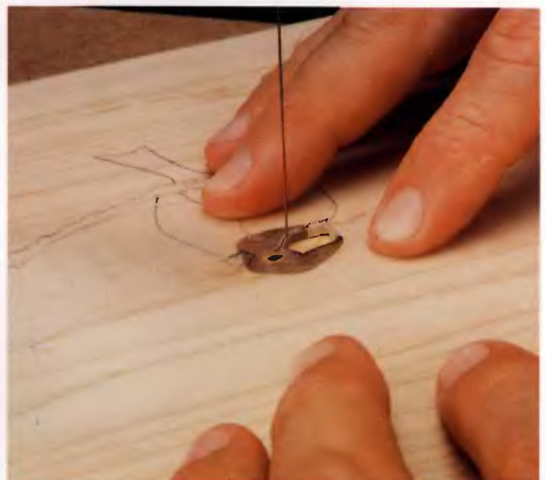
Cutting with a window in the background veneer is no different than other cuts. Keep cutting along the line as if the window is not there.
