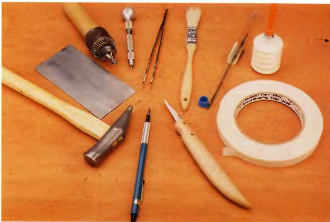
Tools and supplies needed for marquetry. From lower left, and clockwise: small hammer with slightly convex head, cabinet scraper, small countersink, pin vise with tiny drill bit (#68 drill bit), long-handle tweezers, small brush, fret saw blades (jeweler's blades, size 2/0), small glue bottle, 1/2" masking tape, bench knife, mechanical pencil.
