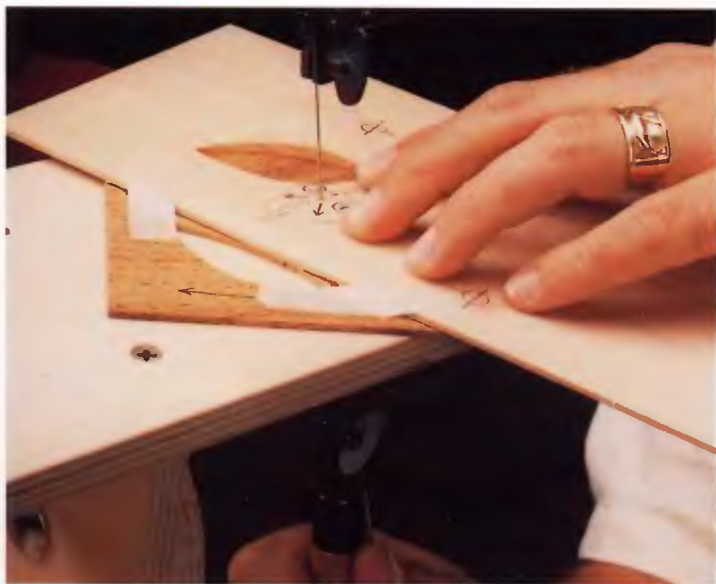
The workpiece and saw are in position to cut. My left hand keeps downward pressure on the workpiece while rotating the workpiece into the teeth of the blade. Because the saw blade's teeth are facing away from you, the rotation of the workpiece is opposite (counter-clockwise) of the rotation used on the scroll saw. With the table tilted down to the left, the waste piece in the background veneer is uphill or to the right of the saw blade.
