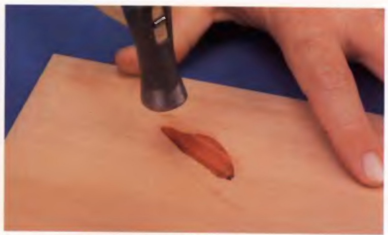
Lightly tap with a small hammer for a snug fit.
