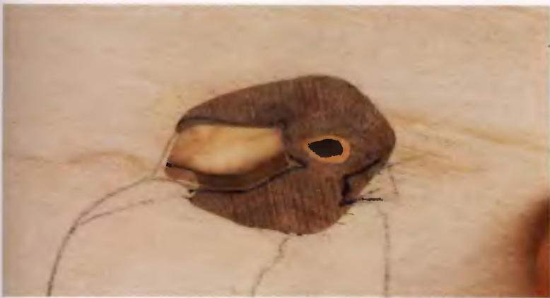
Position the opening in the background veneer over the desired area of the olive veneer. Once satisfied, tape the veneers together.
