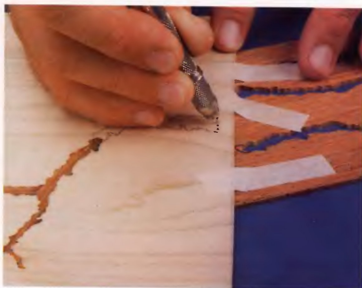
The last section to complete the branch will be let-in. Once again, the dotted line at the end of the branch will be the end of the design while staying within the background veneer. The reason to stay inside the background veneer and leaving a margin is that it maintains stability of the workpiece. I purposely made the background veneer slightly larger than the final size to allow room for this.
