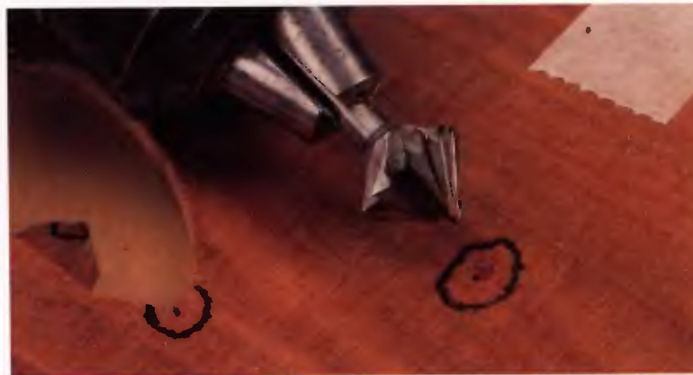
Pierce at the dotted line, turn the workpiece over and countersink the hole.
