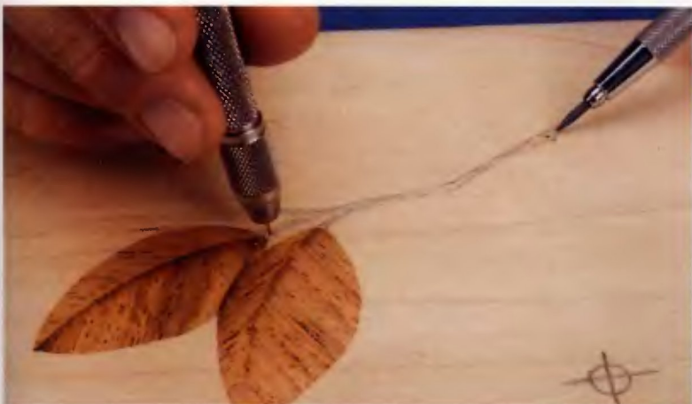
To aid in placing the background veneer on the new insert veneer, I drilled a hole through the background veneer at both ends of the length of the branch. These holes serve as locators when positioning one veneer over another to ensure the desired grain direction and to prevent placement of the veneer outside of the pattern. Because the holes are drilled within the pattern lines they will be cut away when the insert veneer is cut or "let-in" into the background veneer.
