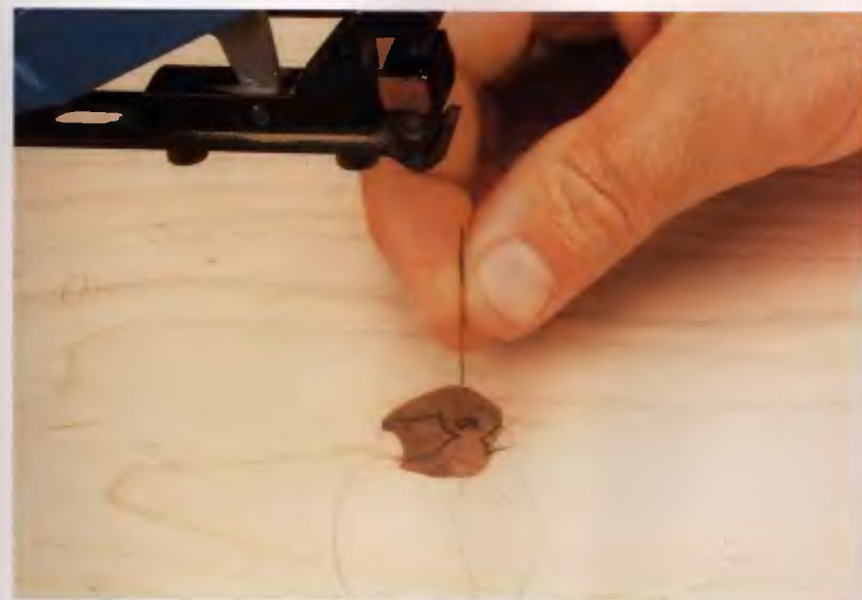
Pierce the veneers, turn the workpiece over and countersink the hole. Make the necessary preparations for cutting.
