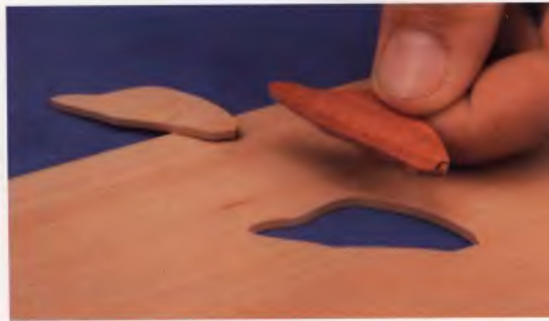
The first insert piece, cut and ready to test fit.
