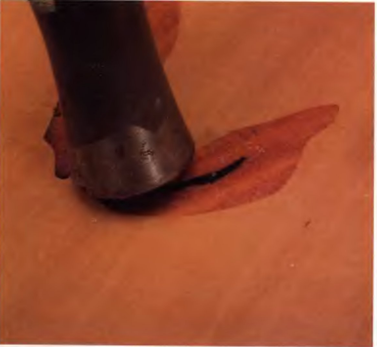
Tap lightly and wipe off excess glue.
