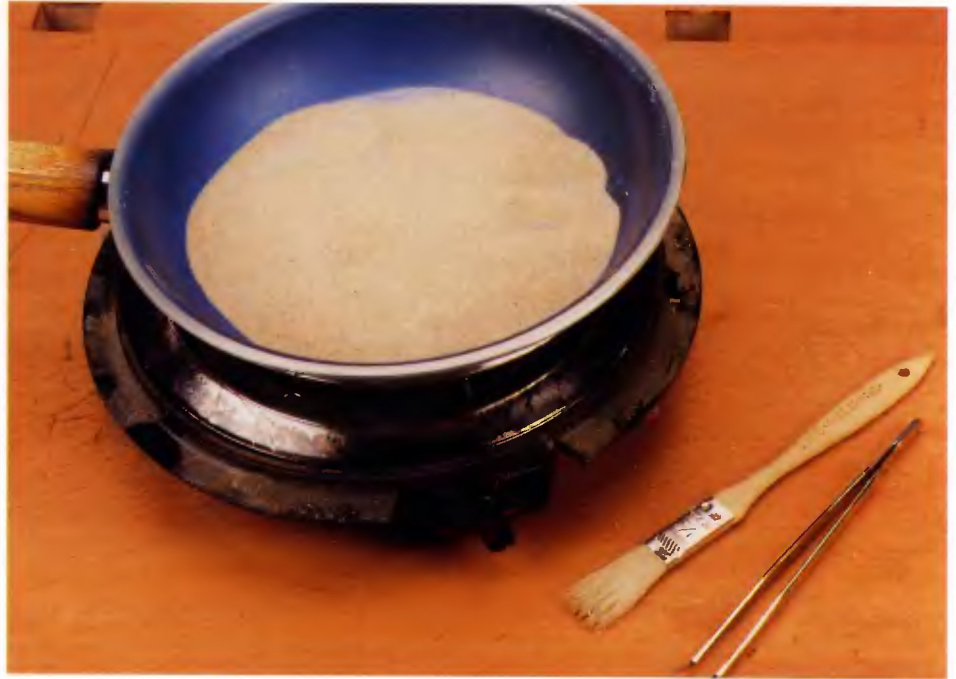
Equipment for sand shading: small hotplate and pan, fine sand (playground sand), small brush, long-handle tweezers.
