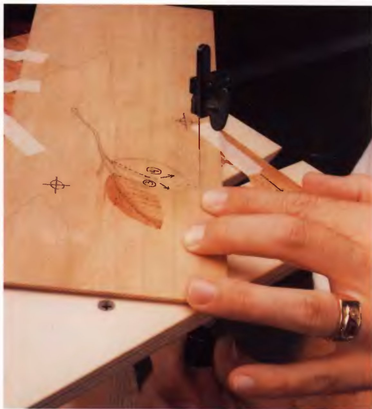
Begin sawing along the line. My right hand operates the saw vertically. To steady the sawing motion, I rest my elbow against my leg. This helps assure that the saw stroke is consistently vertical. Make every effort to saw within the birds-mouth, pausing occasionally to check the saw blade's position. With my left hand manipulating the workpiece, I saw along the dotted line towards the corner.
