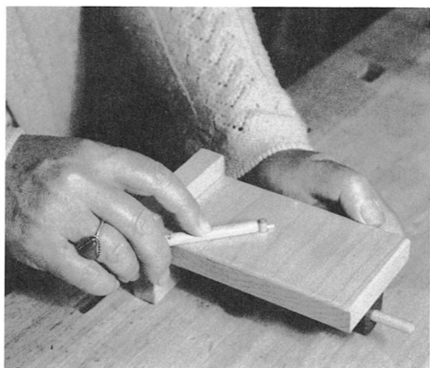
Illus. 2-52. Using the assembly tool to insert the small pin in the Scotch Yoke axle.
