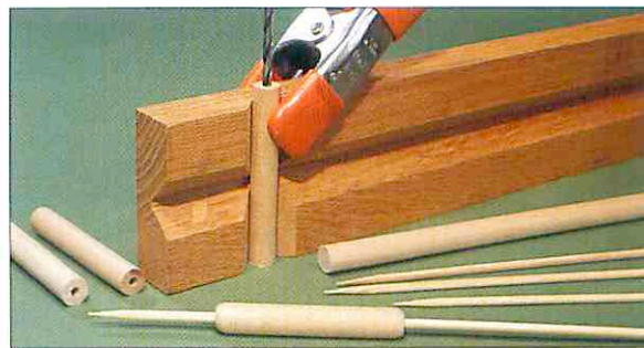
Fig. 3-18: A simple V-block, when set up on a drill press as shown, makes perfectly centered and straight holes into the dowel ends.
