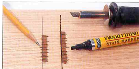
Fig. 3-11: Marker ink bleeding across the pencil line at left but not the burned line at right.
