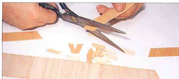
Fig. 5.11-7: Cutting the individual shingles.
