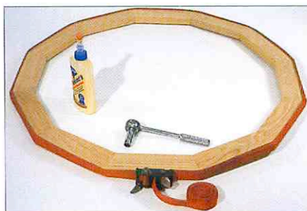
Fig. 1-7: A test assembly with a band clamp.
