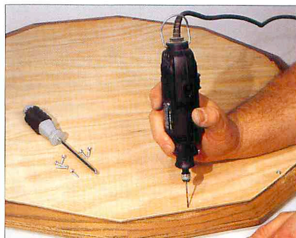
Fig. 2-35: Drilled pilot holes.
