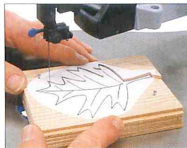
Fig. 3-7: Sawing tacked layers.
