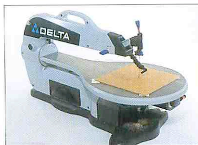
Fig. 3-6: Auxiliary hardboard table with a small blade-entry hole is held in place with double-faced tape. This setup is ideal for sawing small parts and supporting fragile pieces.
