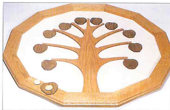
Fig. 4.4-7: Layer 1 in \frac{1}{4} " relief. Also shown on the frame are \frac{1}{8} "-thick shims.
