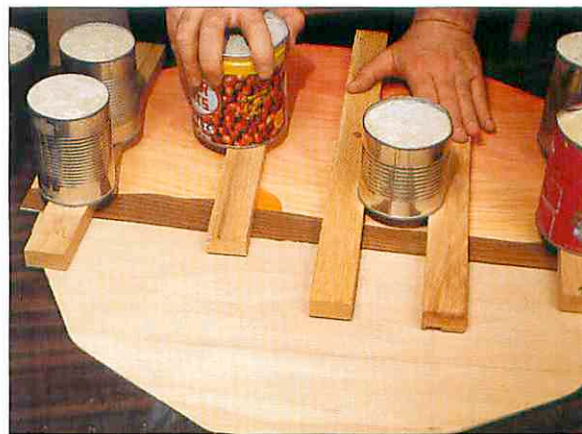
Fig. 2-28: Flat strips of wood and cans containing sand or concrete provide clamping pressure.
