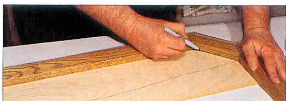
Fig. 2-33: Fitting the layered pieces against the inside of the frame.
