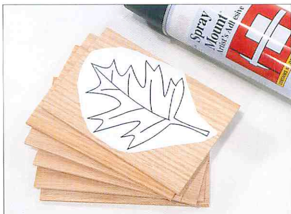
Fig. 3-5: Photocopied pattern temporarily bonded directly to wood.
