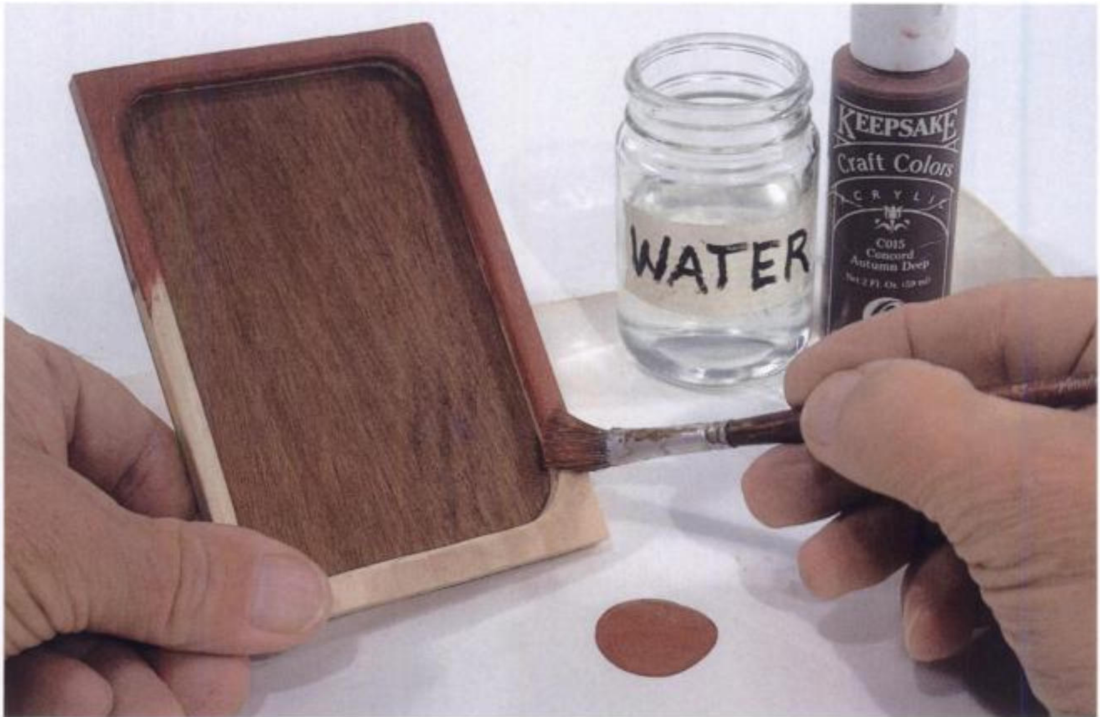
2-34. Painting the frame/border piece with acrylic craft paint. Coat all visible edges and only the rear surface of the backer.
