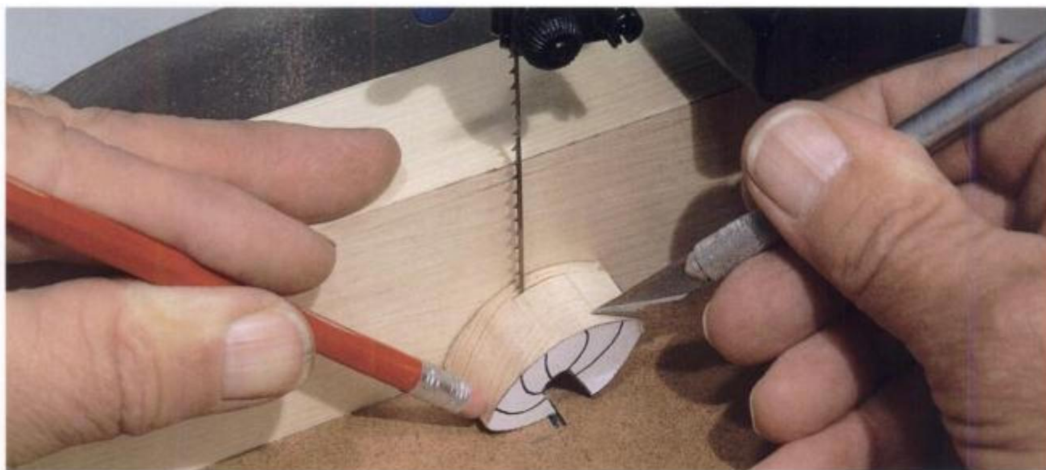
2-22. Resawing small parts using the scroll saw with a combination resawing fence and auxiliary table. Notice the use of a "thick wood" cutting blade.
