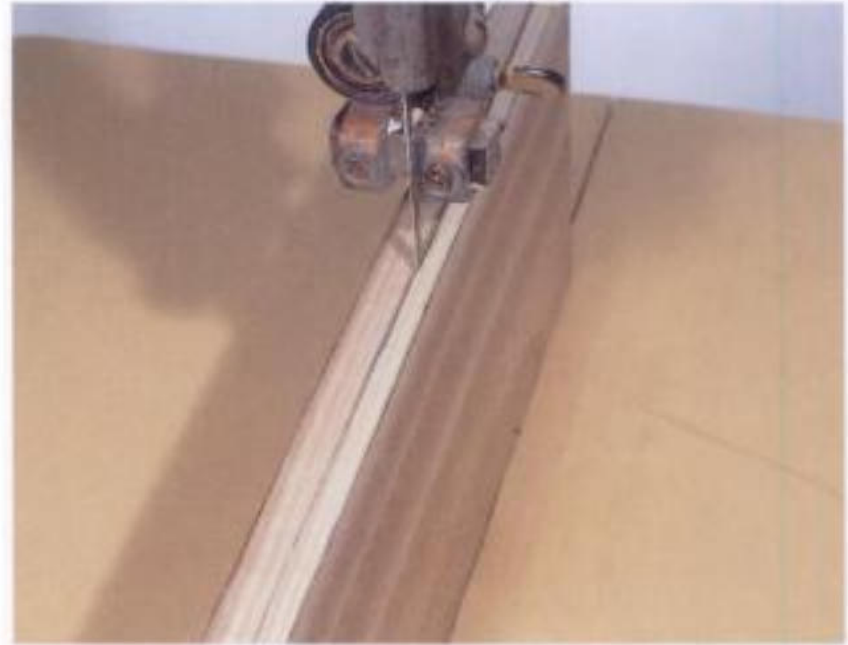
2-5. Resawing to thickness following a marked edge.
