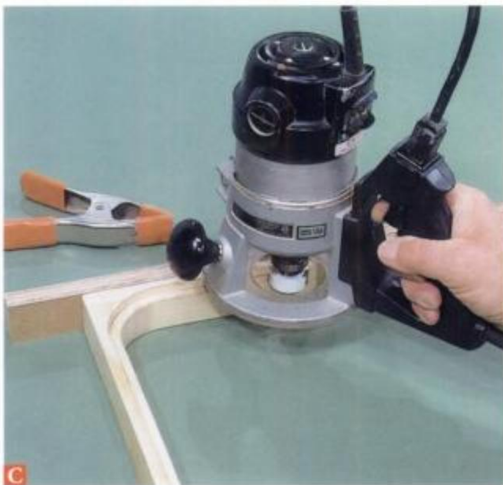
C Rabbing the rear of the frame. A strip of wood clamped to the frame provides more surface support for the router.
