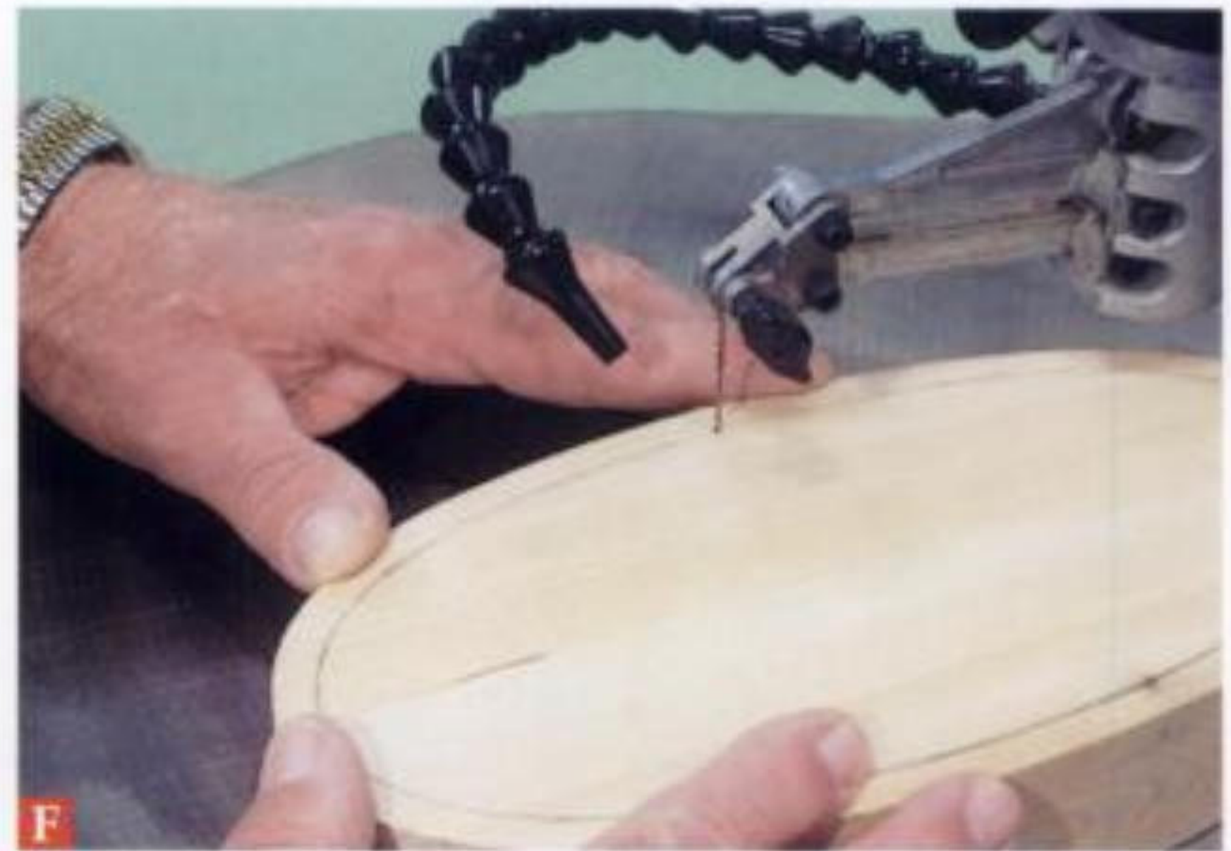
F Cutting out the box opening.
