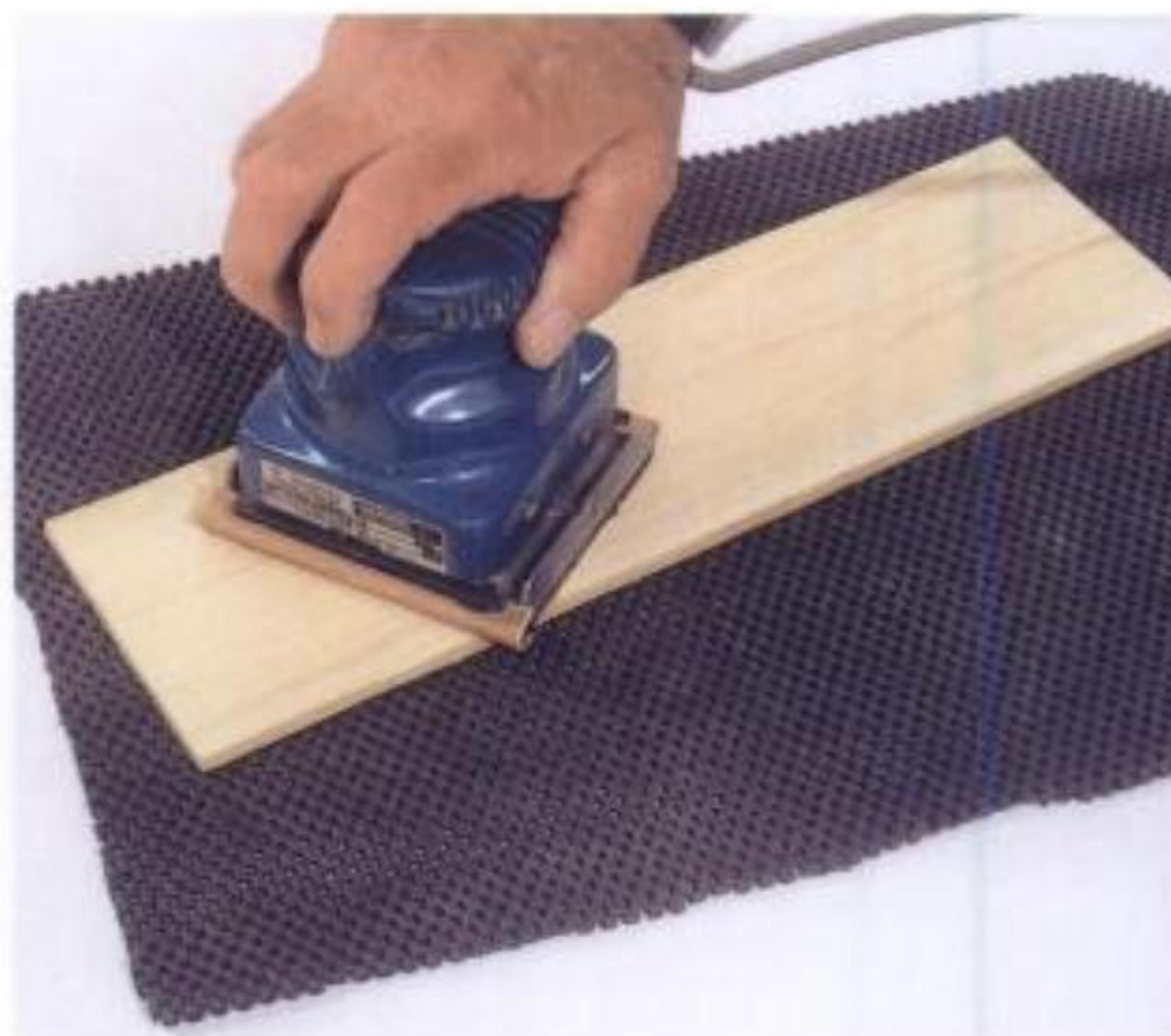
1-11. A small pad sander is used to smooth a flat board supported on a nonslip pad.
