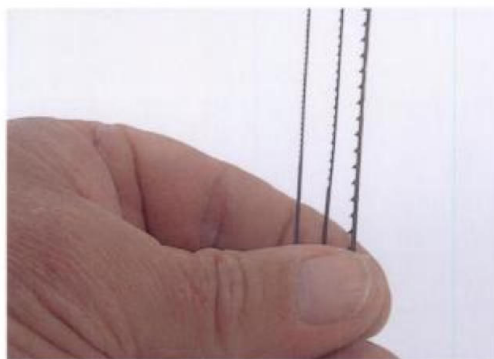
1-6. Basic blades. Left to right: No. 2 and No. 5 blades will handle most jobs; the special thick-wood blade is useful for resawing small pieces to a reduced thickness, but is not essential.
