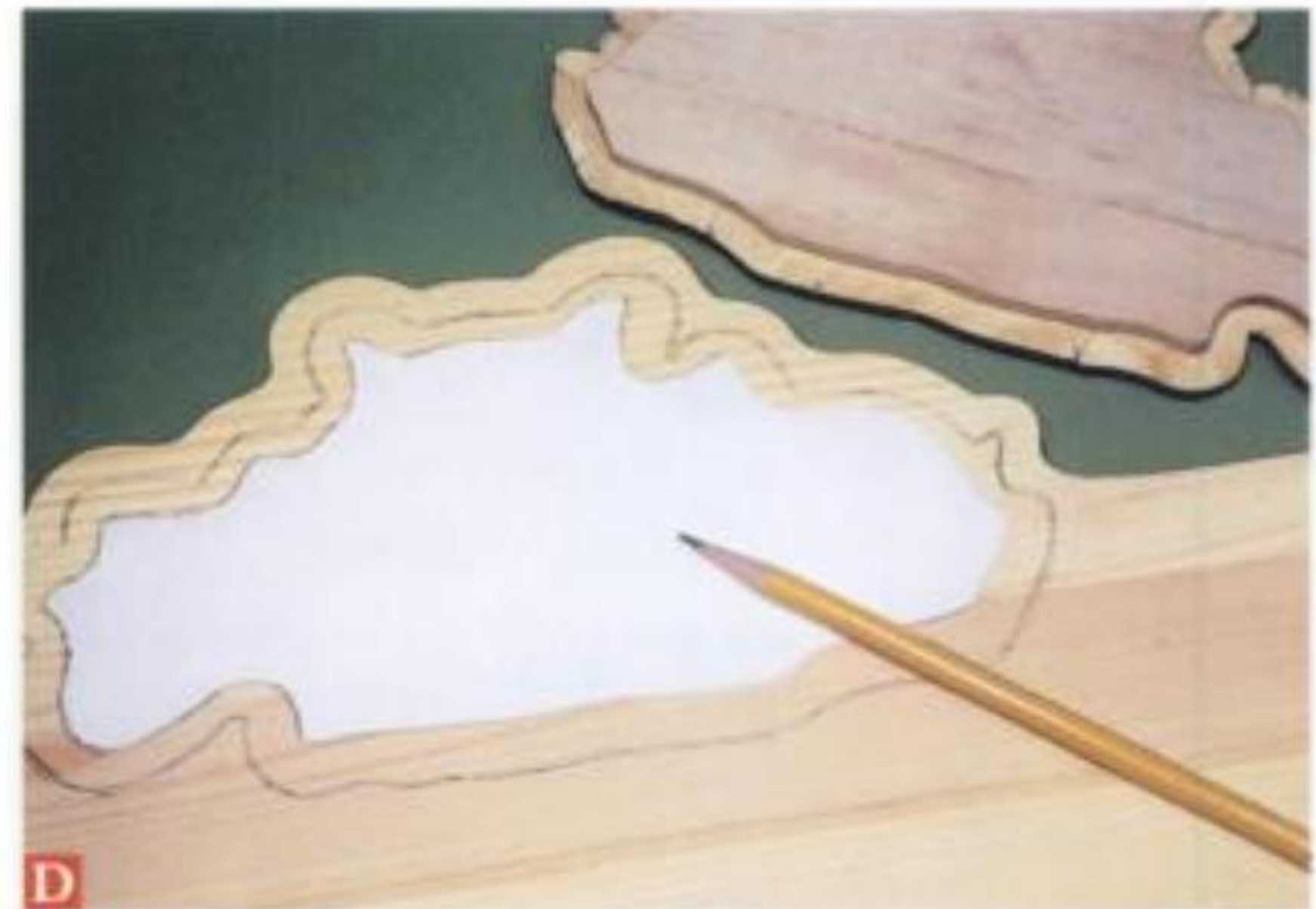
D The “rubbing” pattern for routing a recess is scissor-cut to size and then traced, as shown.
