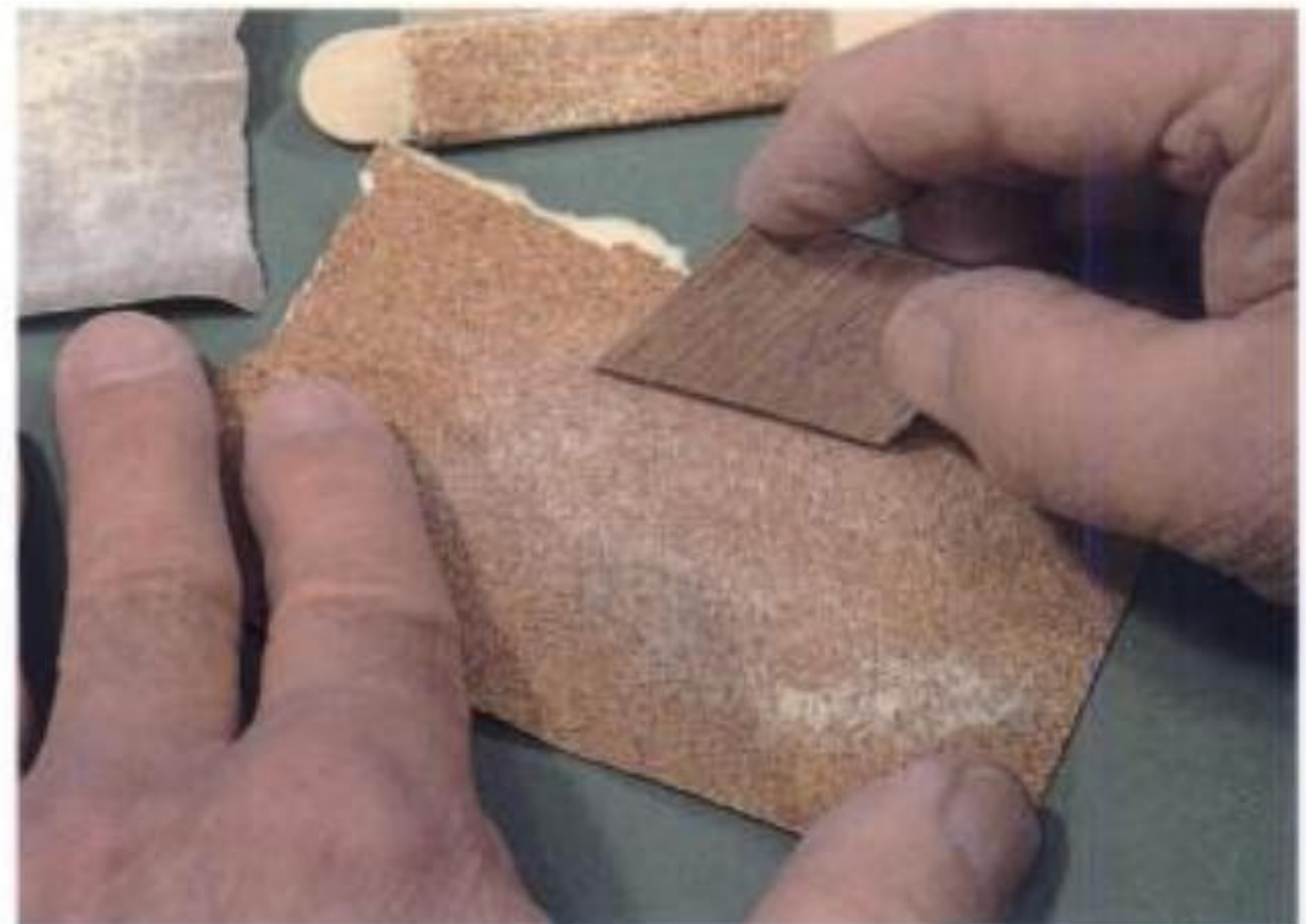
2-28. Rounding over straight edges of a workpiece with sandpaper held flat on the workbench surface.
