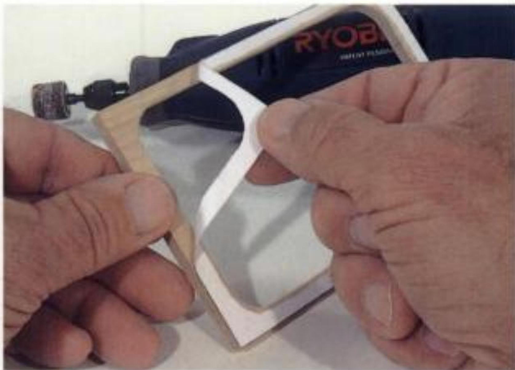
2-32. Properly applied patterns should remove easily; otherwise, use appropriate solvents to soften the adhesive.
