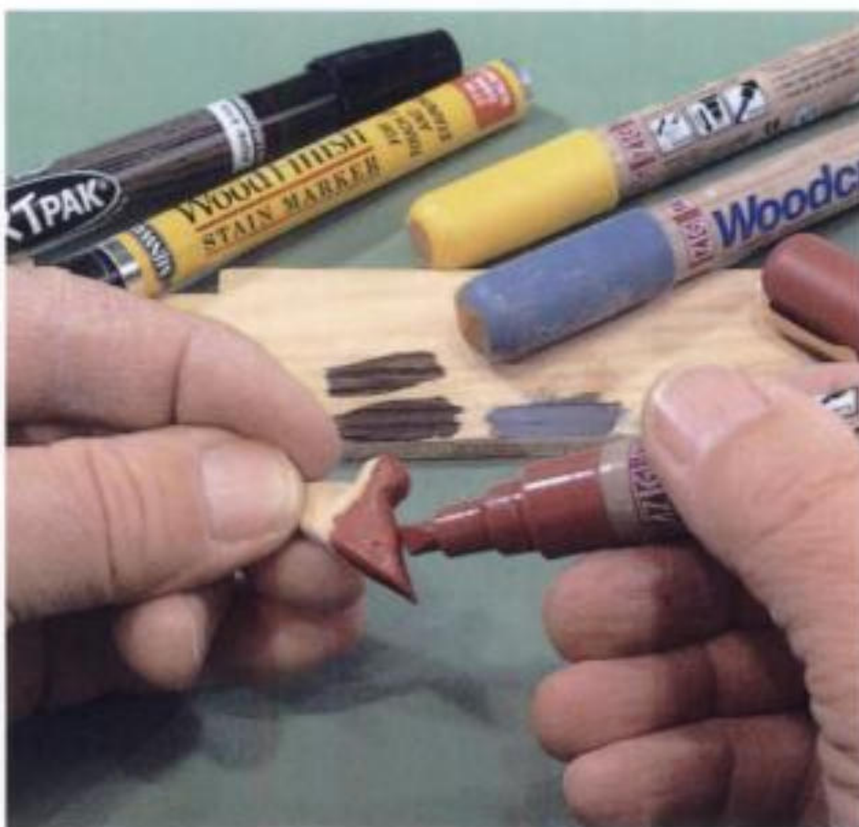
2-35. Small pieces are quickly colored using felt-tip markers.
