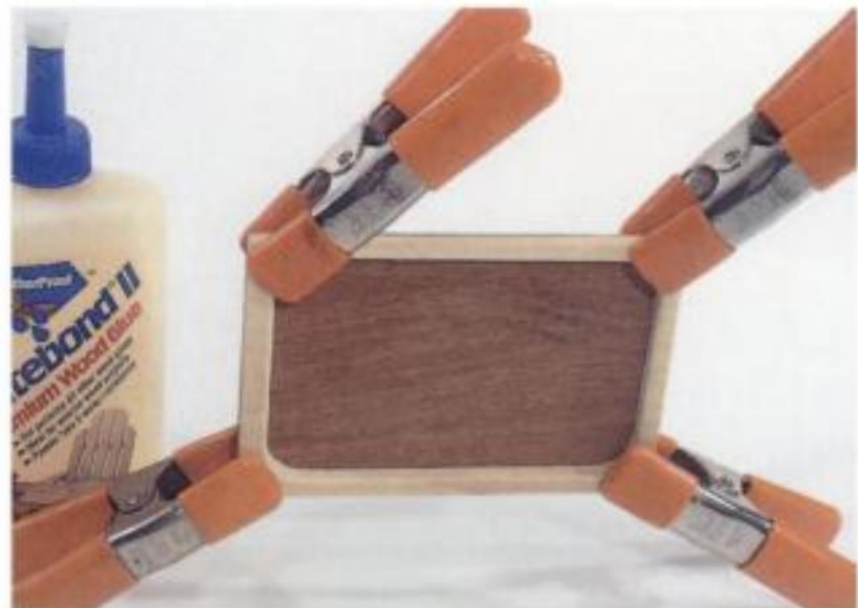
2-33. Gluing a frame to a plywood backer.
