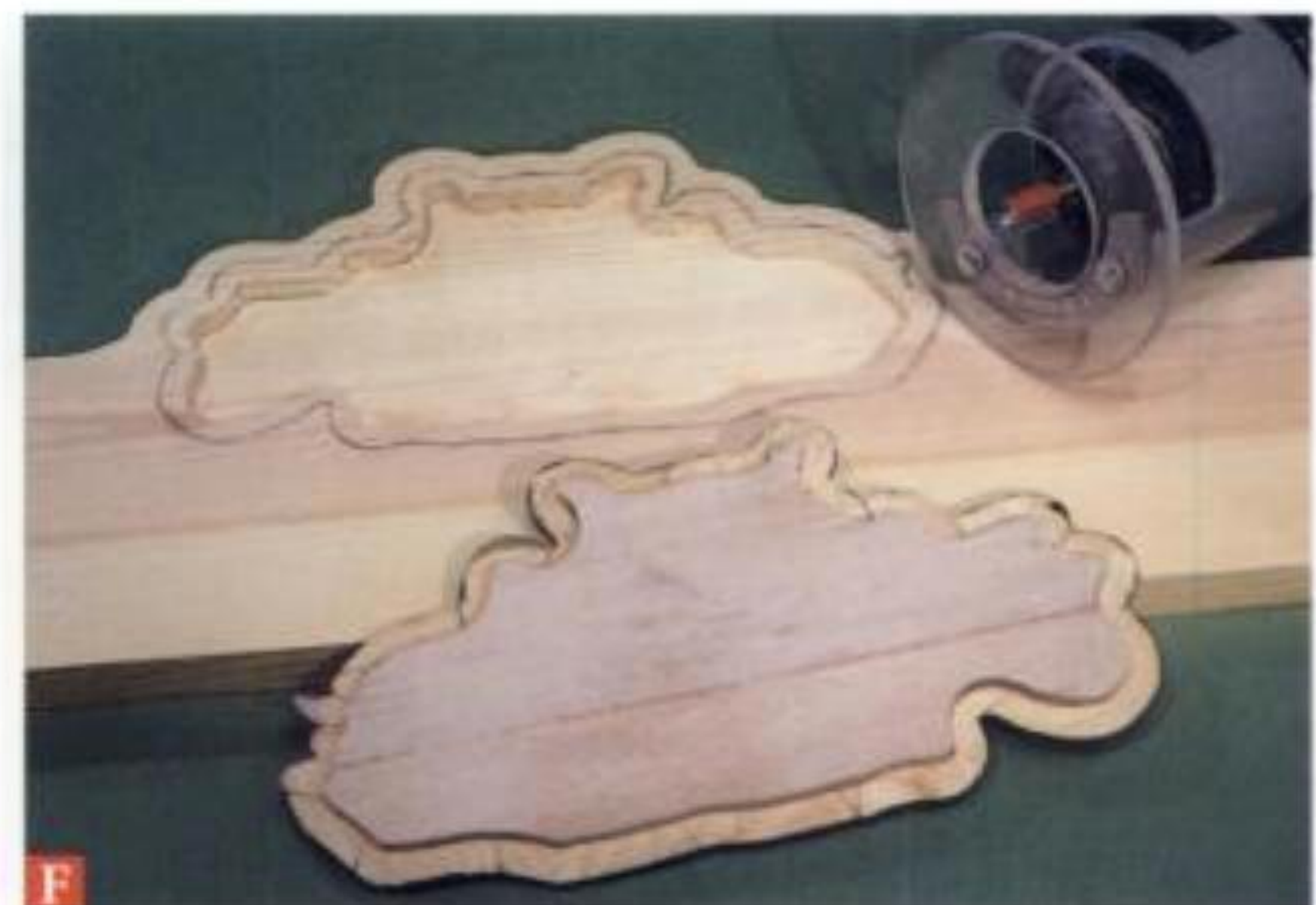
F The completed router-cut recess ready for the rabbeted intarsia piece.
