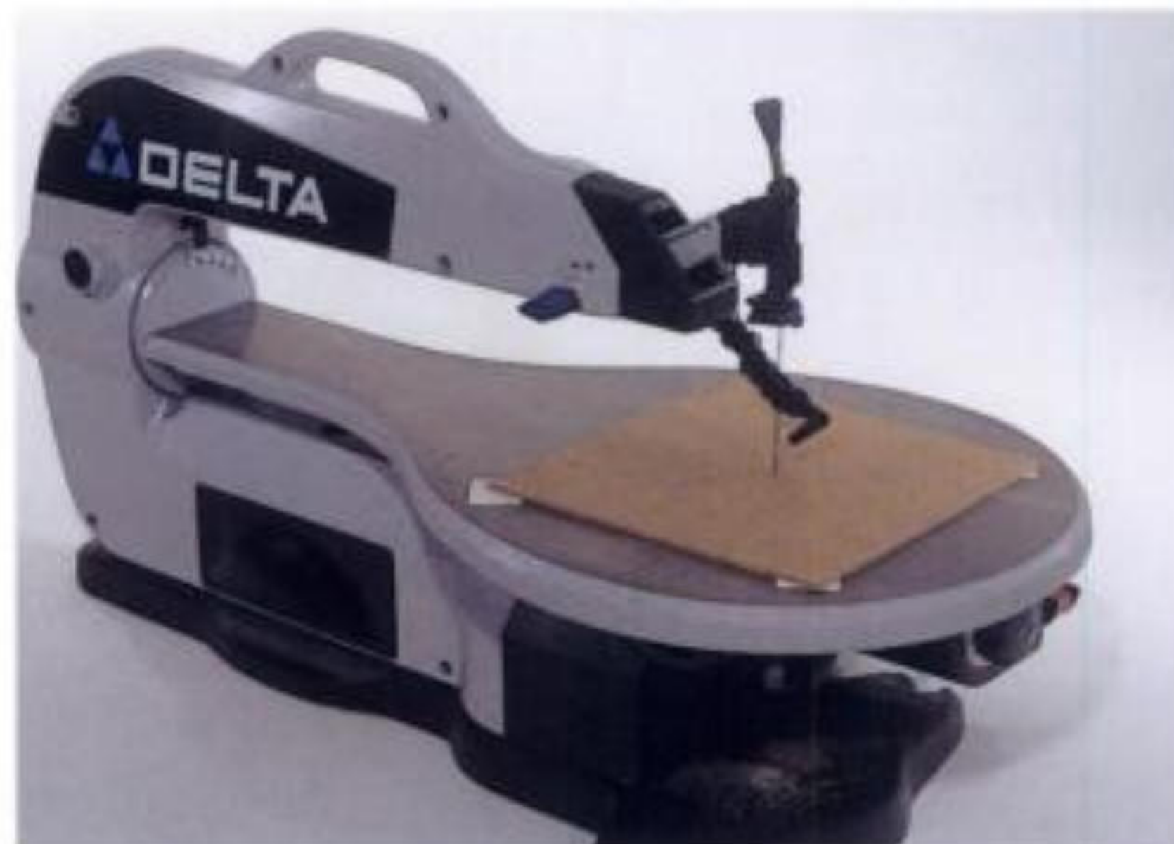
1-5. An economy-model 16-inch bench-top scroll saw with features suitable for making the projects in this book. Notice the auxiliary piece of thin hardboard held in place with double-faced tape. This provides almost zero clearance around the blade, which is necessary for sawing very small parts.
