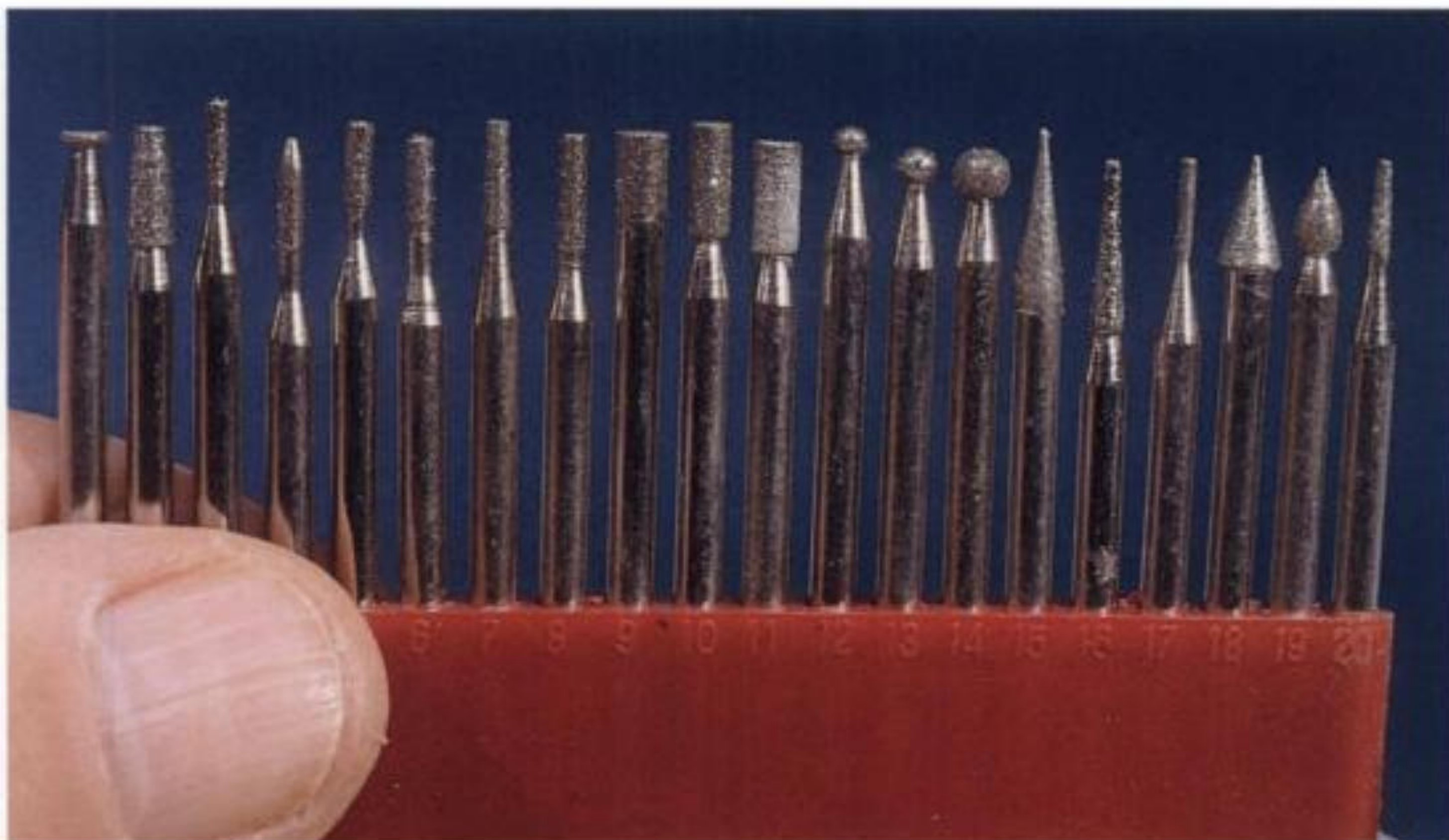
1–9. An inexpensive yet very serviceable set of 20 diamond-coated microburrs on \frac{1}{8} -inch shanks that cost less than 70 cents each.
