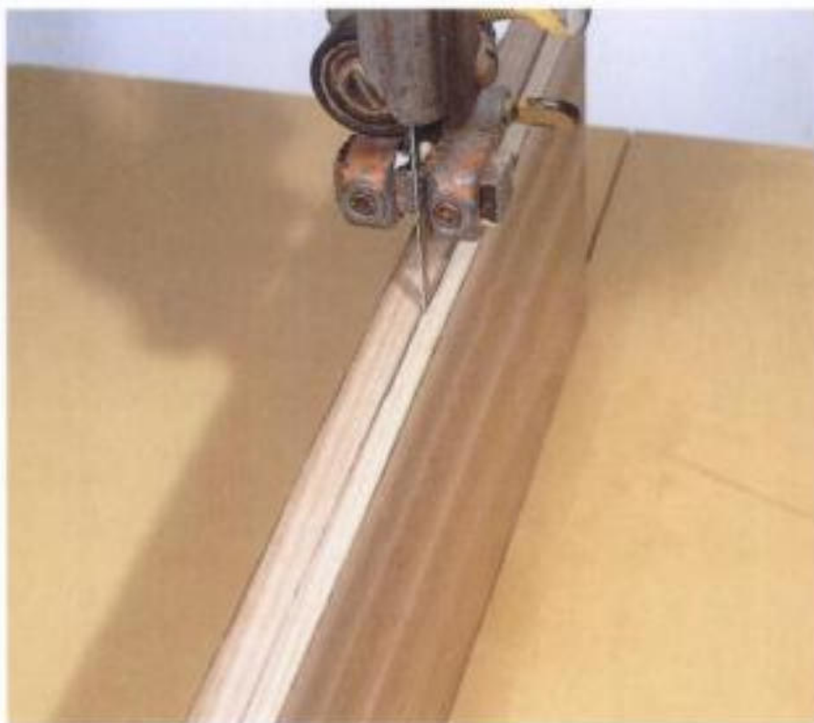
1–7. A bandsaw permits do-it-yourself resawing of solid boards into thin ones, as shown. Plywoods or MDF (medium-density fiberboard) panels of various thicknesses can be obtained for making painted projects.
