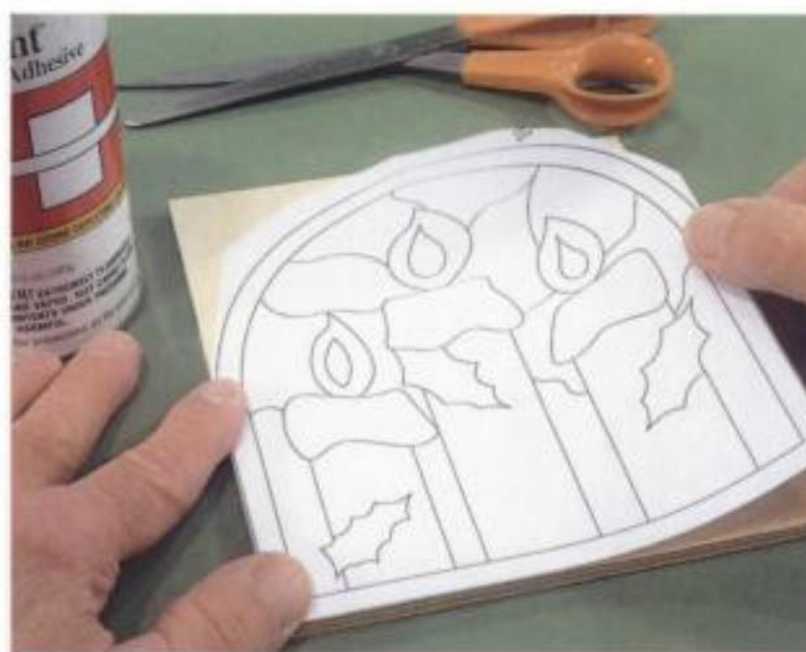
1–3. A temporary bond spray adhesive mounts a photocopied pattern directly to the workpiece for sawing. Note that the three straight edges were precut.
