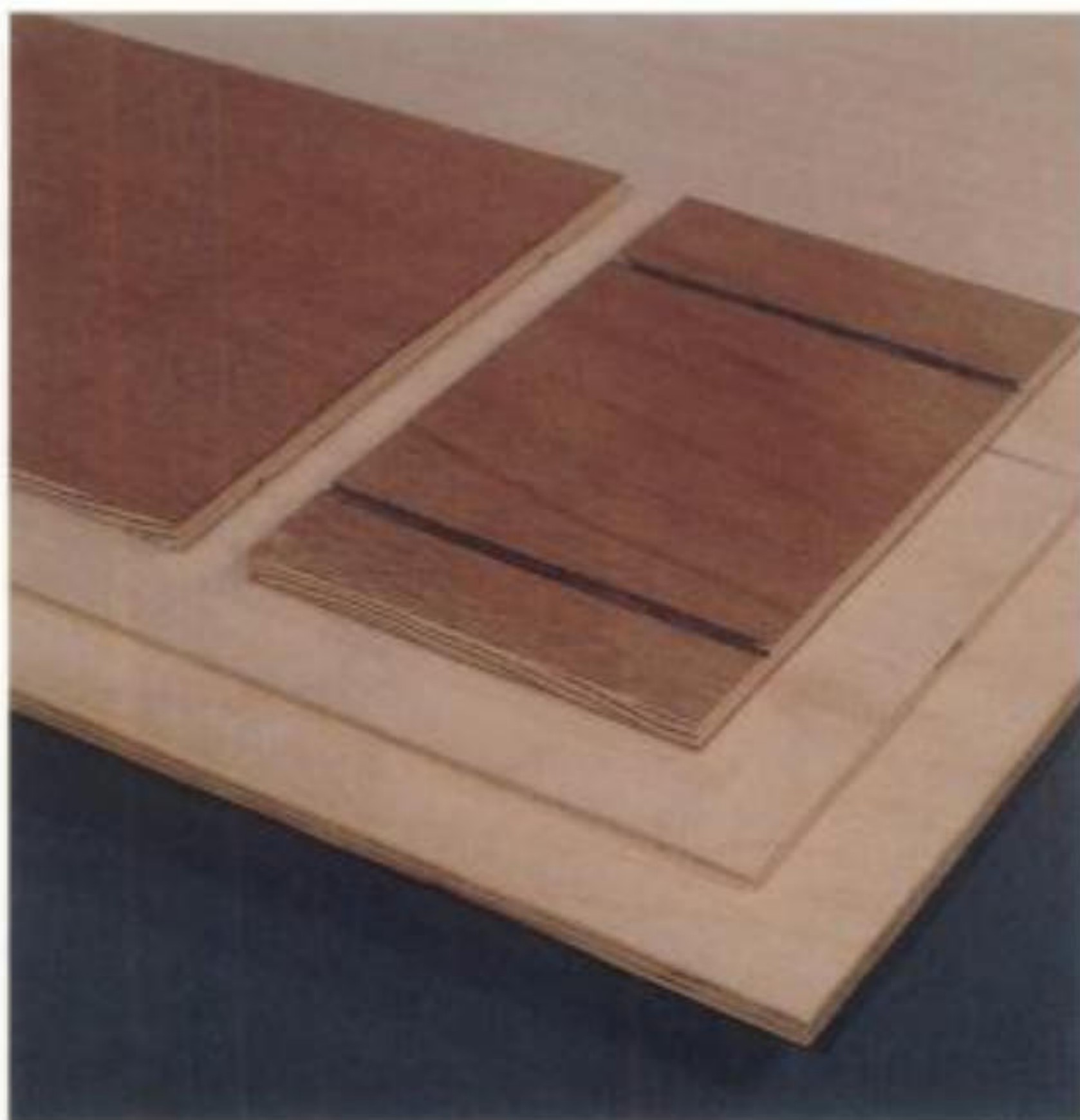
1–2. Plywood. Shown on top of 1/8- and 1/4-inch sheets of Baltic birch plywood are two pieces of recycled wall paneling: the finished face on the right and the gluable surface on the left.
