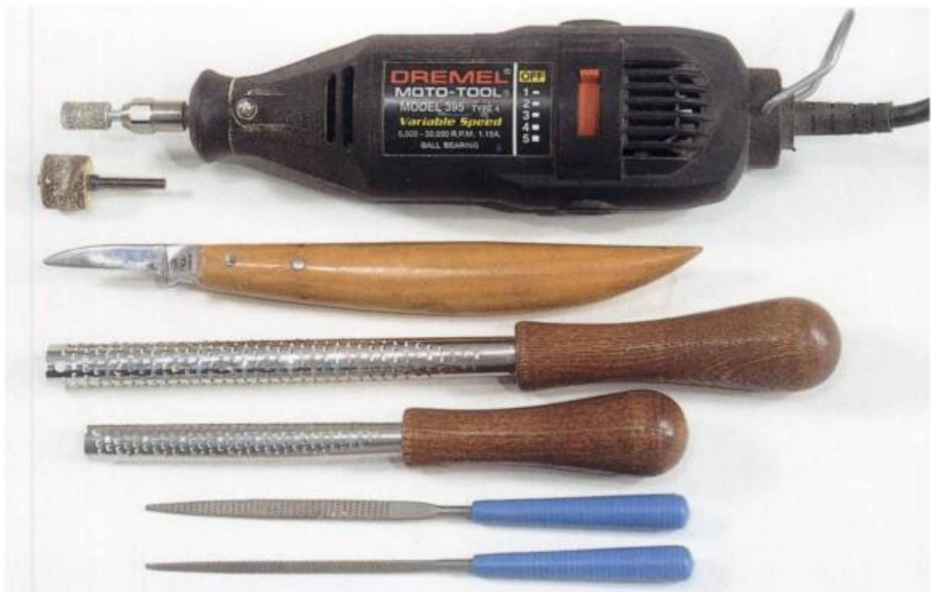
1–8. Tools for rounding over edges, shaping contours, and detailing. Shown from top to bottom: a high-speed rotary tool that carries various small cutters and sanding drums; a knife; small rasps; and files.
