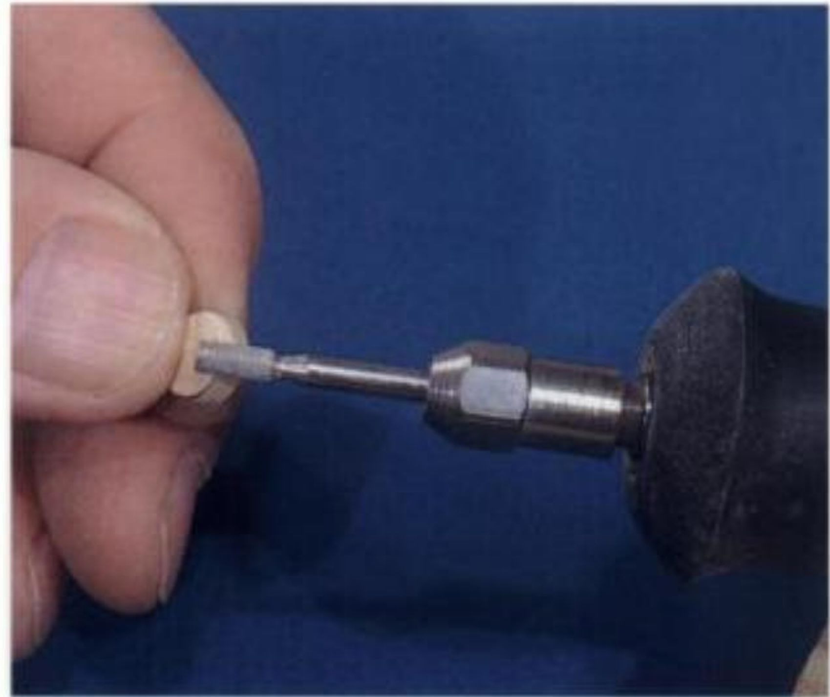
2-31. Very small pieces are safely and quickly rounded over using diamond-coated microburrs. See Illus. 1-9 on page 13.
