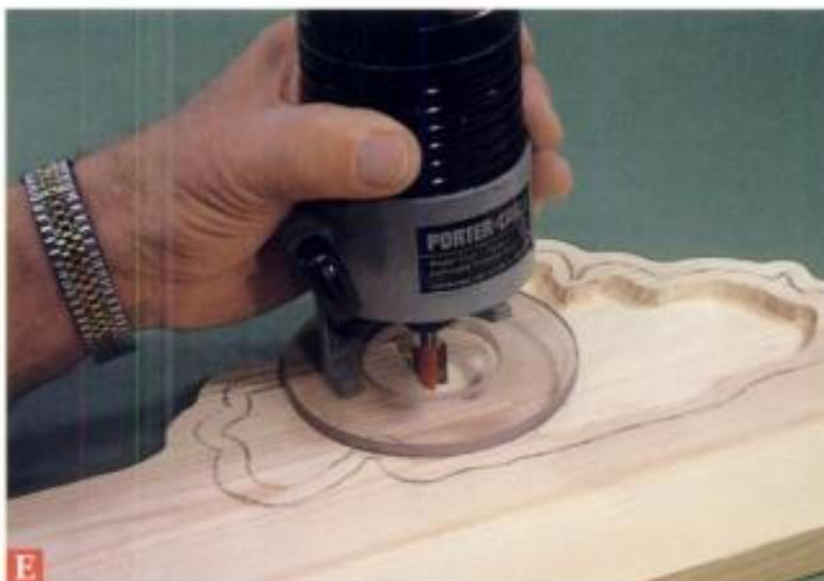
E Freehand-routing a rough-sized recess to receive the rabbeted intarsia piece.
