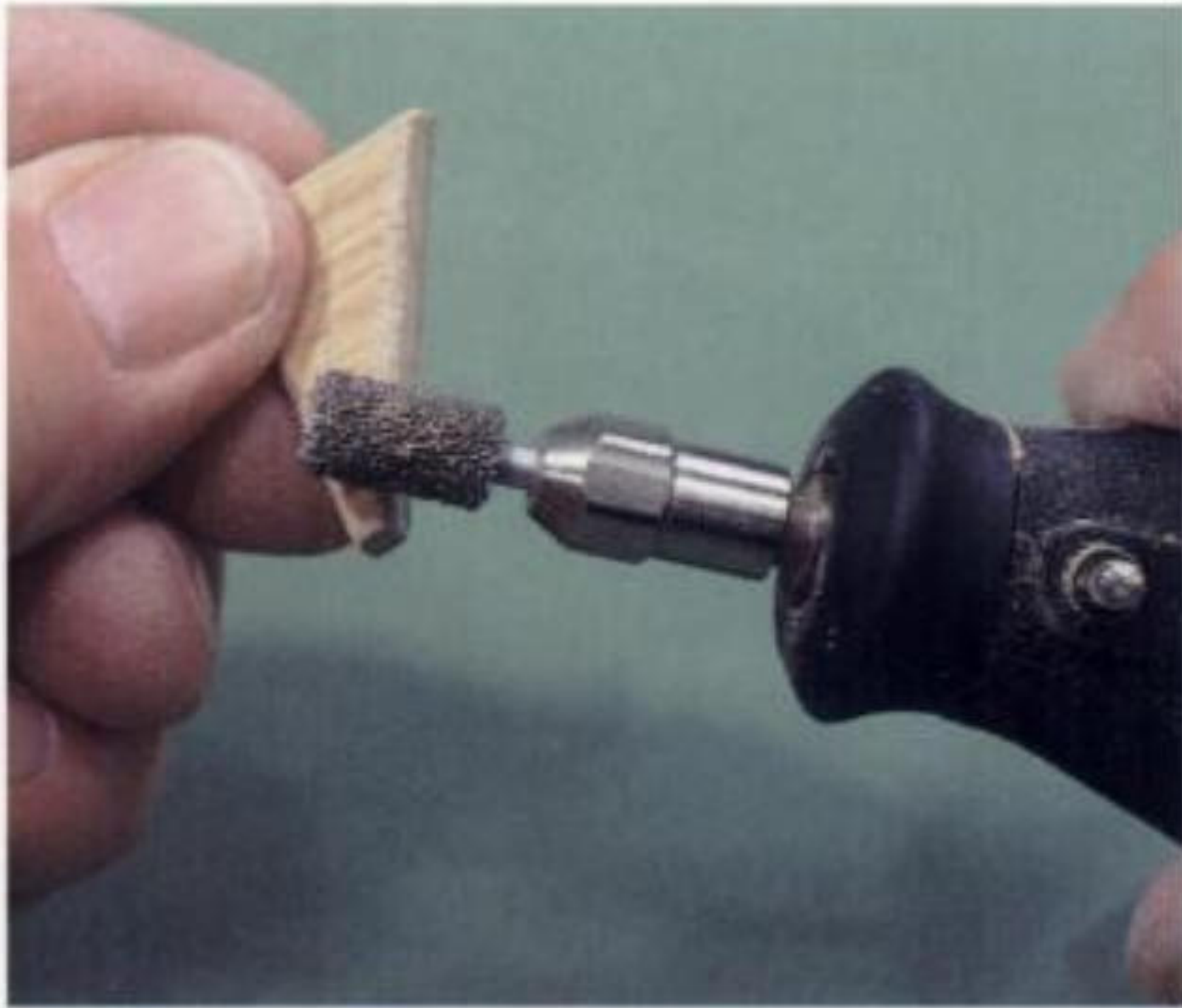
2-30. A structured carbide cutter in a rotary tool removes material quickly.
