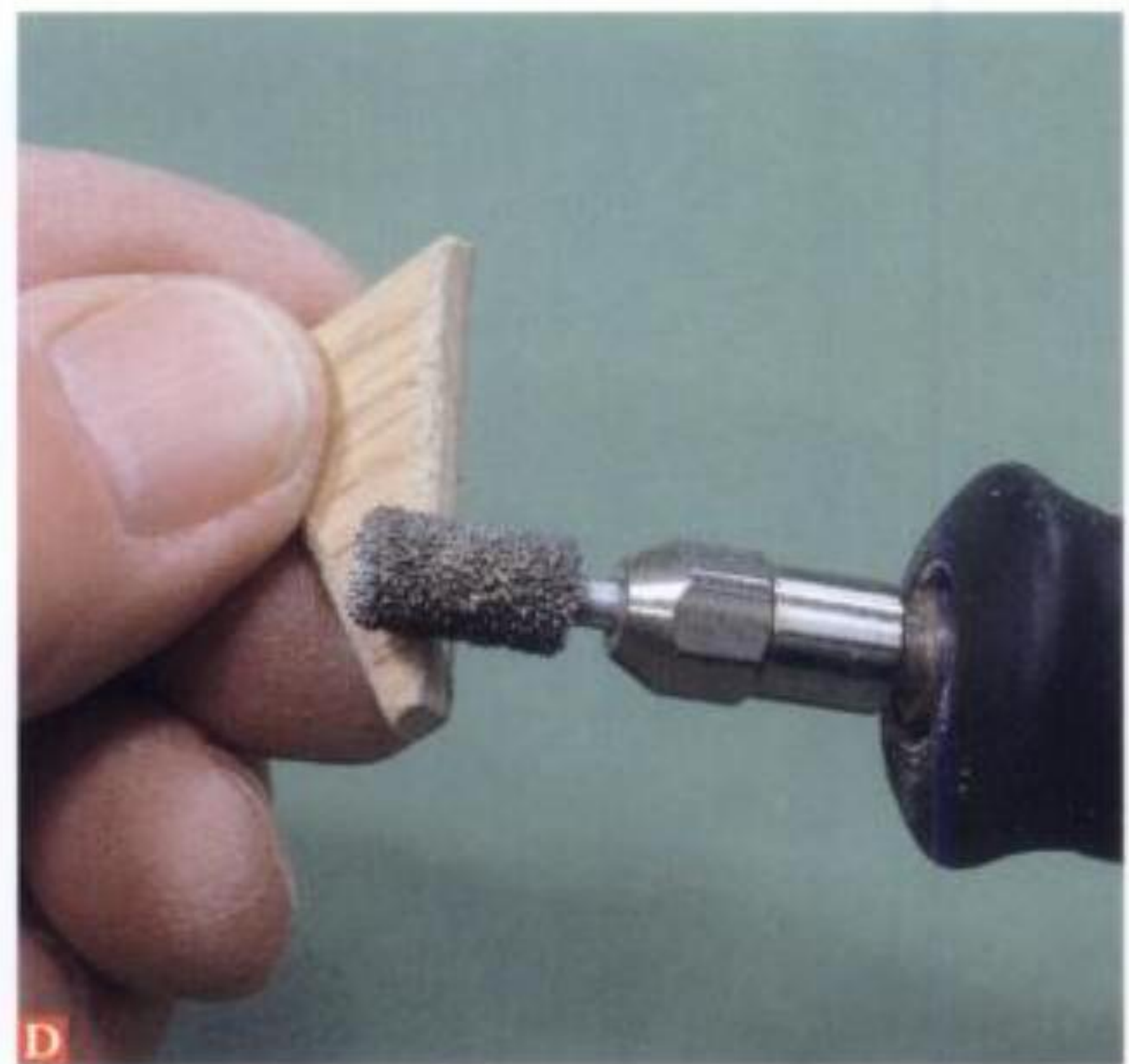
D Rounding the edges of the lighthouse segments with a rotary tool.
