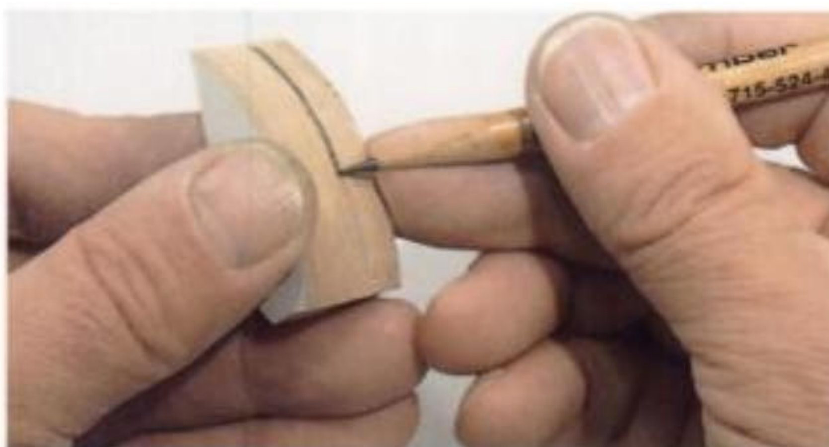
2-17. Finger-gauging a guideline for reducing the thickness of a workpiece.
