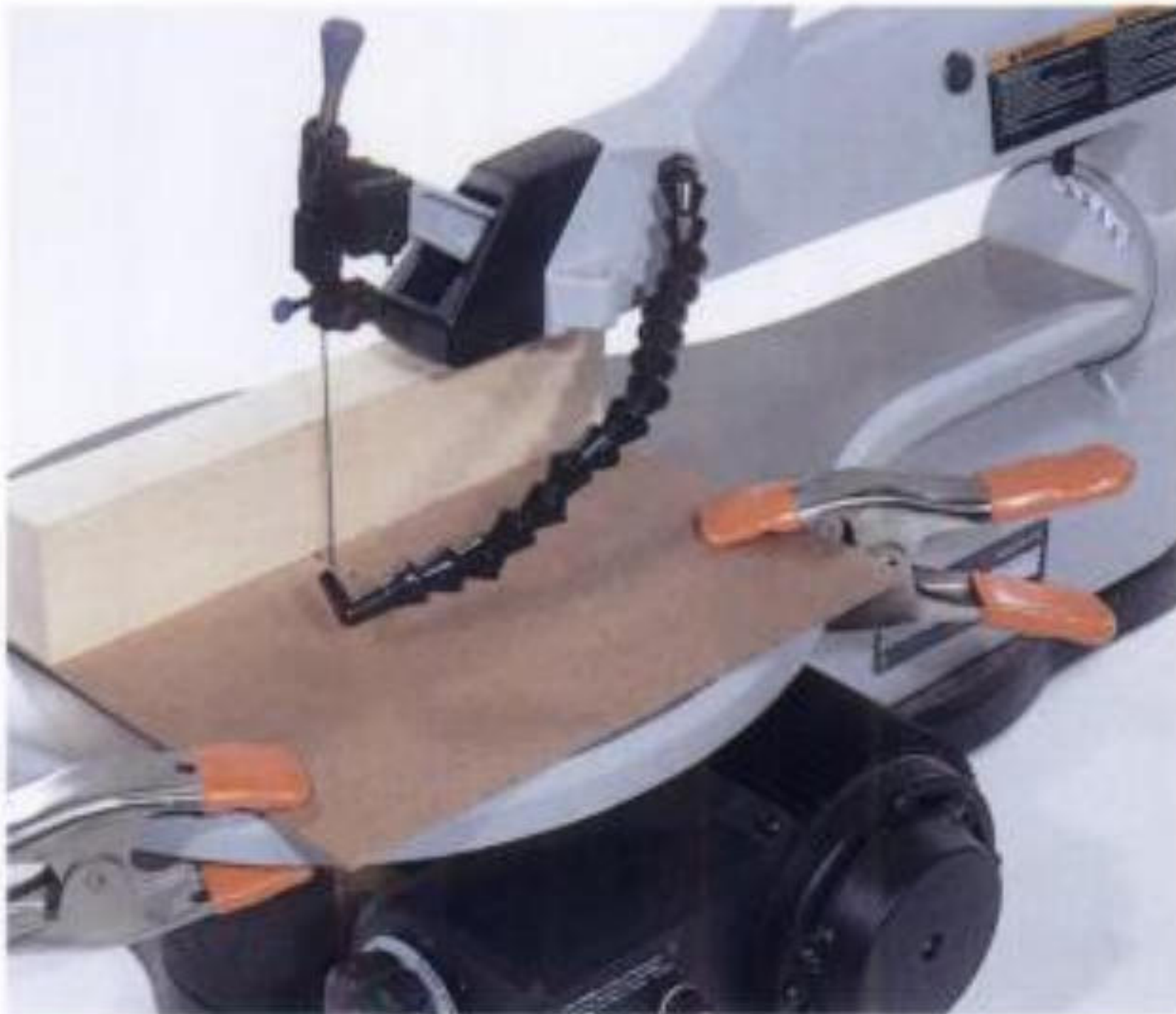
2-25. The ripping/resawing fence clamped to the scroll-saw table.
