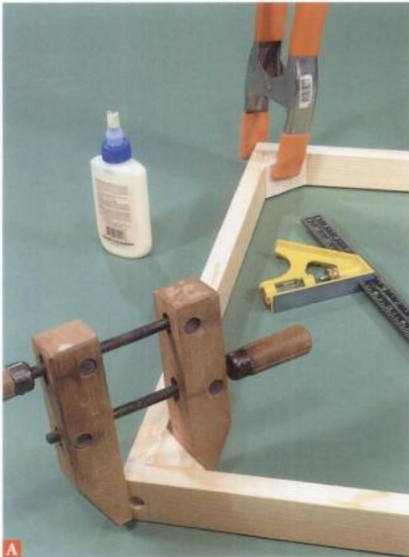
A Inside corner blocks glued in place.
