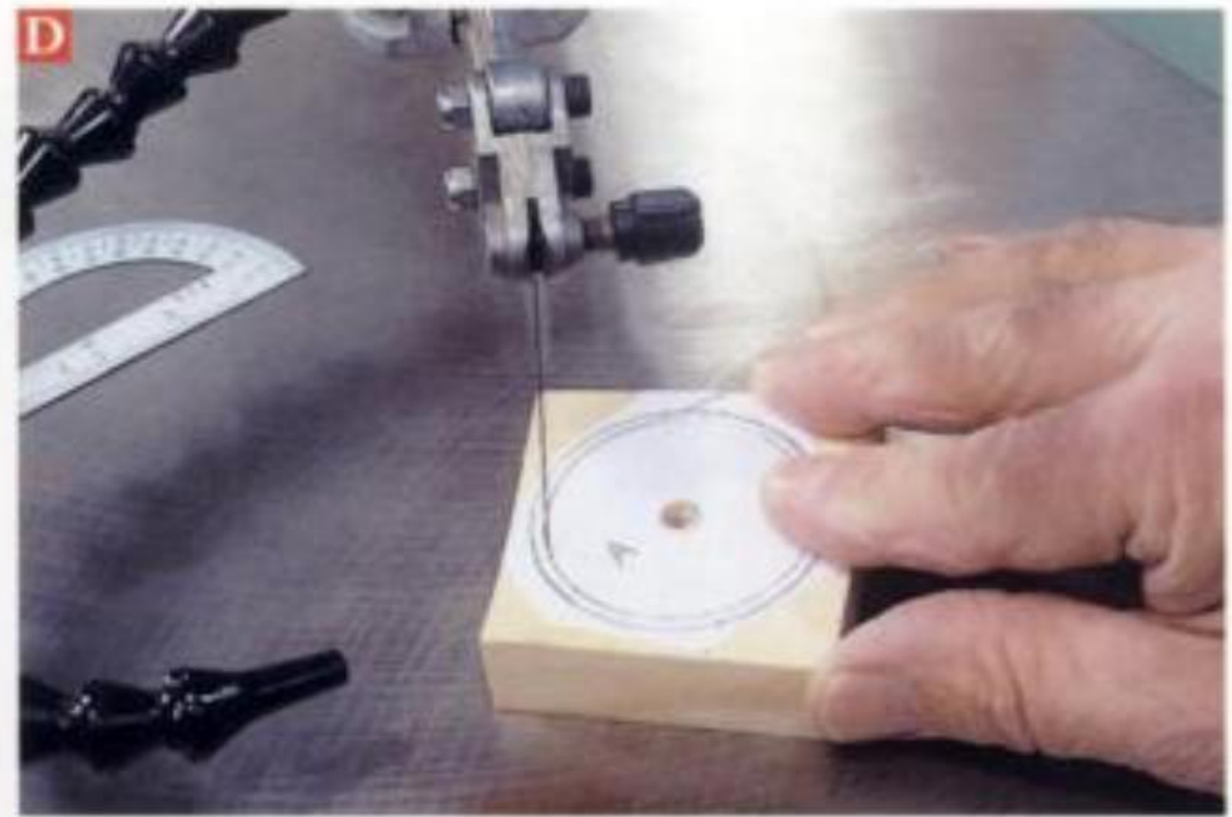
Cutting the lower tower pieces at a 5-degree bevel employing a clockwise feed and following the inside line.
