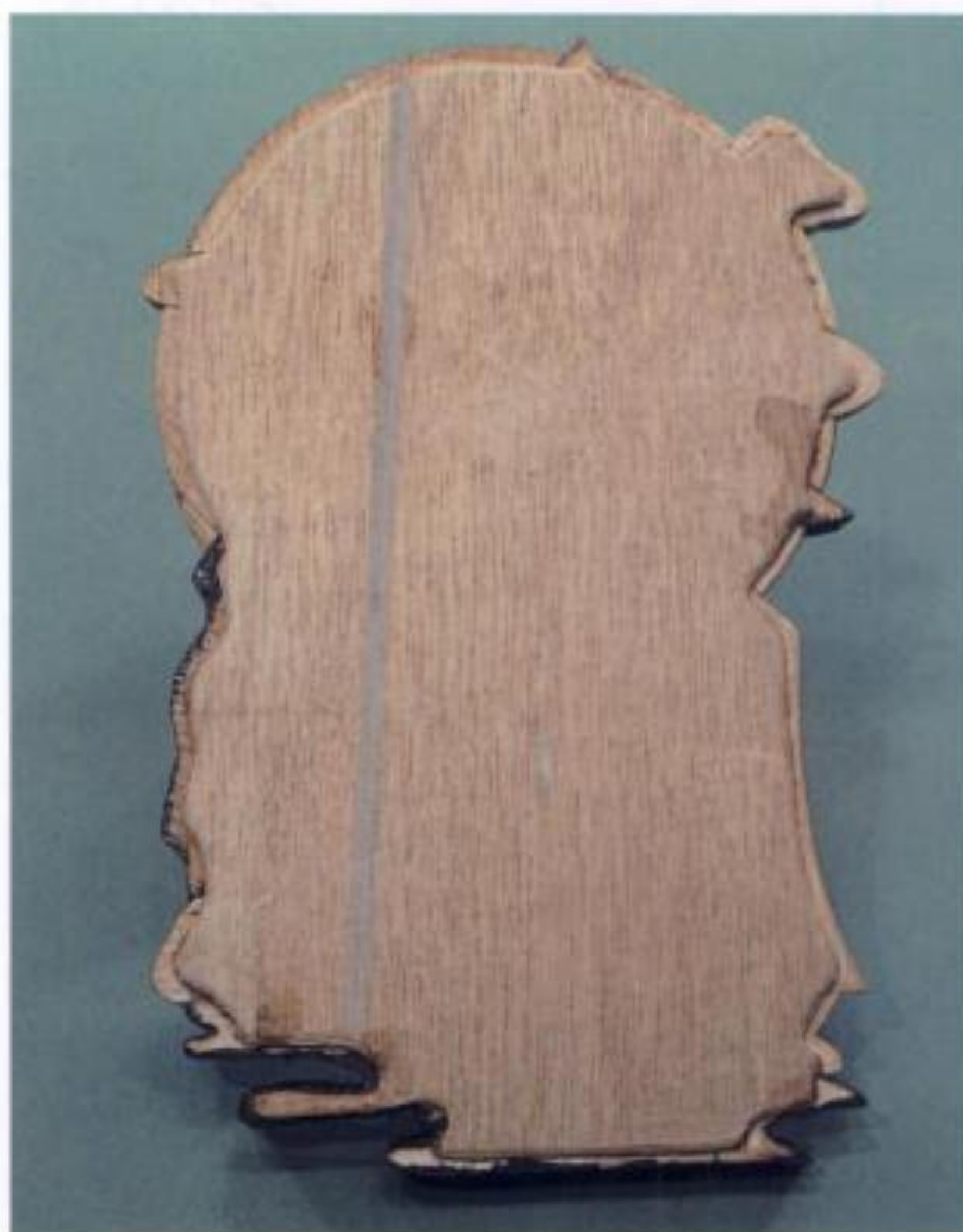
2–41. This rear view shows a backer made from recycled plywood wall paneling that is cut slightly smaller than the face profile and has beveled edges.
