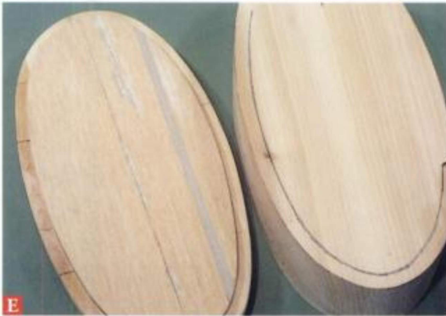
E The appropriate wall thickness is finger-gauged all around the sawn block.
