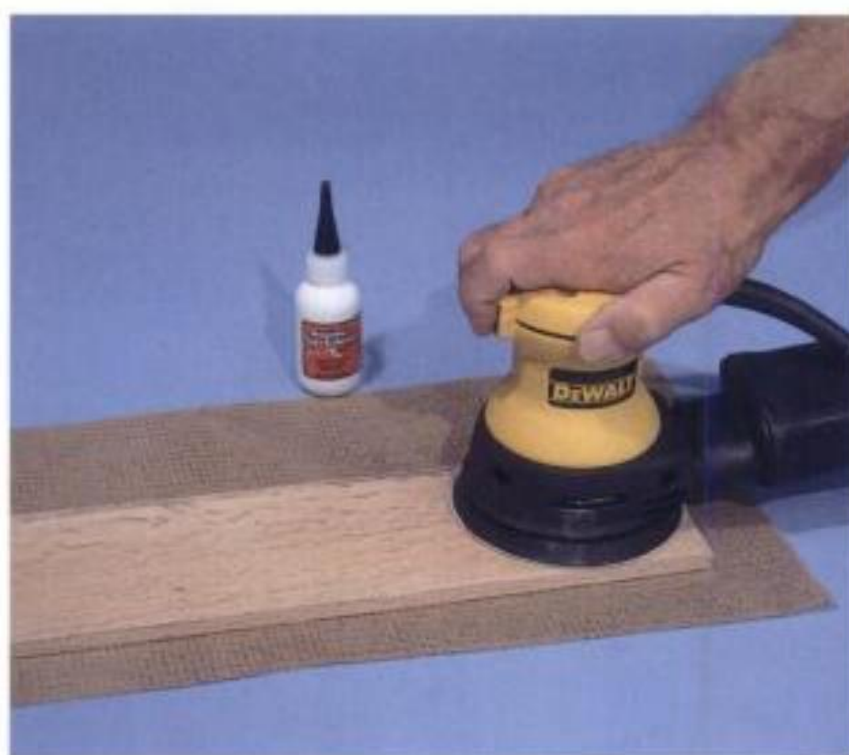
1-12. A random orbit sander prepares the surface before mounting the photocopied cutting pattern.
