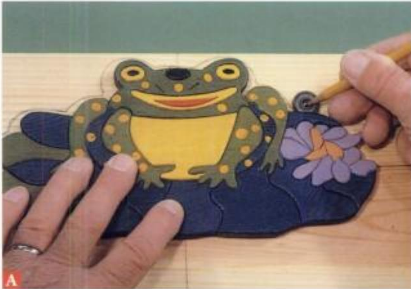
A The “washer trick” makes drawing a line parallel to the general profile shape easy.
