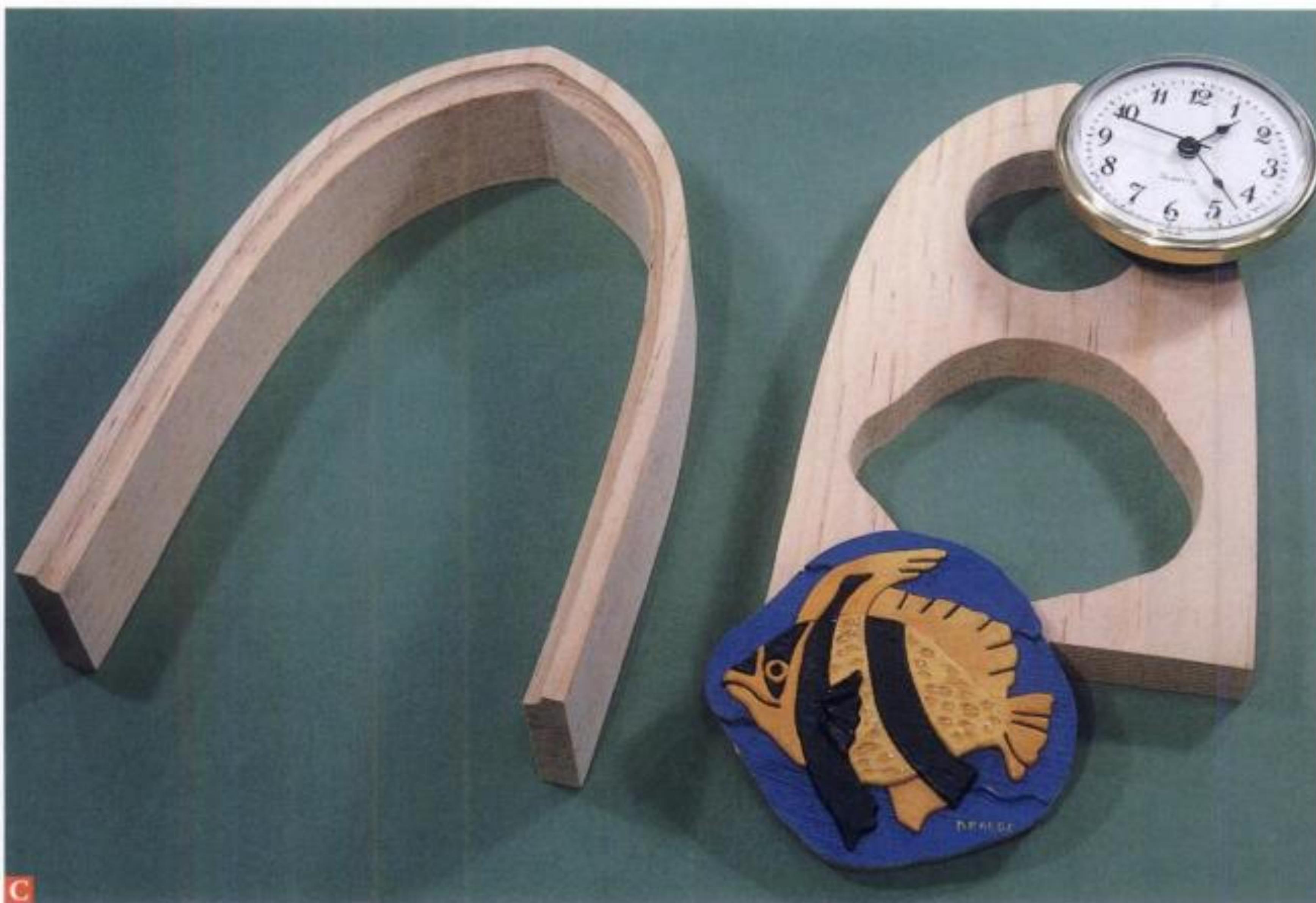
C The completed components. Note the face panel, which is the inside piece remaining from sawing the thick arch. It was then subsequently resawn to a \frac{3}{4} -inch thickness.
