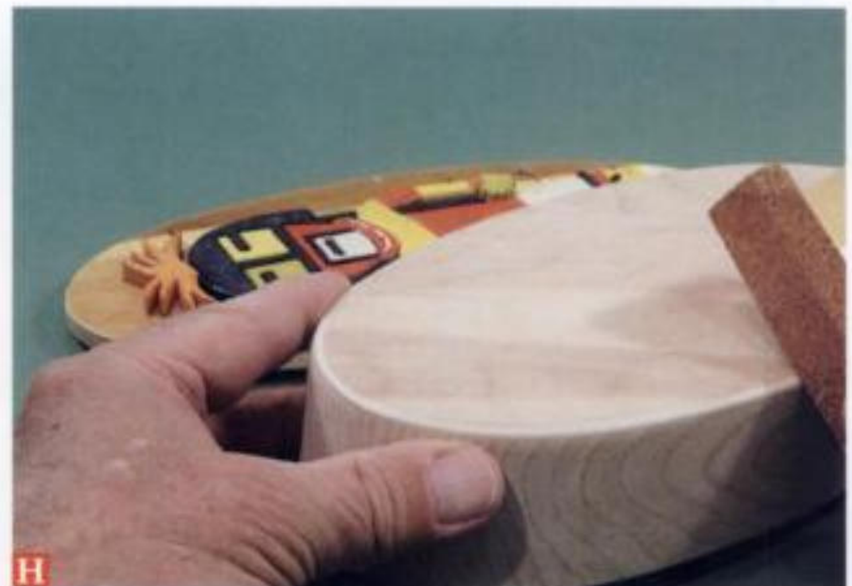
H Sanding back the bottom edges so they are not visible.
