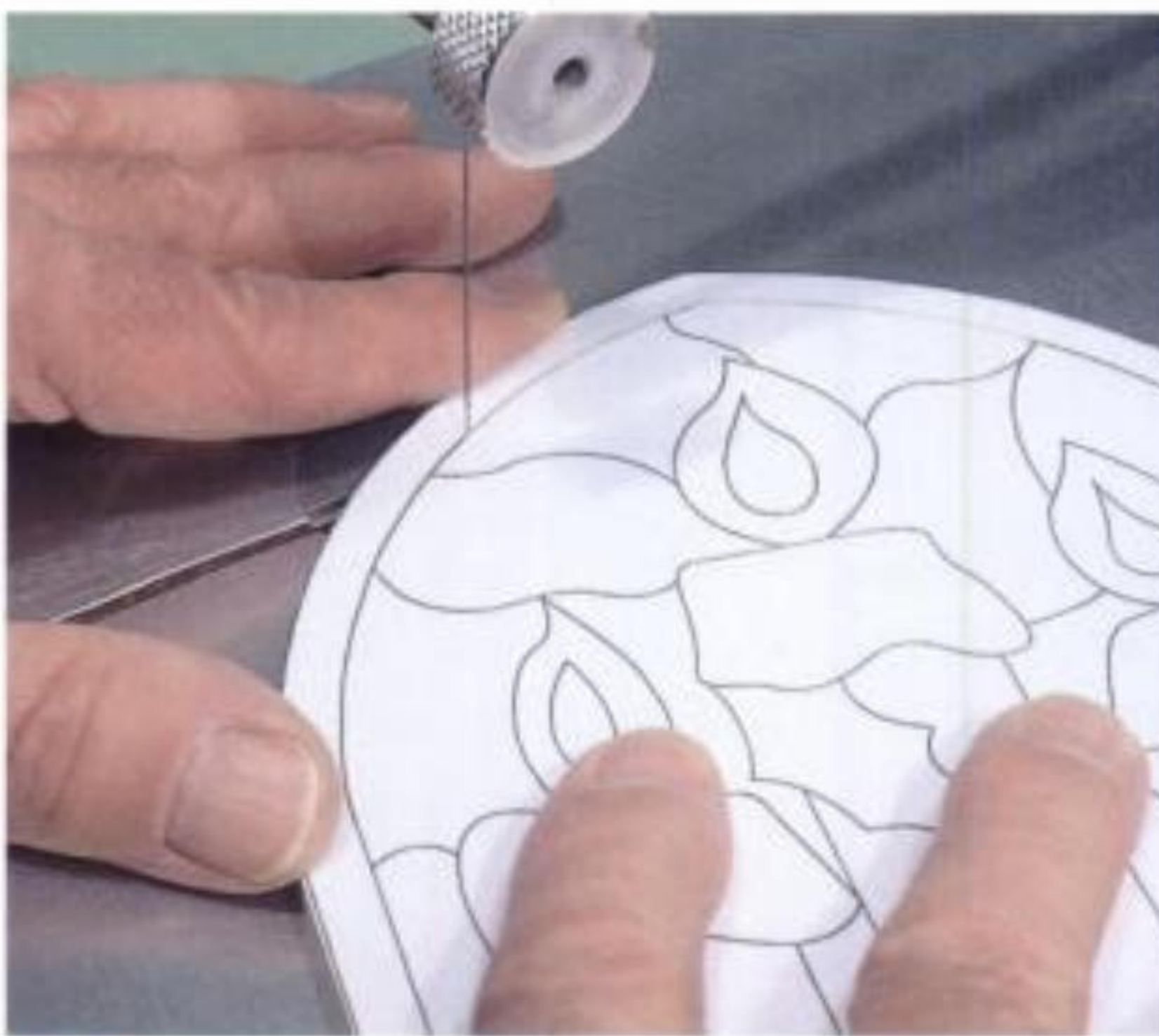
2-15. Sawing technique for cutting a parallel line to a curved or straight edge. The two stationary fingers of the left hand act as contact points and a cutting guide while the stock is advanced with the right hand to complete the curved portion of the cut.
