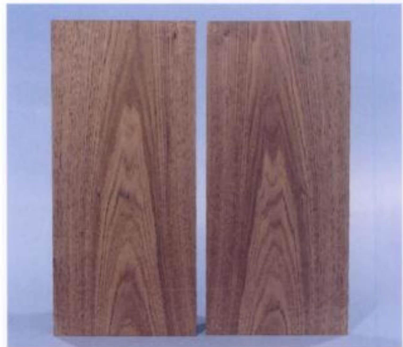
2-6. Resawing may produce two or more usable pieces from one board.
