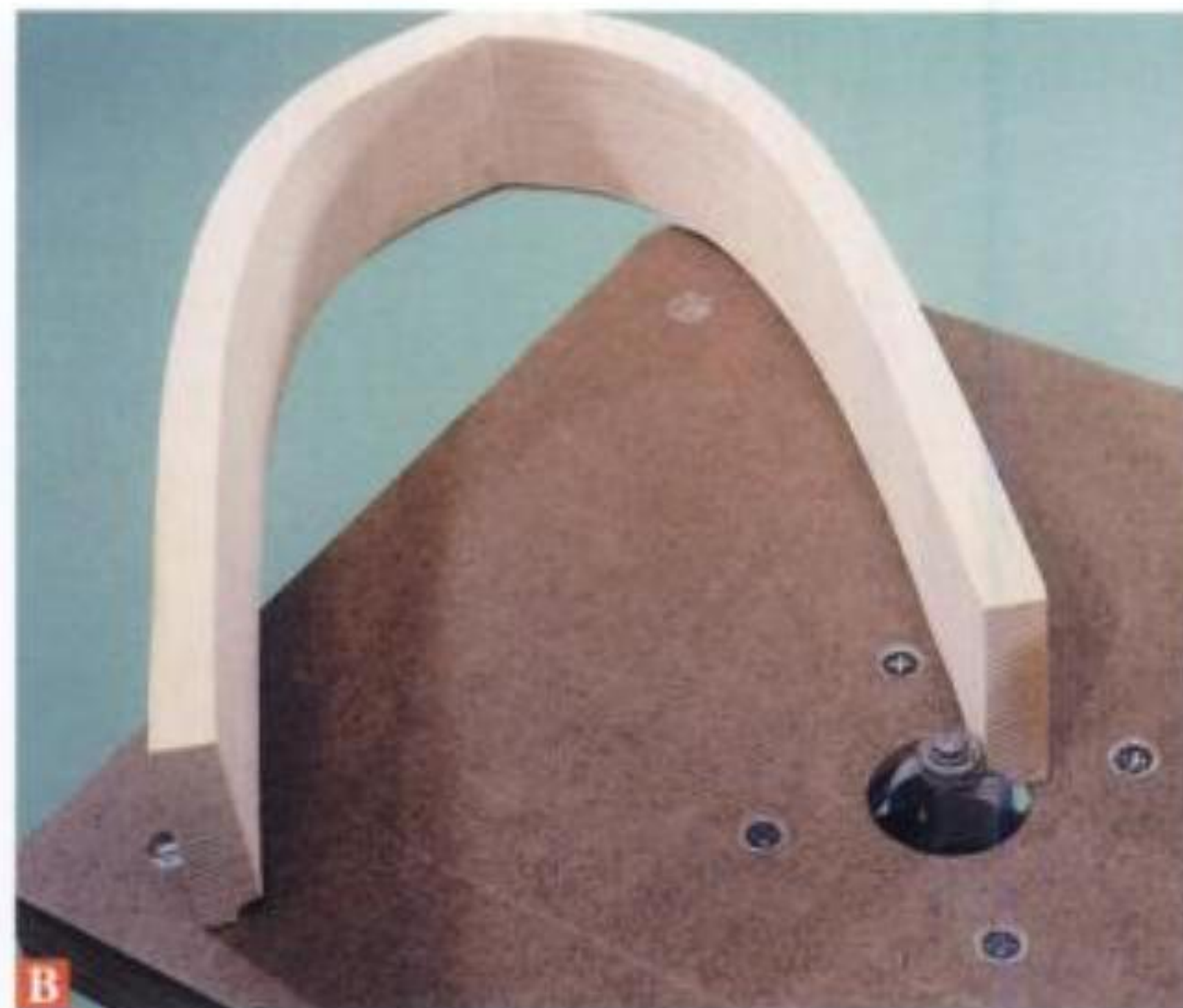
B Routing the inside edge of the arched frame piece.
