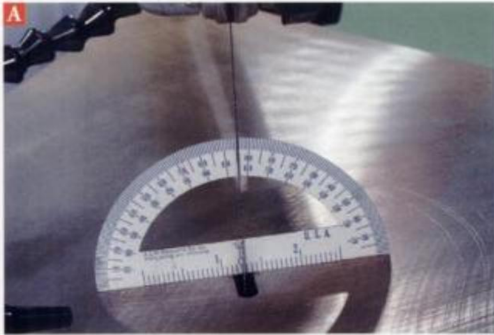
A protractor used on the table makes setting the amount of table tilt for bevel-sawing easy.
