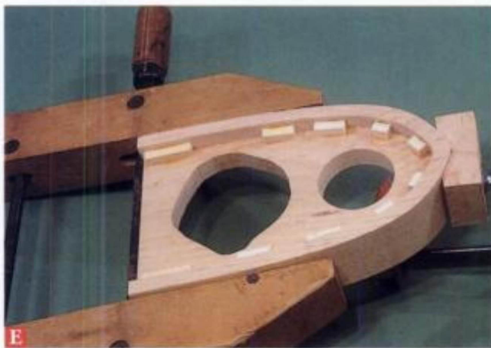
This rear view shows the use of glue blocks.
