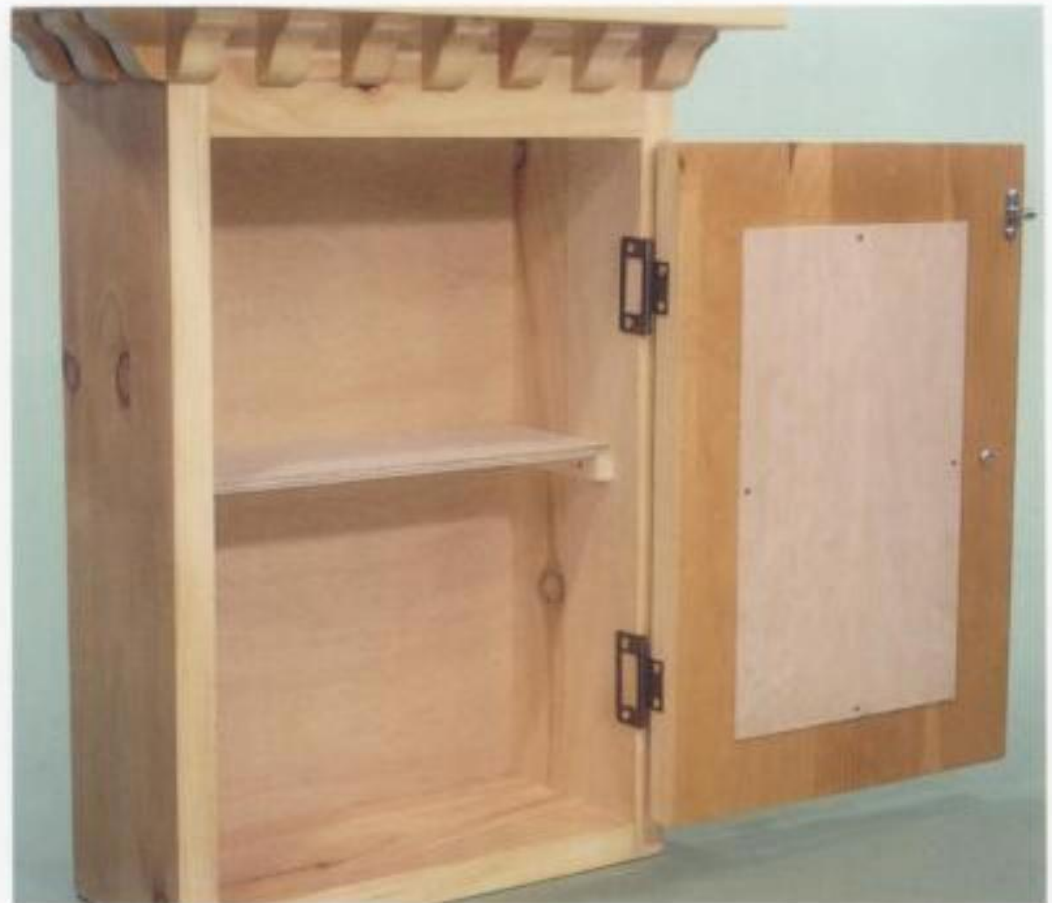
A thin piece of plywood, tacked inside the door as shown, hides the backer side of the rabbeted overlay of the dragon intarsia assembly.
