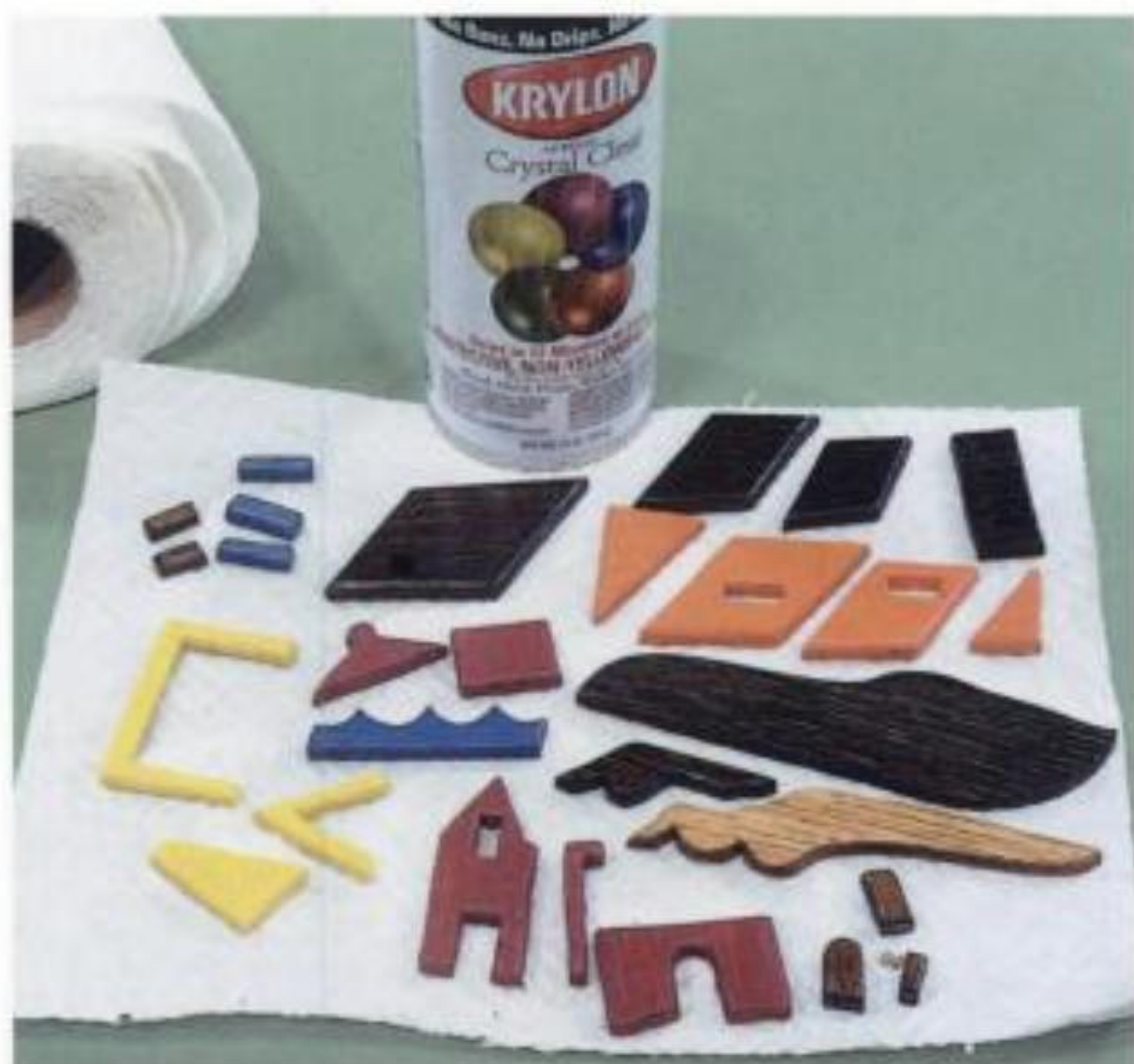
2-36. Stained and colored pieces ready to be glued to a backer.
