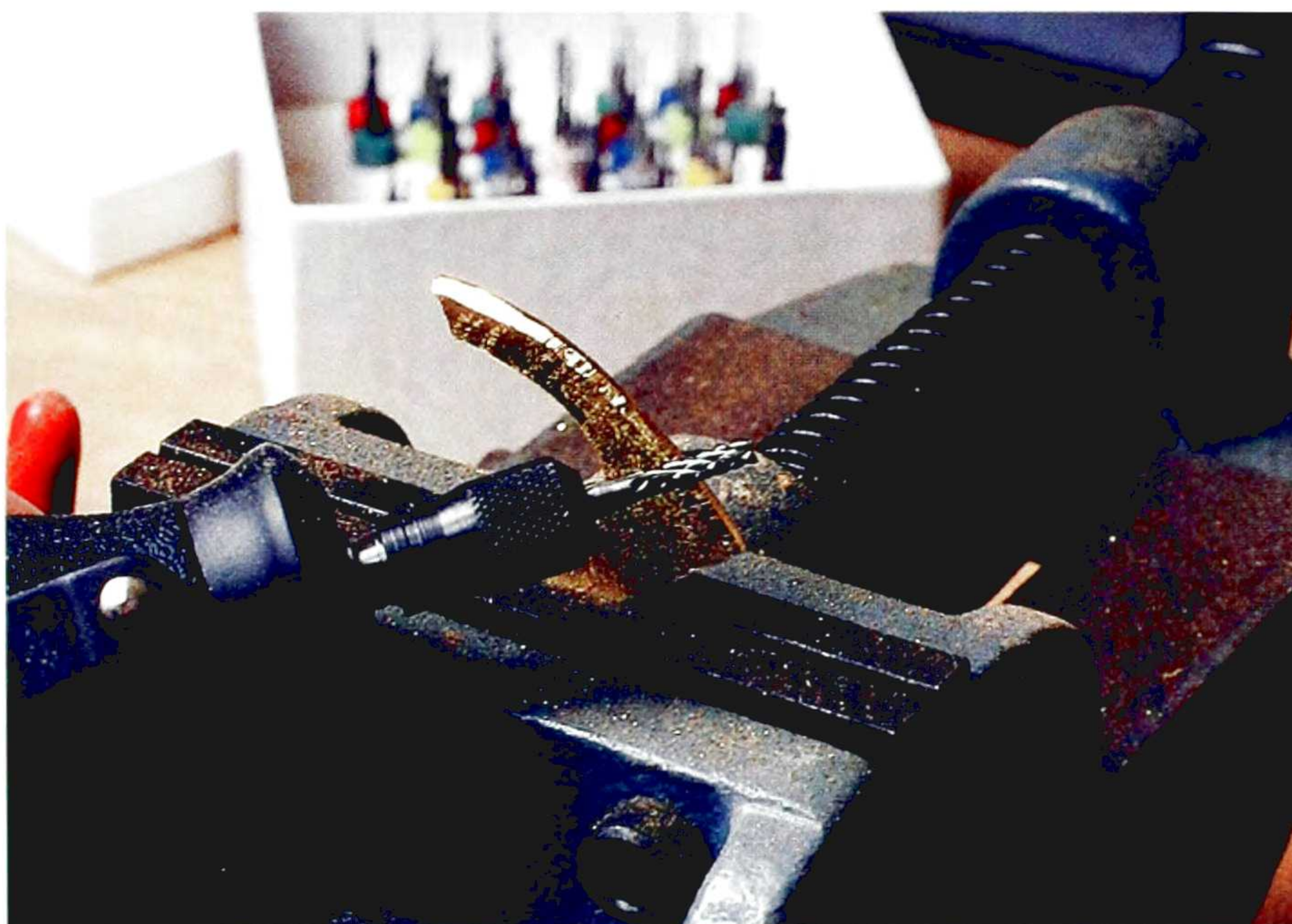
Using the minidrill to shape the brass pieces before positioning them on the front panel
