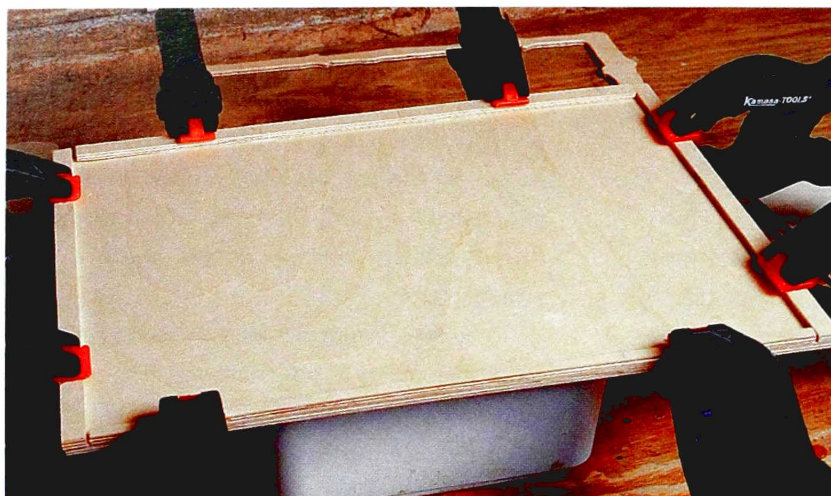
Clamping the in-between pieces of ply in position while the glue dries
