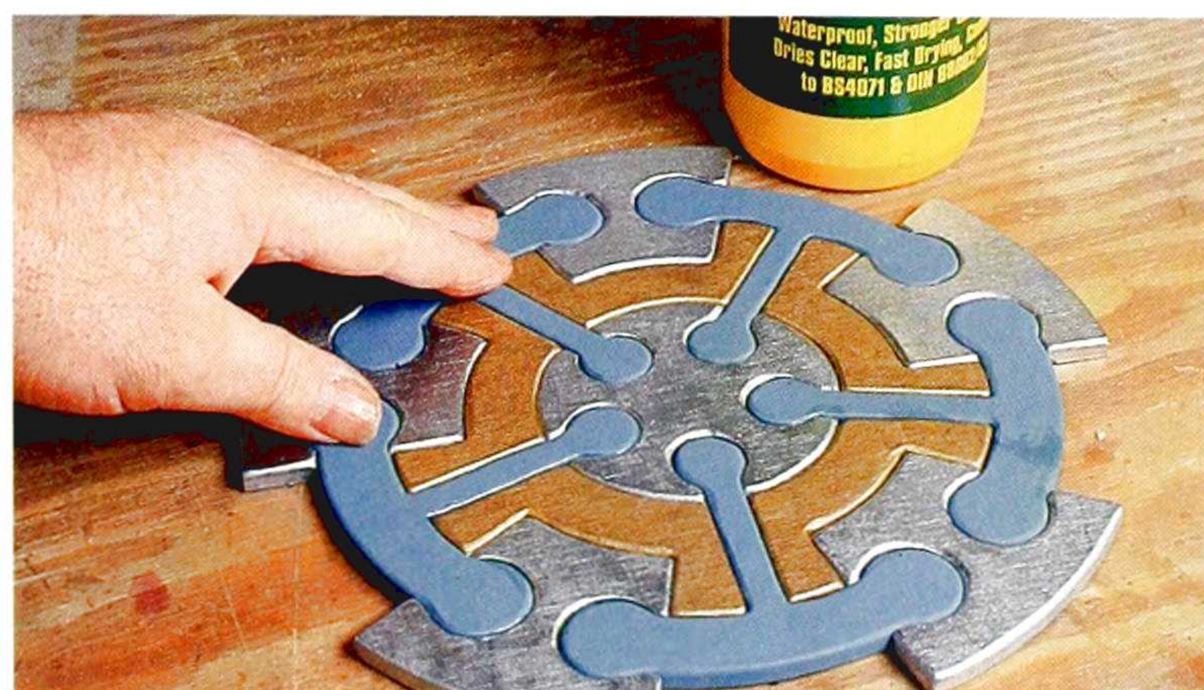
Gluing a protective cork base to the plate stand
