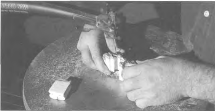
Recutting the second terrace to bring it up to the right height.
