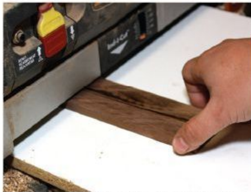
Plan ahead and plane 16" (406mm)-long pieces of lumber that can later be cut to the necessary length for a project.
