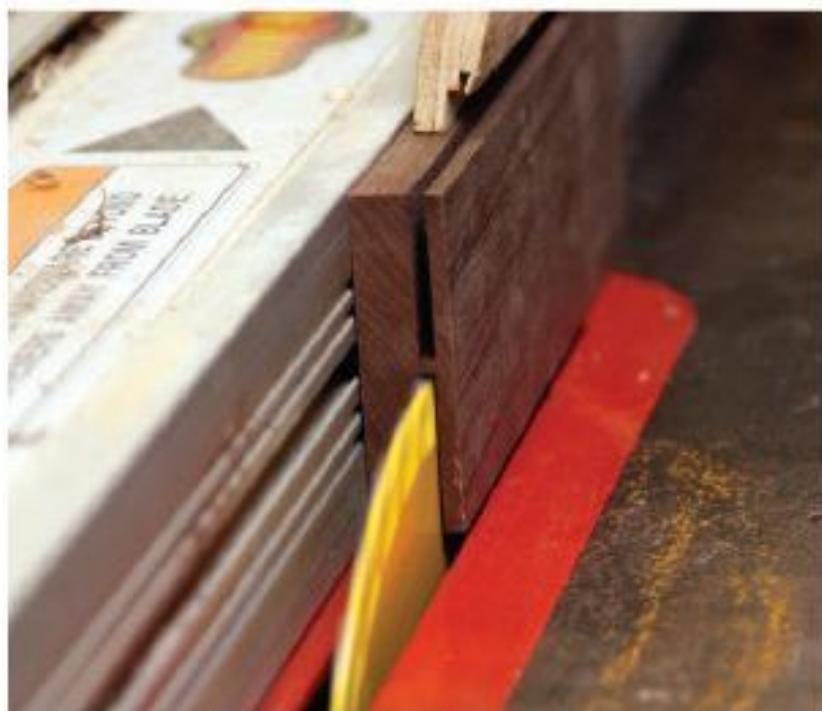
You can re-saw lumber using a table, but you must remember to take extra safety precautions.
