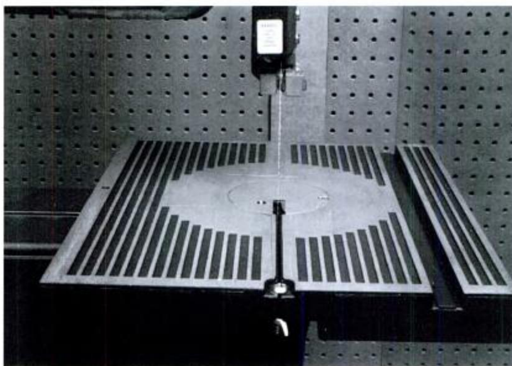
Illus. 4-5. The grooves in a band saw table like this one cause hang-ups when cutting curves. A special pad eliminates this nuisance.
