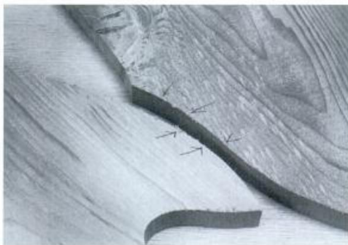
Illus. 4-10. Above: The saw blade forms burrs like these each time it makes a cut. Right: A sanding block removes the burrs from the pieces before resawing so they will lie flat on the saw table.
