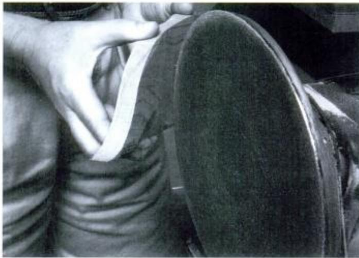
Illus. 6-1. The edge of a disc sander makes a handy carving tool, and its face removes wood quickly.
