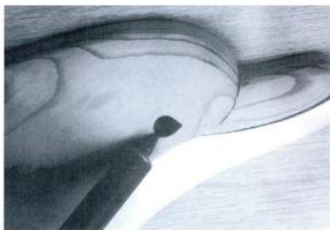
Illus. 6-23. Using a wood burner, burn the inside circumference of the hole drilled for the eye. Then use the burner to make corners on the eye.
