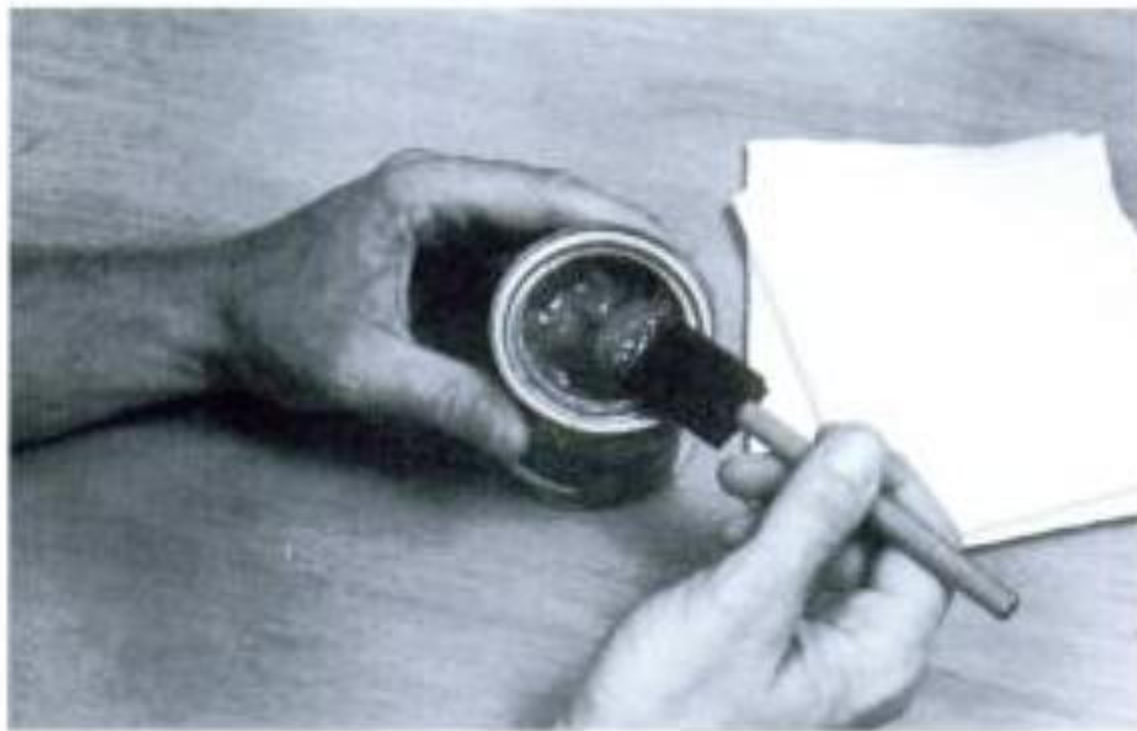
Illus. 7-4. For a professional finish on intarsia projects, use a foam brush to apply three coats of a clear wiping gel like the one shown here. Wipe the gel off with folded paper towels.
