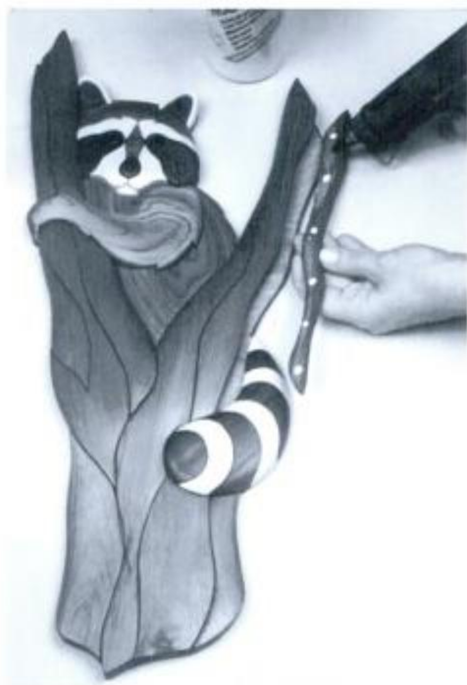
Illus. R5-3. First, glue down the outer segment of the upper right branch. Dot wood glue (white in the photograph) on the back of the part; then apply hotmelt adhesive between the dots.
