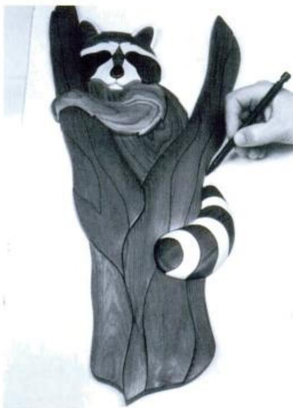
Illus. R5-2. With the Raccoon parts assembled on paper-covered backing plywood, trace around them to make an outline on which to cut the backing. Note that all parts are carefully spaced as for the finished piece.
