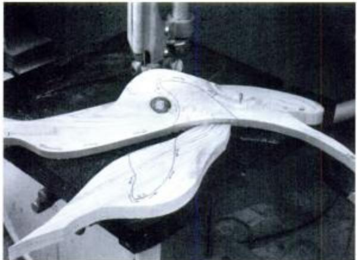
Illus. 4-29. Next saw the dorsal fin and flipper from their blanks. Note the completed body of the larger dolphin underneath the blanks.
