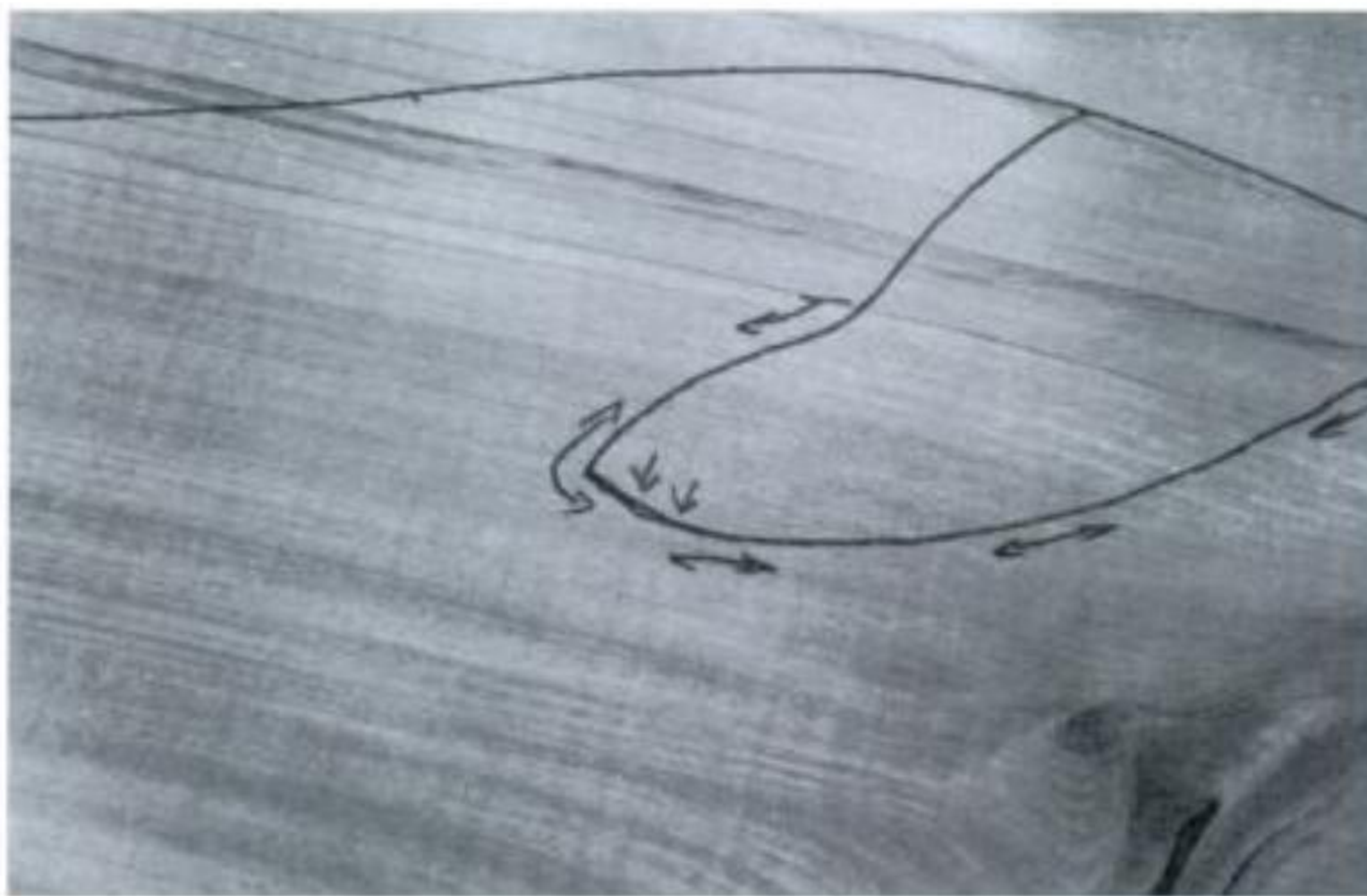
Illus. 3-10. Extending a pattern outline beyond the actual part, as though you were beginning to draw the adjoining part, provides a "lead" on which to line up the saw blade.
