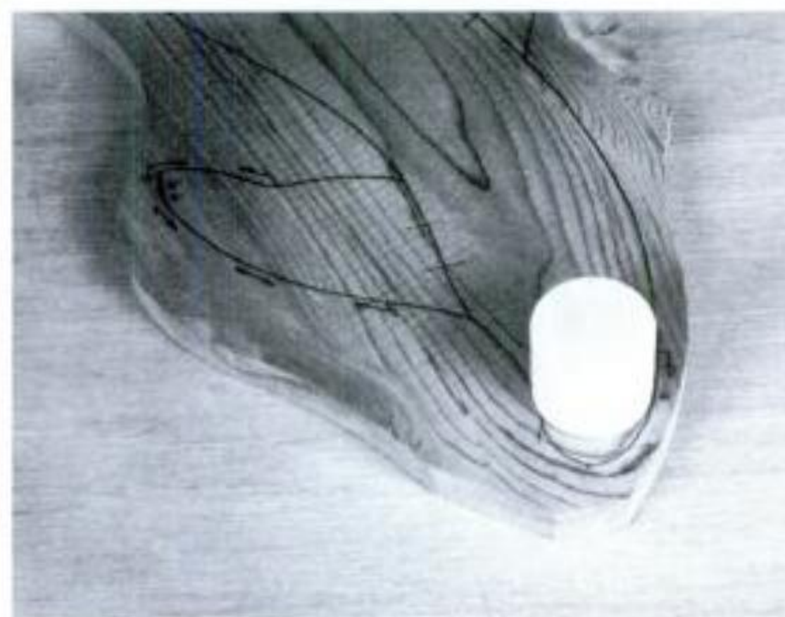
Illus. 4-18. Left: A band saw with a 1/8" blade can cut the outside curve of the dolphin's head without peeling. Right: Cut relief slots around the outside curve of the dolphin's head before trying to cut it with a 1/4" blade.
