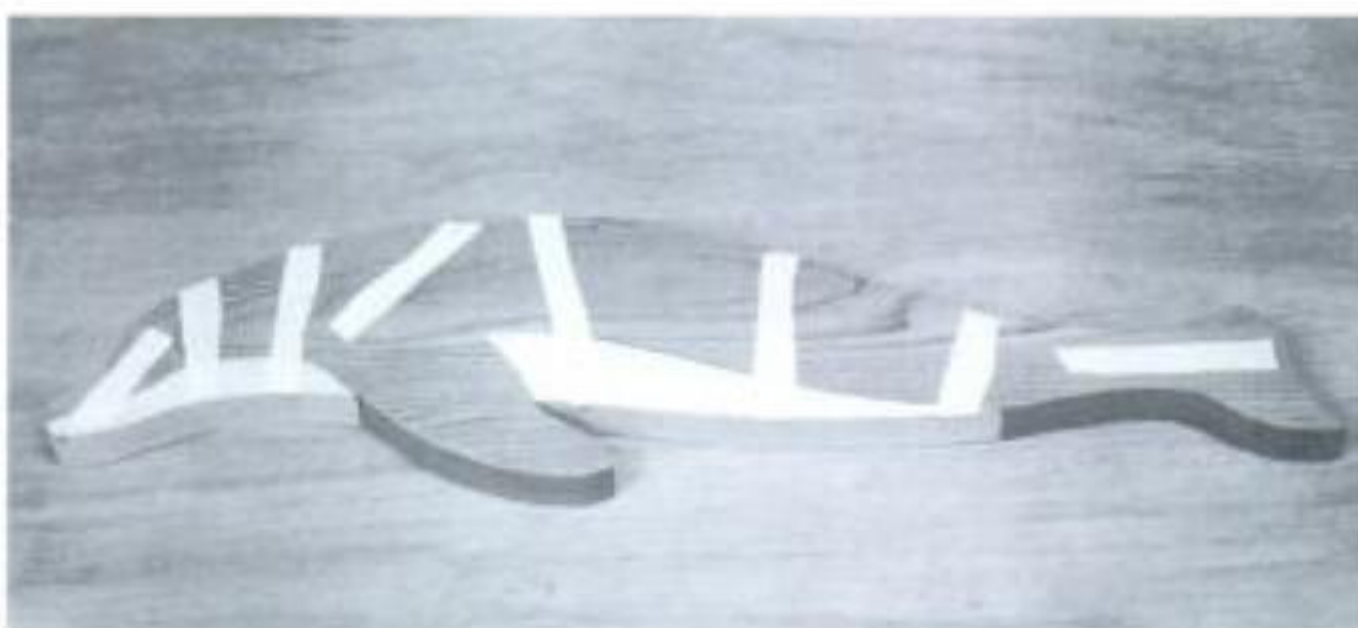
Illus. 6-17. Tape the lower dolphin's body parts for unit sanding. Use the flipper as an aid to position the belly parts during taping.
