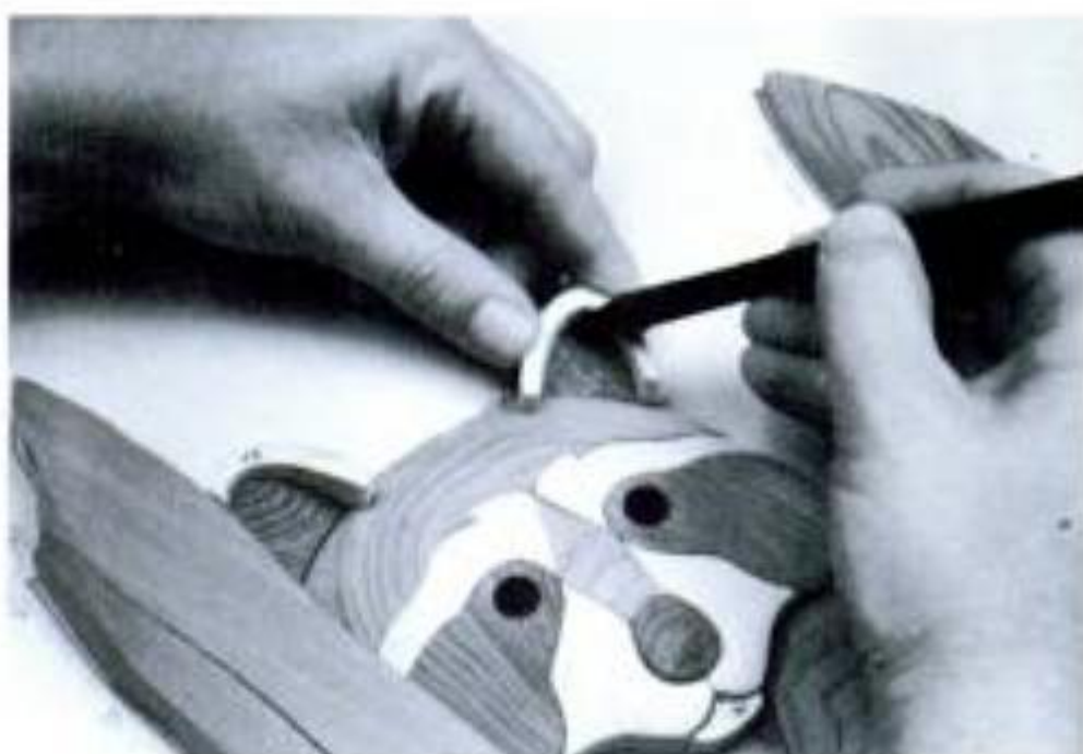
Illus. R4-22. After sanding the dark ear parts, put them in place and mark the thickness (about 5/16 ") on the inner edge of the white ear parts.
