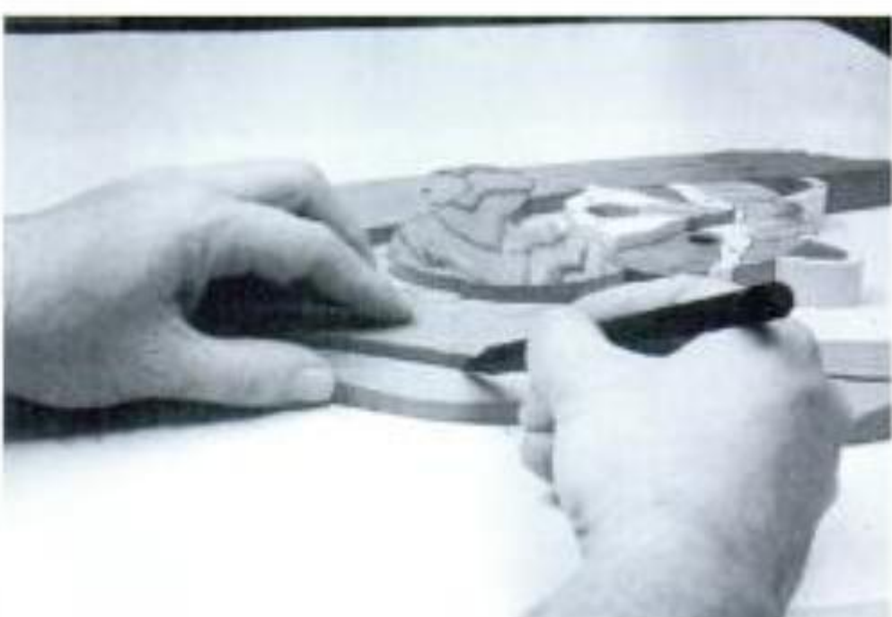
Illus. R4-8. After you sand each part, put it in place and mark its thickness on any adjoining parts.
