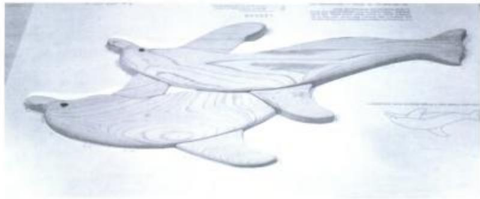
Illus. 6-25. These two views of the Dolphins show how the parts should be sanded and shaped to give the project dimension. Areas farther from the viewer are thinner; those closer are thicker. Exposed edges are rounded, and areas where parts join are hand-sanded for smoothness.
