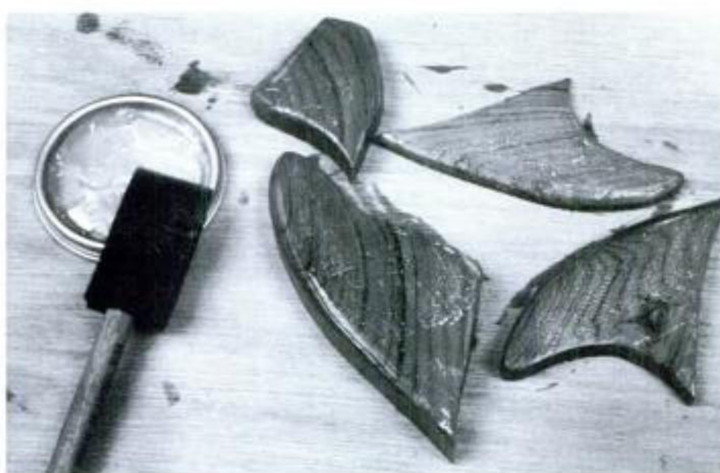
Illus. 7-7. Coat only three or four parts at a time. Wipe those off and then coat the next group. Note the thickness of this first-coat gel application.
