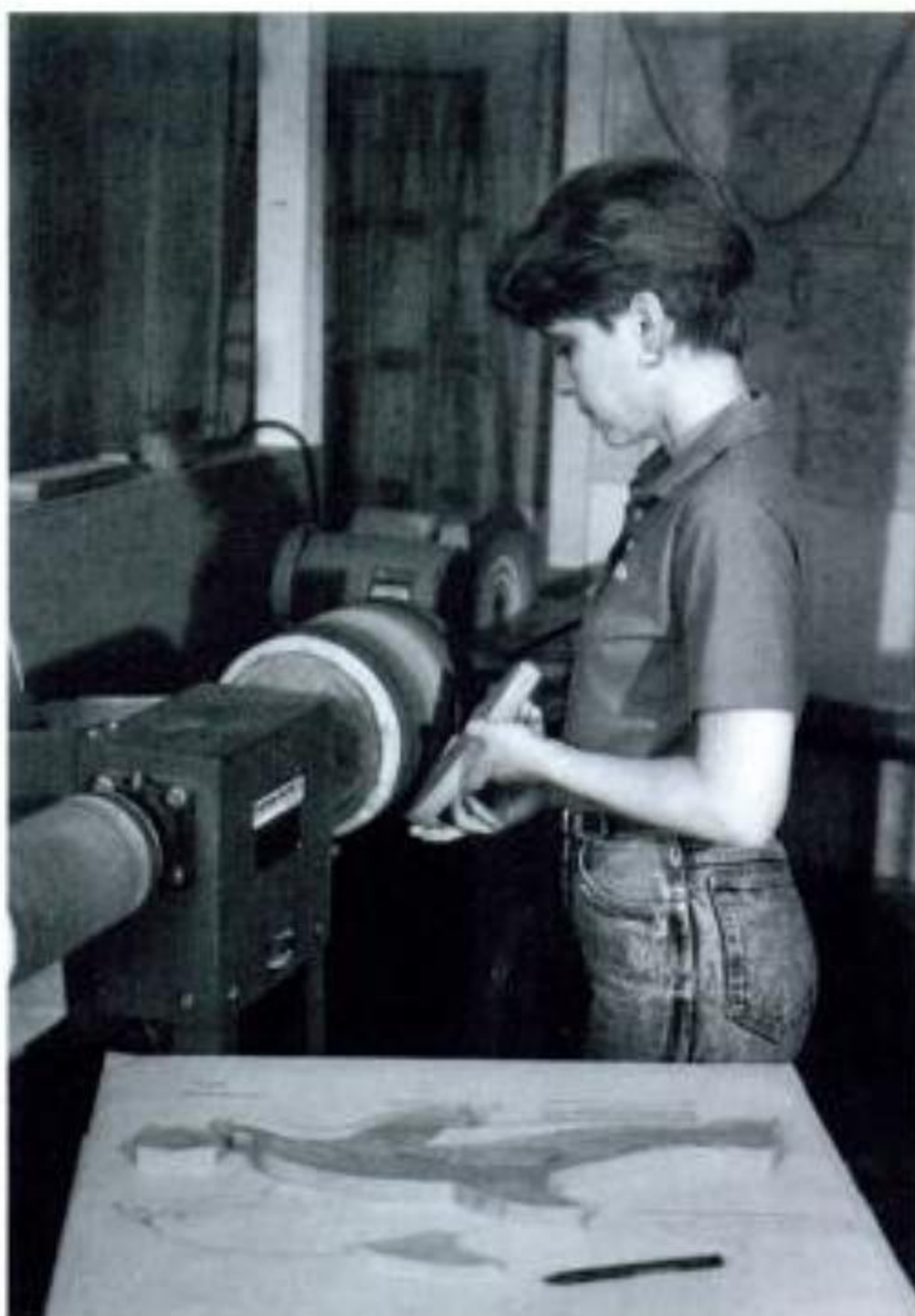
Illus. 6-5. Having the project close at hand as you sand refreshes your memory about how much wood to remove from a part, whether it has an exposed edge, and other aspects of the project as a whole. Note: Eye protection and dust mask removed for photography.
