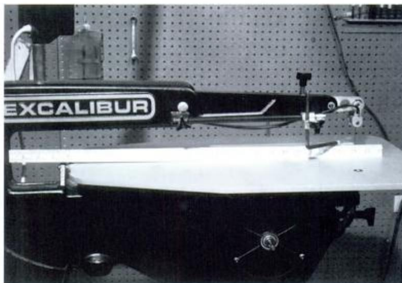
Illus. 4-2. This 24" scroll saw should accommodate almost any intarsia project.
