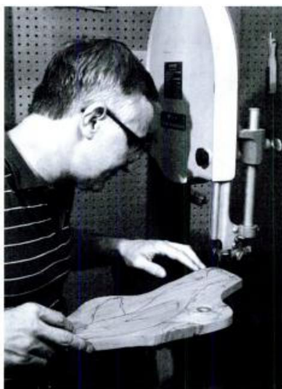
Illus. 4-20. If a piece exceeds the saw's throat capacity, figure out where to start the cut so that the piece will swing away from the saw column as it is sawed.
