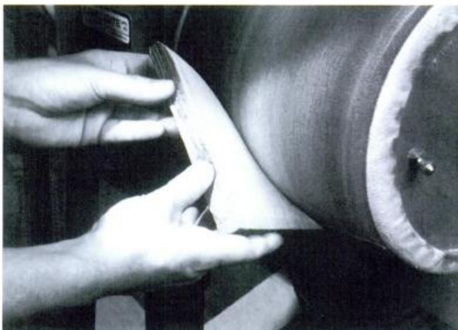
Illus. 6-3. A pneumatic drum sander produces smooth rolling curves. Its soft drums (filled with air just like a tire) make this type of sander easy to work with.
