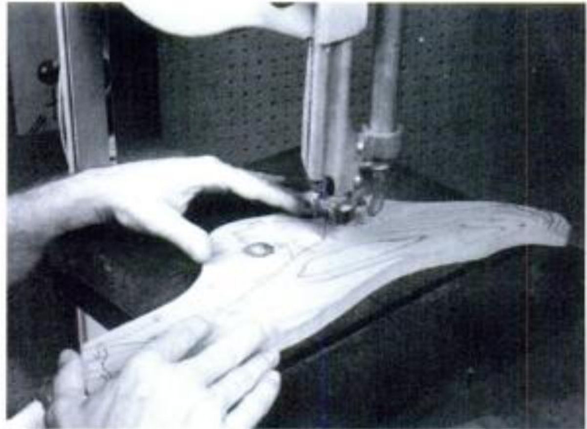
Illus. 4-28. Exit the cut at the end of the tail, sawing straight off the end of the blank.
