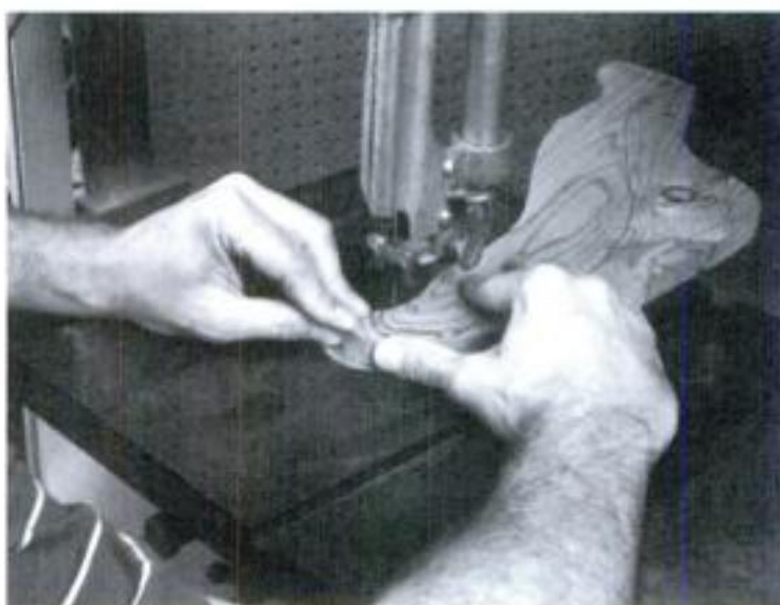
Illus. 4-25. After deburring the piece, replace it on the saw table and begin the cut again. Note that you swing the piece away from the saw column as you cut around the head.
