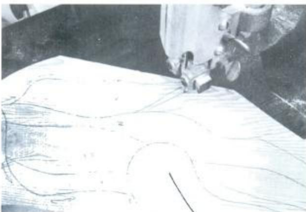
Illus. R2-3. To cut the outline of Part 2, first saw an escape cut like this one in the adjacent waste wood. Stop the saw 1/8" from the point where the escape cut would intersect the outline of the part.
