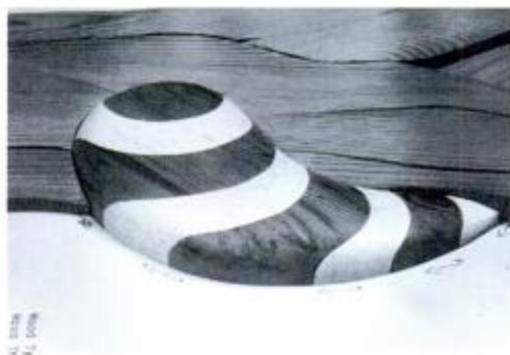
Illus. R4-27. Sanding all the tail parts as one (attached to the sanding backing with tape), taper the tail down to about 3/16 " at the small end. Round the tail down below the pencil line on its upper half but above the pencil line on the lower end. Round the exposed edges toward the outside.
