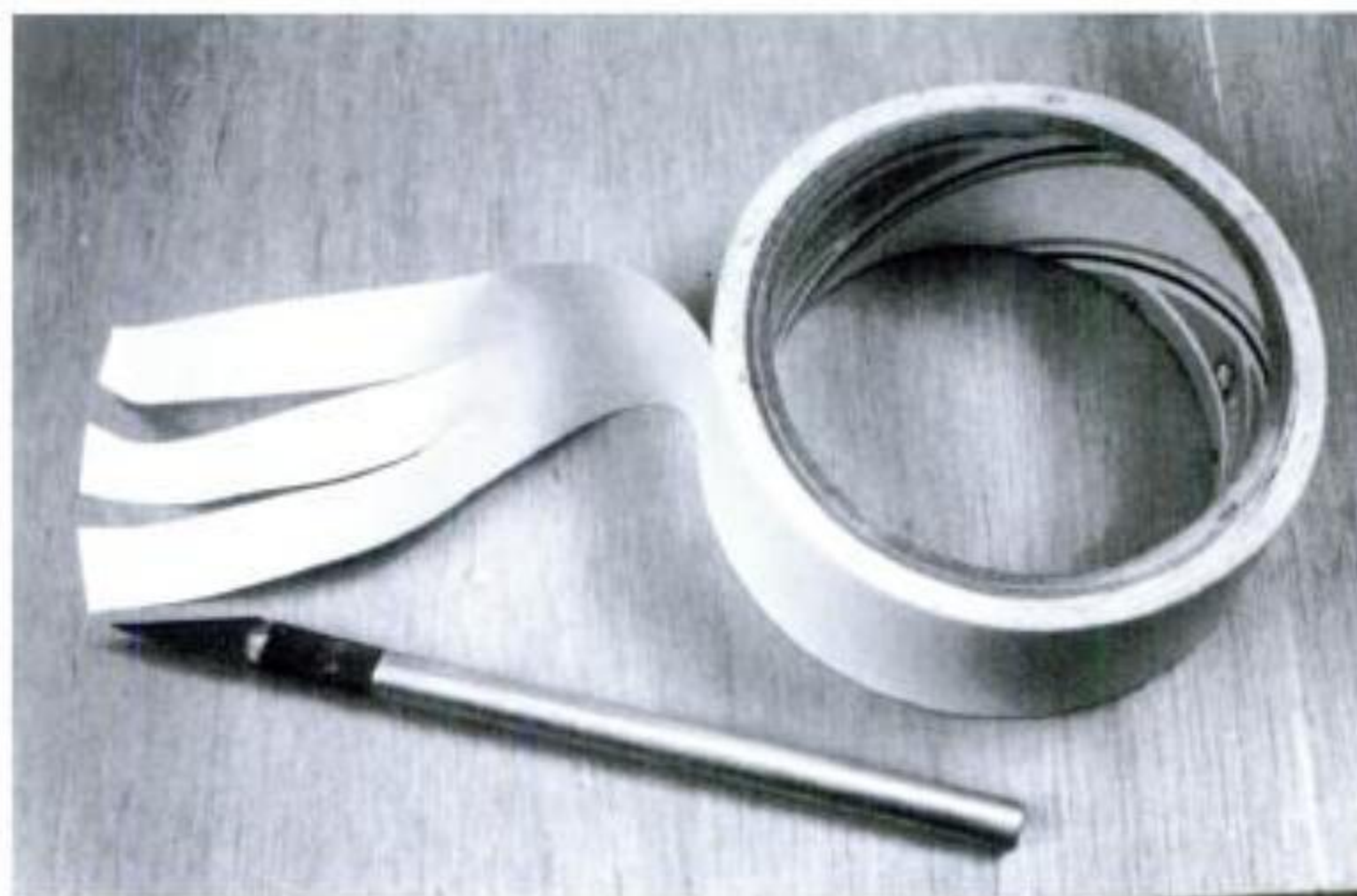
Illus. 6-8. Use double-sided tape to attach intarsia parts to a temporary backing for sanding. Cut the tape into thin (1/2" thick) strips to make it less aggressive.
