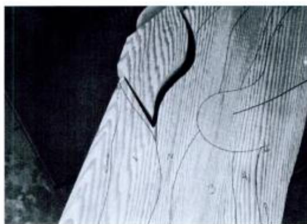
Illus. R2-4. Back the saw out just a little and then saw toward the escape cut. Plan the location of the escape cut so that the waste piece is tapered like a wedge.
