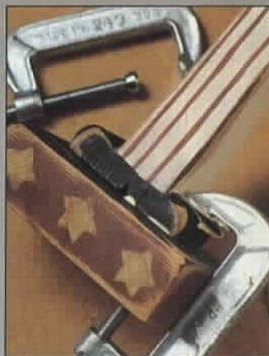
Apply glue to mating surfaces, clamp pieces together, and wipe away glue squeeze-out.
