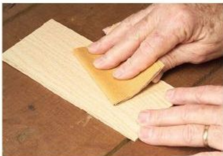
Figure 1. Be sure to sand the workpiece before applying the pattern. You may also want to sand the wood lightly once you have cut the design and removed the pattern to eliminate any “fuzz” and to get rid of any glue residue.
