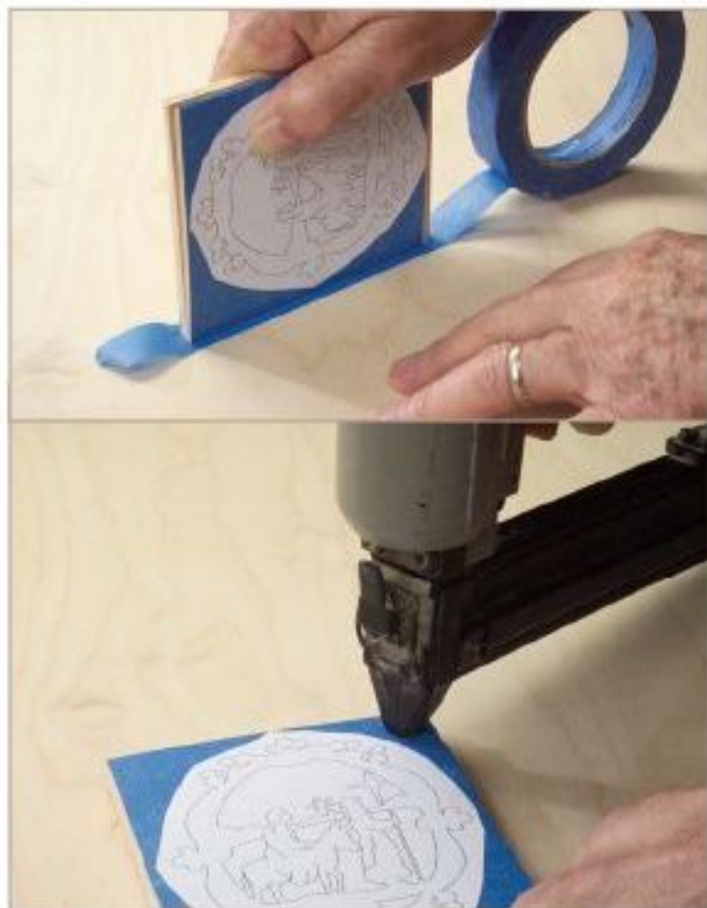
Figure 9. Masking tape or painter's tape (shown) placed around the edges can be used to hold a stack together. Some scrollers also like to cover the surface of the wood with tape before adhering the pattern to help lubricate the blade as it cuts. Driving nails in the corners of the stack can also be an effective method of holding the stack together.
