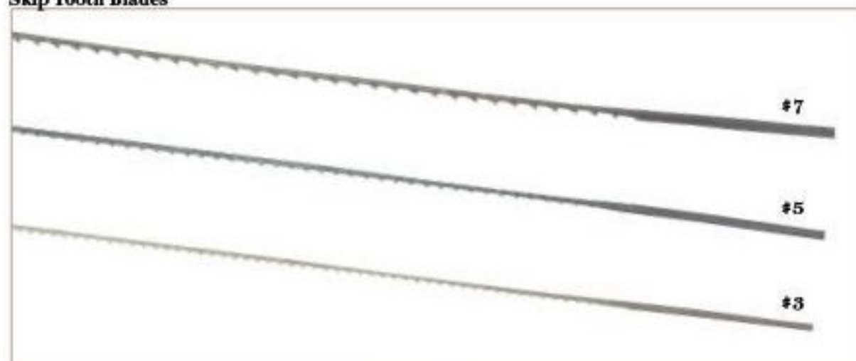
Figure 4. Skip tooth blades can be good blades for a beginning scroller. Pictured here from bottom to top are skip tooth blades #3, #5, and #7.
