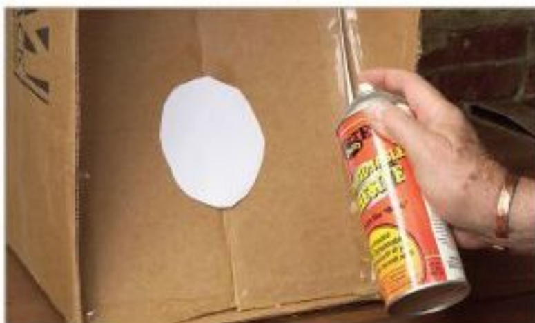
Figure 2. Use “repositionable” spray adhesive to adhere your patterns to the wood. A simple glue box, made from a common cardboard box, helps to confine the adhesive.
