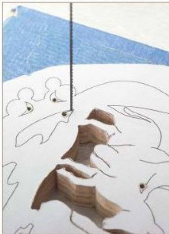
Figure 7. Drill any blade entry holes close to corners so that it will take less time for the blade to reach the pattern line.
