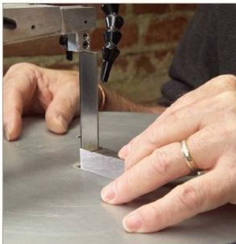
Figure 5. One way to check if your table is square to your blade is to use a small square. Place the square next to the blade and adjust the table as necessary until the blade and the square are parallel.
