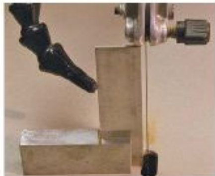
Your blade must be square to your saw table to produce close-fitting intarsia.
