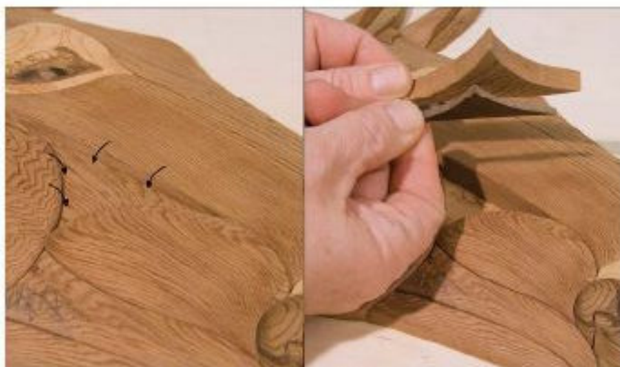
The arrows (left) show a piece that has been sanded too thin. Cut a shim to fit under the piece (right), raising the piece to the correct height.
