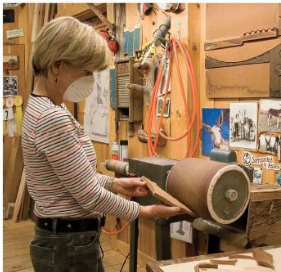
Judy uses an 8"-diameter drum with a 100-grit sanding sleeve to remove wood quickly.
