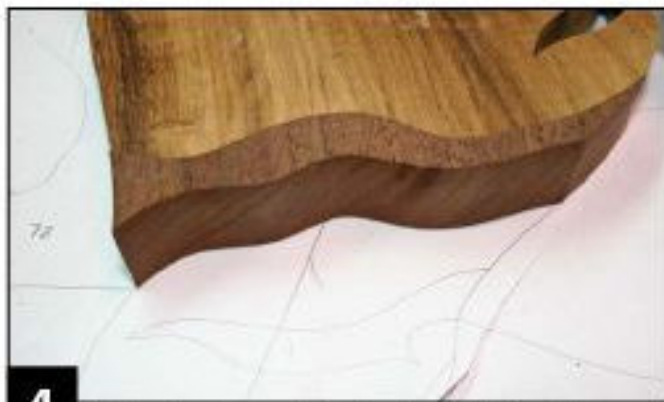
4 Cut the front legs and feet. Do not cut the stripes that are totally surrounded by the leg. Cut the full stripes and the legs, including the feet. Make sure to align the grain direction of the stripes with the legs.
