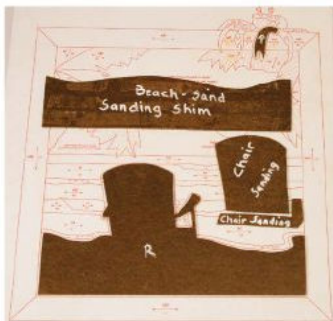
Use sanding shims to shape pieces in sections. Use rising shims to add dimension to the project.
