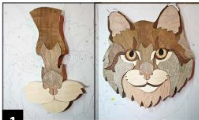
1 Cut the face. Start with the nose. Number the pattern and the bottom of each piece as you cut it. Assemble the pieces on a master pattern to check for fit and wood selection. Leave the small tufts on the tips of the ears connected to the ears for now.
