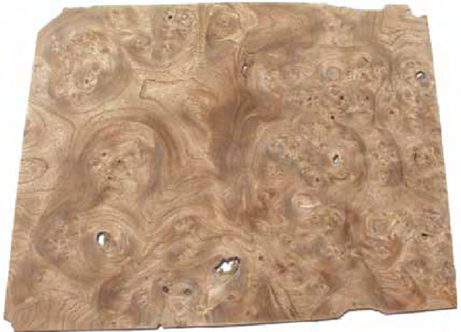
Figure 3. The Treated Veneer. After treatment, the veneer is smooth and pliable and ready for use in a marquetry project.
