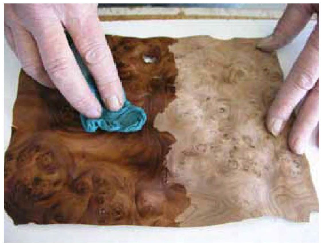
Figure 2. Wild Veneer Treatment. A solution of glycerin and water is rubbed on the front and the back of the wild veneer.
