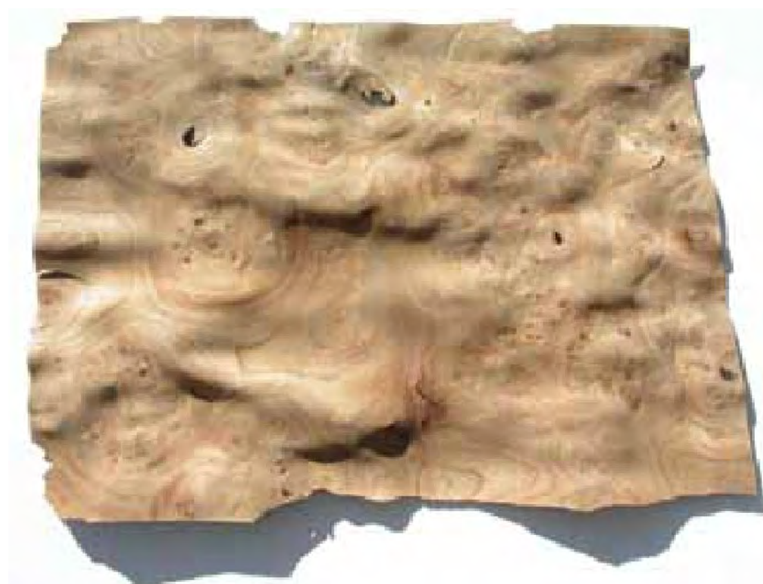
Figure 1. Flattening Wild Veneer. This wild Bubinga burl veneer is rough, brittle and has cracks and curls. As such, it is of no use in marquetry.
