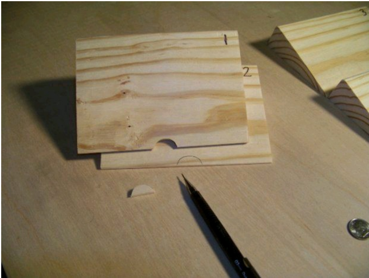
Figure 7 – The cutout from the first segment is used as a pattern for the next segment. Keep the thin edges aligned when tracing.
