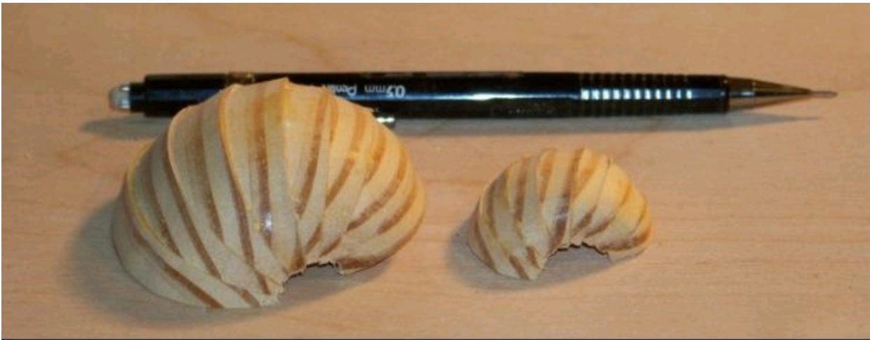
Figure 12 – After pairing 3 times, the segment groups contain 8 segments. Don't let yourself get ahead of the interior sanding that needs to be done while it is easy access.
