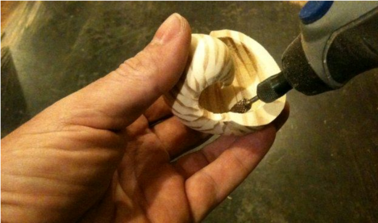
Figure 13 – Smoothing the interior. The flat faces from the saw cut need to blend together to form a smooth continuous curve.
