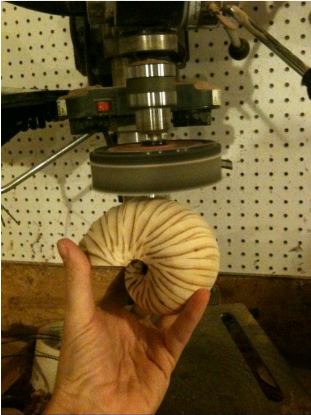
Figure 15 - Use a disc sander with thick foam pad in a drill press to smooth and sand the exterior.
