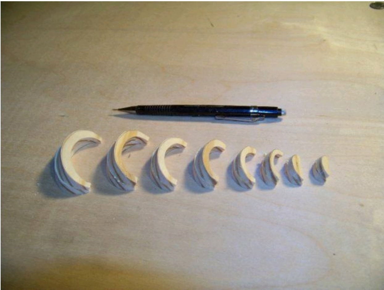
Figure 11 – The first 16 segments are glued to become 8 pairs of segments.
