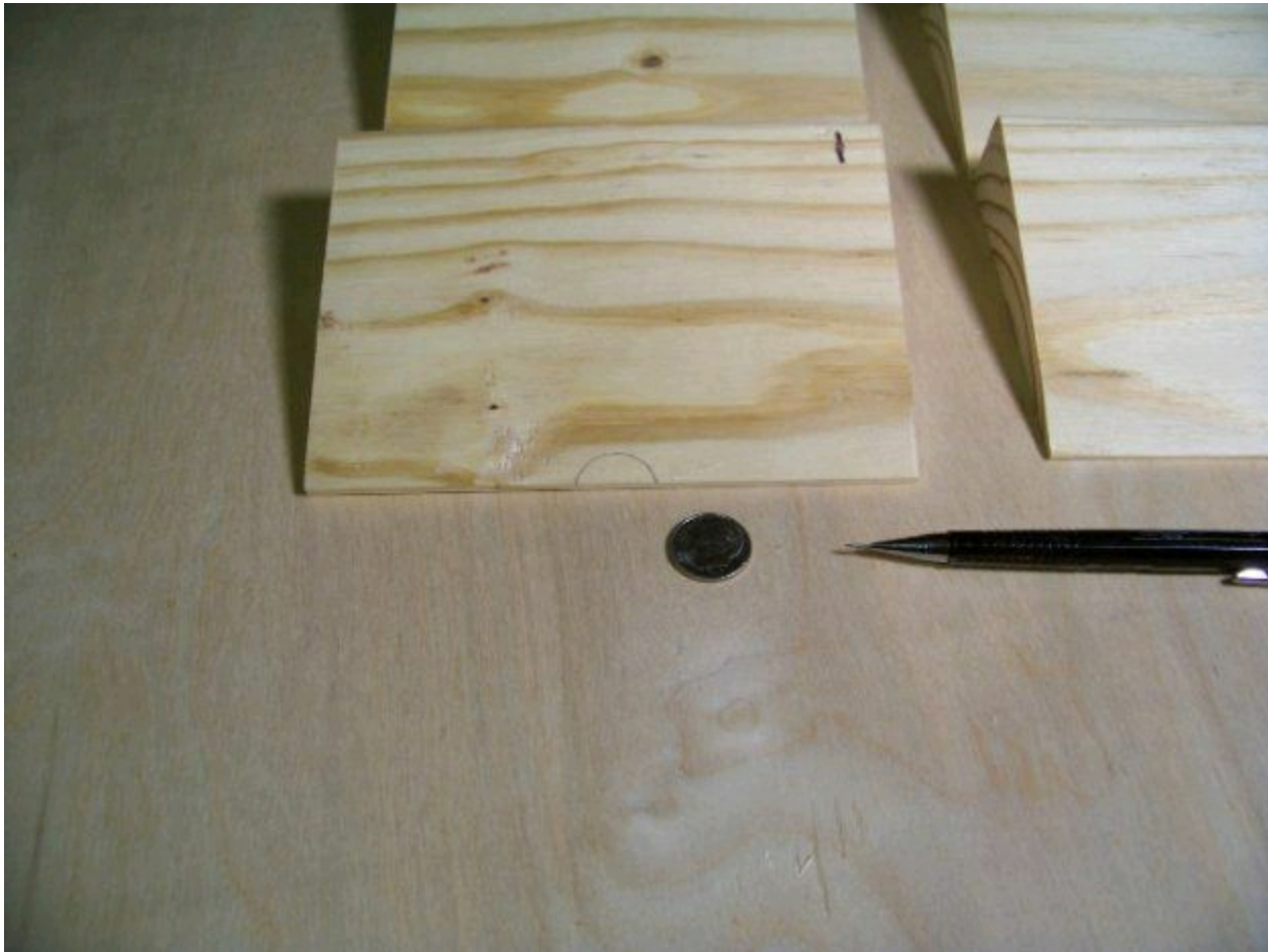
Figure 5 – A semi-circle is the pattern for the first segment cut. Subsequent segments will use the previous segment as a pattern.
