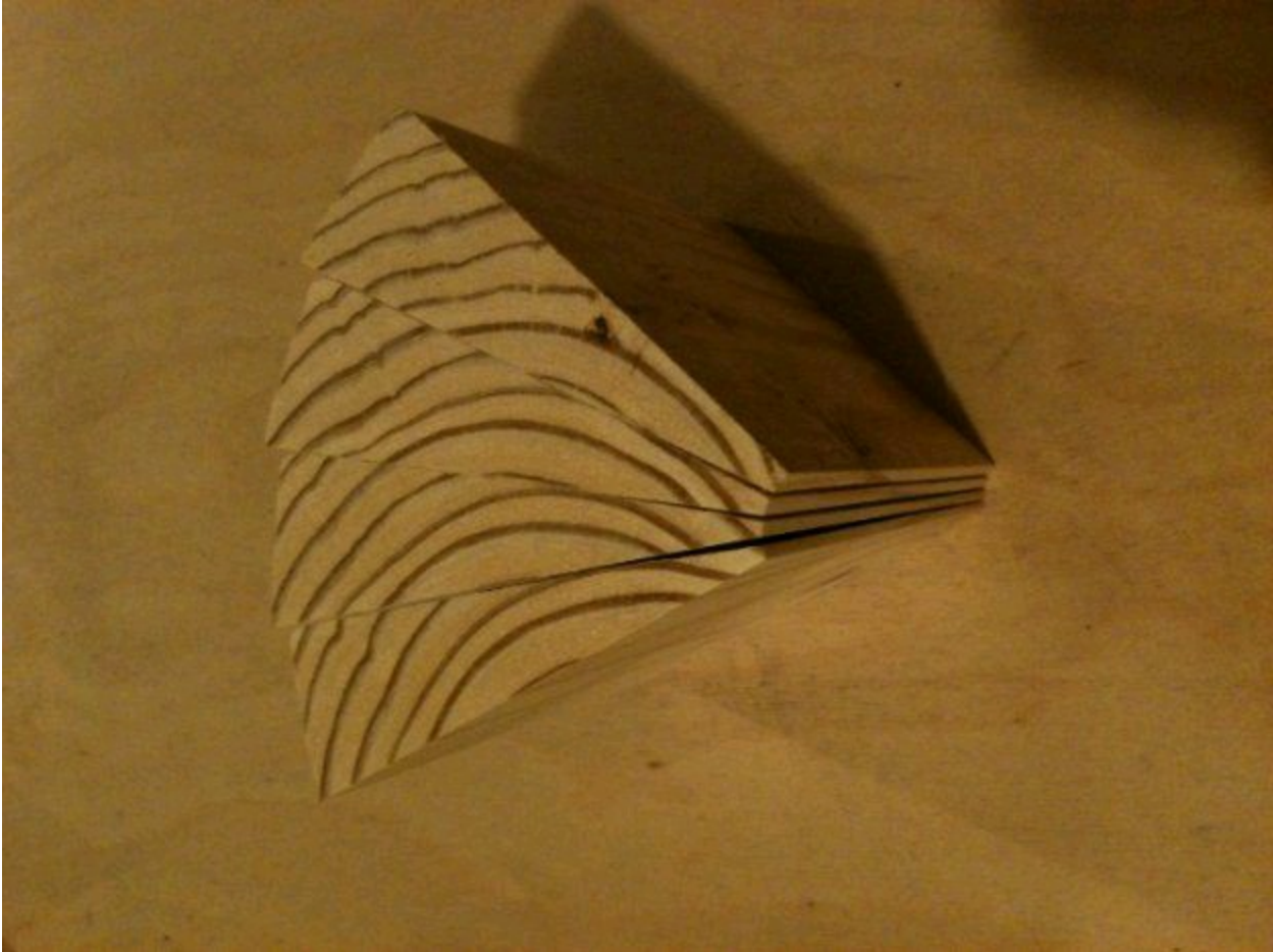
Figure 4 – The growth rings are oriented the same way. This set of wedges is ready to be numbered and used.
