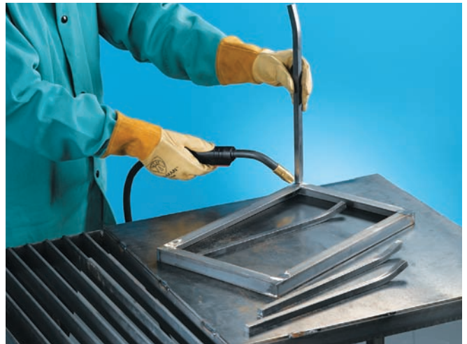
For a tiled tabletop, weld the legs to the flat underside—so that the flanges form a cradle for the tile and backing material.
