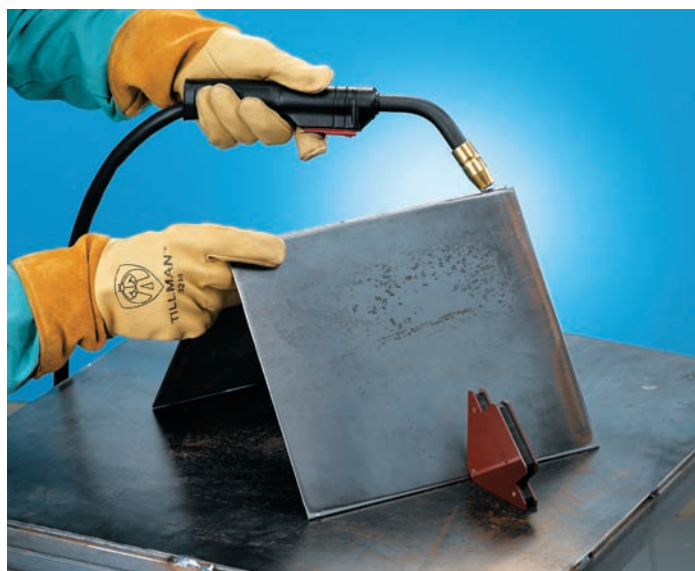
Form a V with rack sides and clamp with magnetic clamps. Weld the seam.
