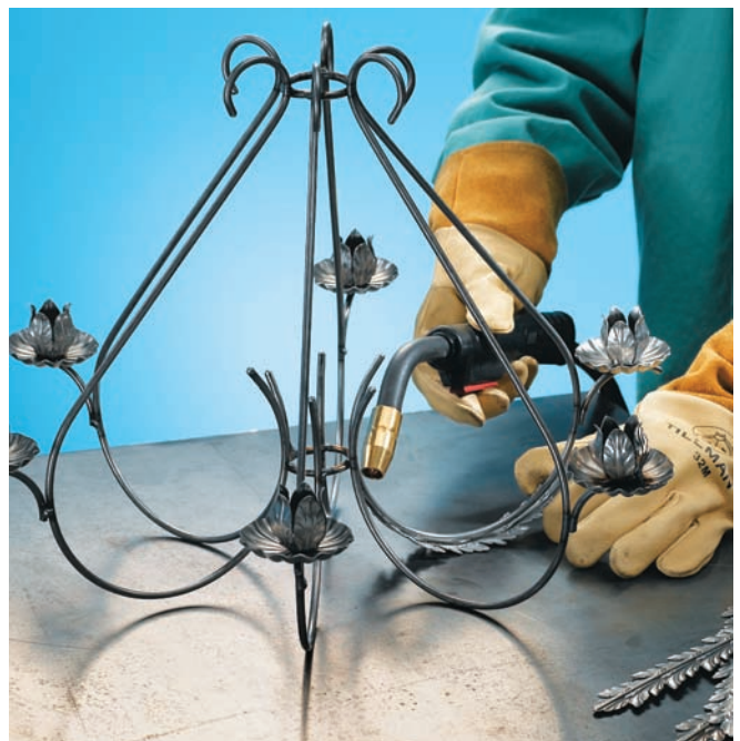
Bend the acanthus leaves to fit around the bottom curve of the scroll. Weld in place.
