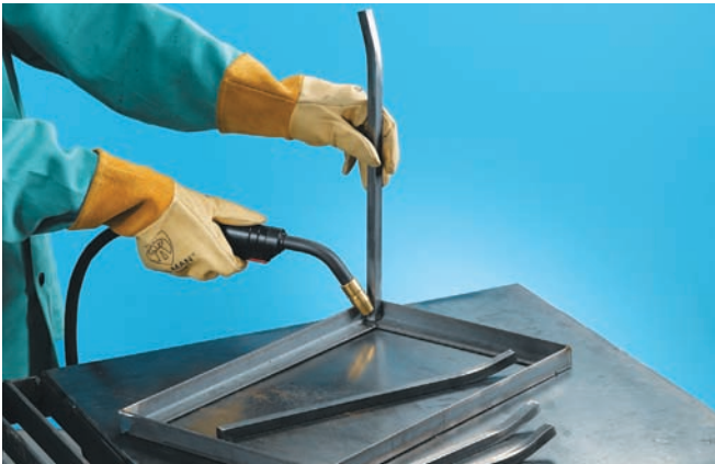
For a wood or metal tabletop, weld the legs inside the corner formed by the flanges. Align the curved legs so they point toward the long sides.
