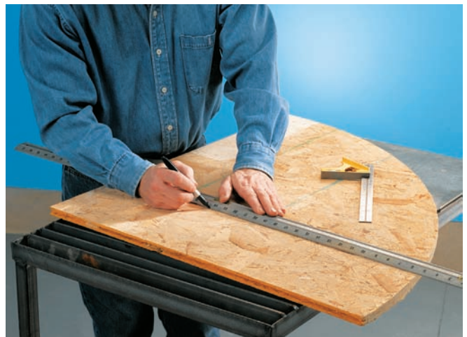
After bending the main arches, remove the quarter circles from the jig. Mark in 7½" from one flat edge and cut the form down.
