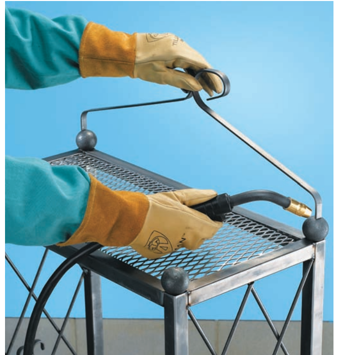
Weld the spheres to the tops of the legs and weld the scroll to the tops of the rear spheres.
