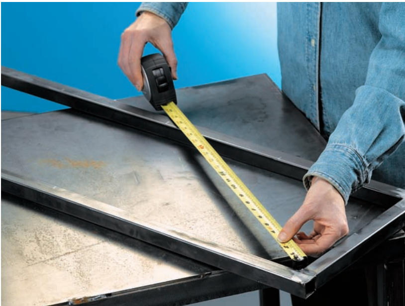
Measure between a corner and the opposite midpoint to find the length for the long diagonals.
