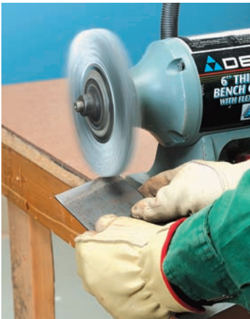
Cleaning the mill scale off mild steel is an important step. A bench-mounted power wire brush works well on small pieces. Wire brushing the entire project prior to finishing is critical for good paint adhesion.
