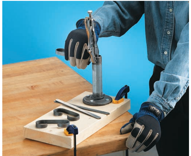
Bend the C-scrolls using a 1" pipe bending form.
