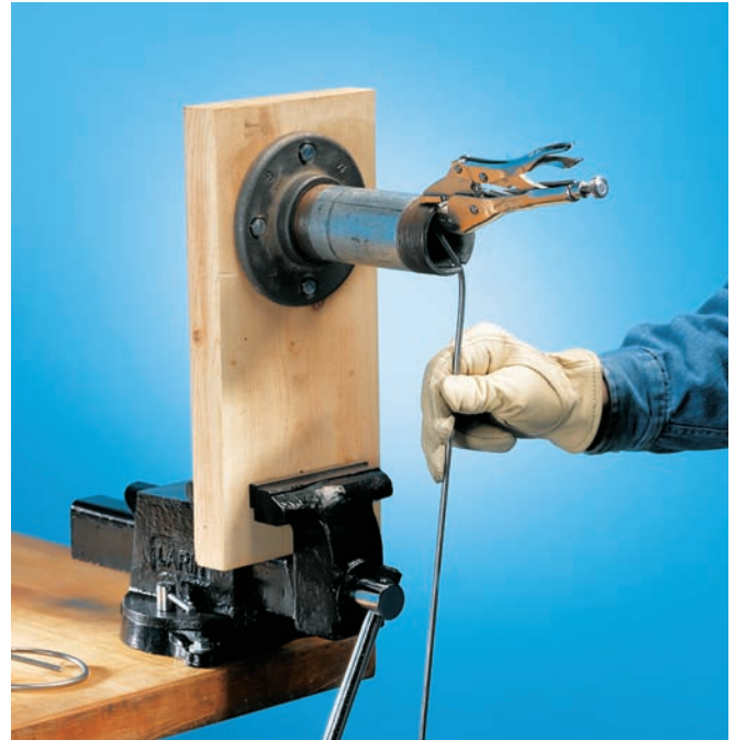
Cut a \frac{3}{16} " notch in a 2" pipe to create the bending jig for the scrolls. Slide the rod into the notch, then bend the rod around the pipe.
