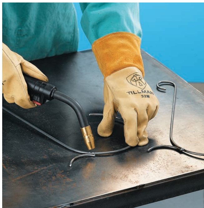
Weld the candle arms to the large end of the scrolls, even with the ring mark.
