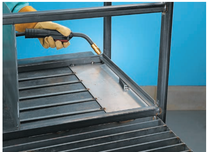
Weld the drawer glides to the legs.
