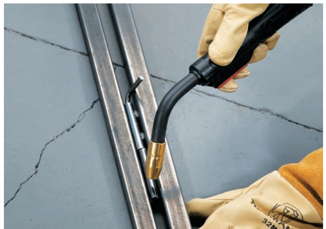
Insert a hinge pin into two hinge barrels. Place the hinge between two side panels and weld one barrel to one panel and the other barrel to the adjoining panel.
