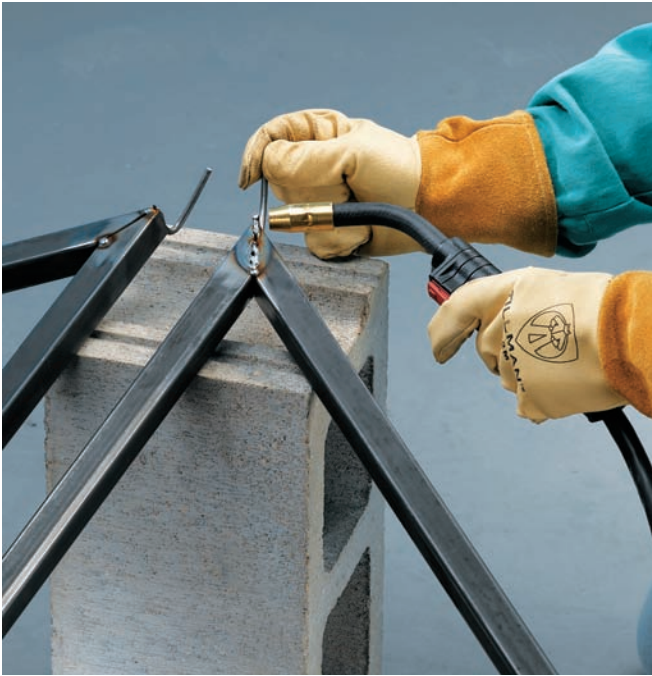
Support roof sections on a cinder block. Weld the finial pegs to the points of the panels.
