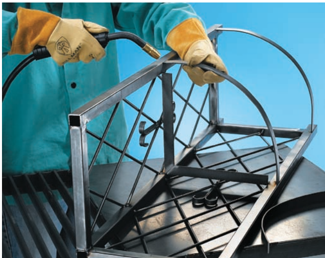
Weld the arched fronts to the sides, even with the crossbars.
