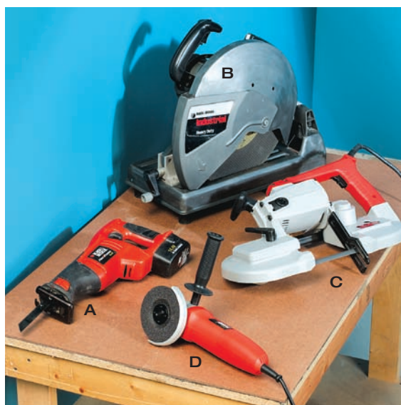
Power tools for a welding shop include: A. reciprocating saw, B. chop saw, C. portable band saw, D. angle grinder.
