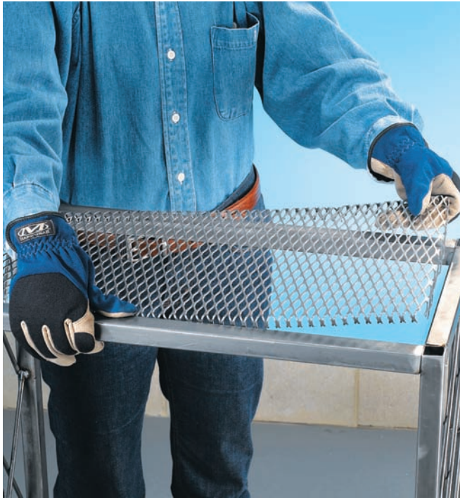
Bend the top shelf to fit inside the sides and supports.
