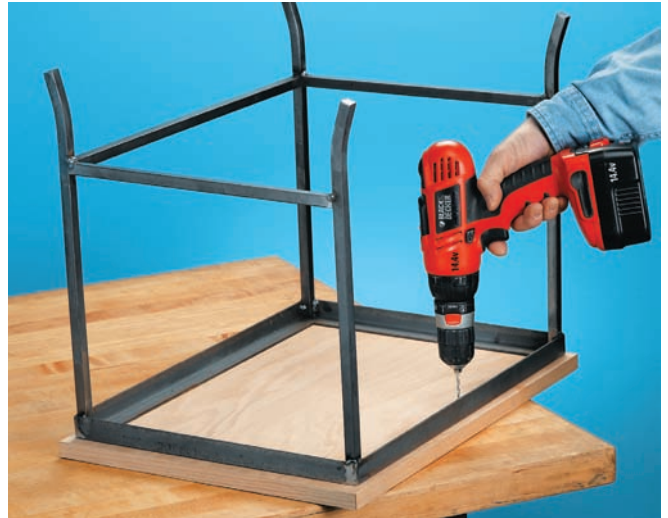
After drilling holes in each of the table's sides, align the wood top and drill pilot holes for the mounting screws.
