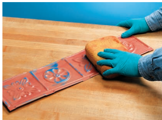
One method for creating an antique finish is to apply two wet top coats of different colors to a dry base coat of a third color. Before the top coats dry, wipe the top coats off in selected areas with a wet sponge.
