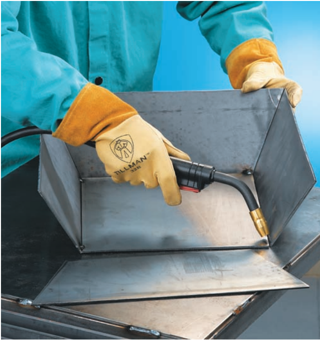
Tack-weld the sides to the base from the inside. Then turn the pit over and weld all the seams.
