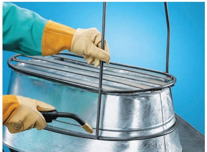
Tack-weld the legs in place, then remove the tub and finish the welds.
