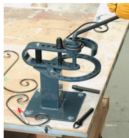
Use a scroll bender to bend decorative scrolls.
