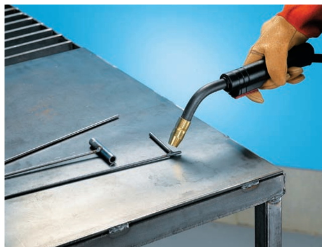
Weld the back leg to the hinge barrel, then weld the hinge pin to one front leg.
