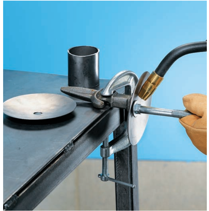
Create the finial assembly by welding the finial to the drip tray, then welding the bolt to the drip tray.
