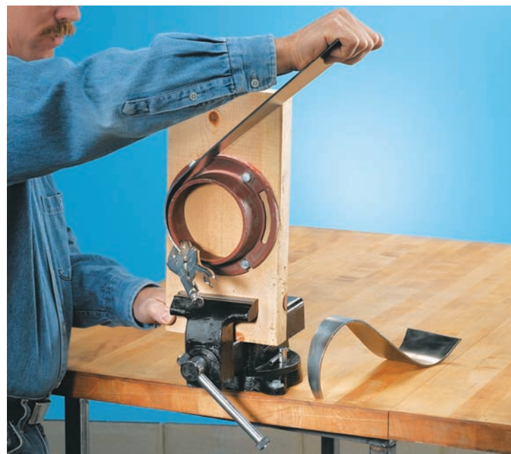
Clamp the narrow wave end to a 4" bending form and bend it slightly past halfway.
