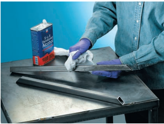
Use denatured alcohol to clean dirt and oil from project parts. Wear rubber gloves to protect your hands.
