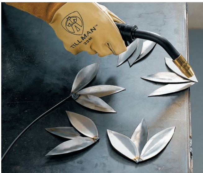
Arrange the leaves in sets of three. Weld the points together, then weld the stem to the leaf sets.
