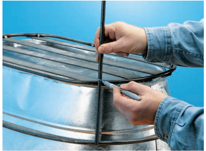
With the tub upside down, rest the tub support and base on the tub. Mark the leg blanks where they cross the base.
