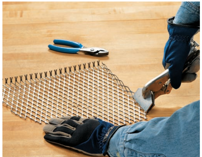
Use a hand seamer and pliers to bend the expanded sheet metal to fit inside the top and bottom crossbars.
