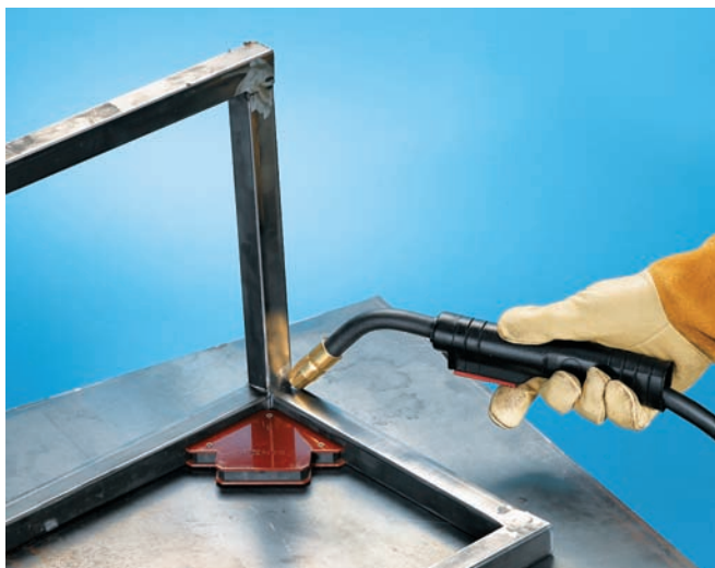
Attach the third leg and crosspieces to create a 90° angle.
