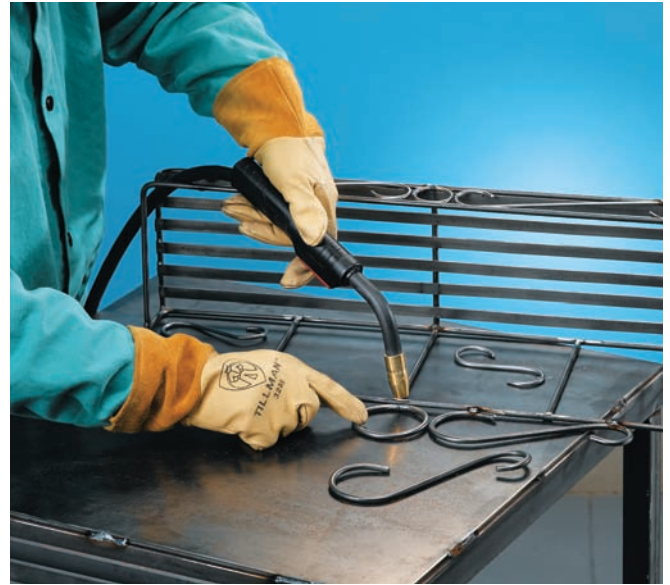
Weld the decorative scrolls and circles to the frames.
