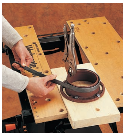
Use a vise-style pliers to hold the metal to the jig. Wrap the metal around the jig in a smooth motion.
