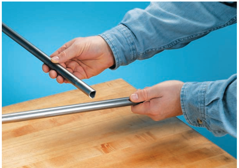
Grind a semicircle in the crossbar ends to create a saddle to fit around the legs.
