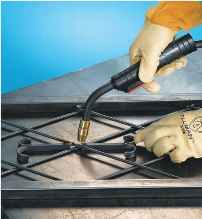
Weld the decorations to the middle X of the diagonals.
