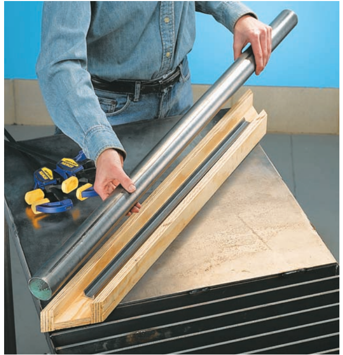
Creating a jig using a piece of channel iron and plywood makes cutting the 45° angles easier.
