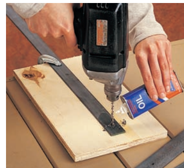
Drilling metal is fairly easy with a handheld drill or drill press.
