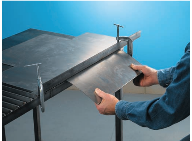
Cut the drawer to size. Clamp the drawer to a sharp-edged surface using C clamps and a piece of angle iron. Bend the sides, back and front of the drawer to 90°.
