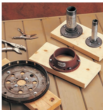
Bending jigs can be made from any rigid circular item. An engine flywheel, toilet flange, and various pipe sizes are shown here.
