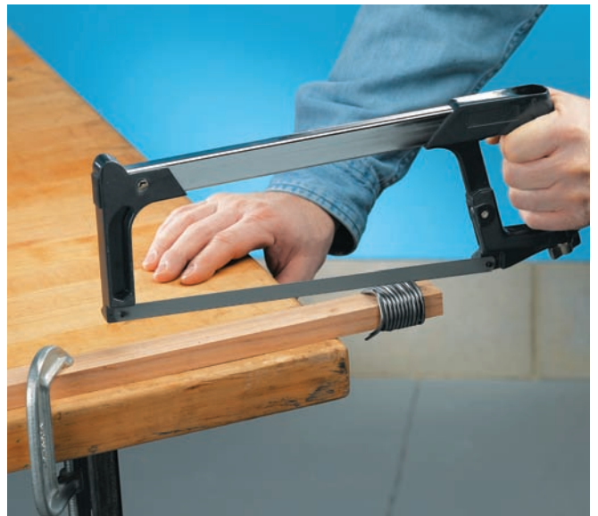
Wrap 1/8" round rod around a 1 x 1/2" hardwood stick. Clamp the stick to a stable surface and cut through the rod on the 1" side to make the individual chain links.
