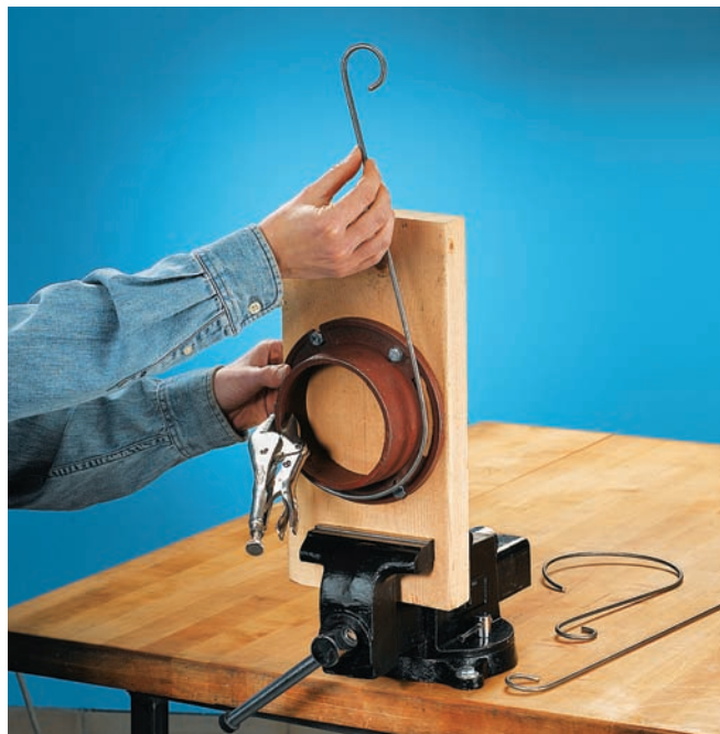
Make the second scroll bend around a 4" bending form.
