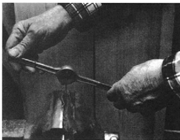
Figure 2-5. Thread drive shaft with a 6/32 die.
